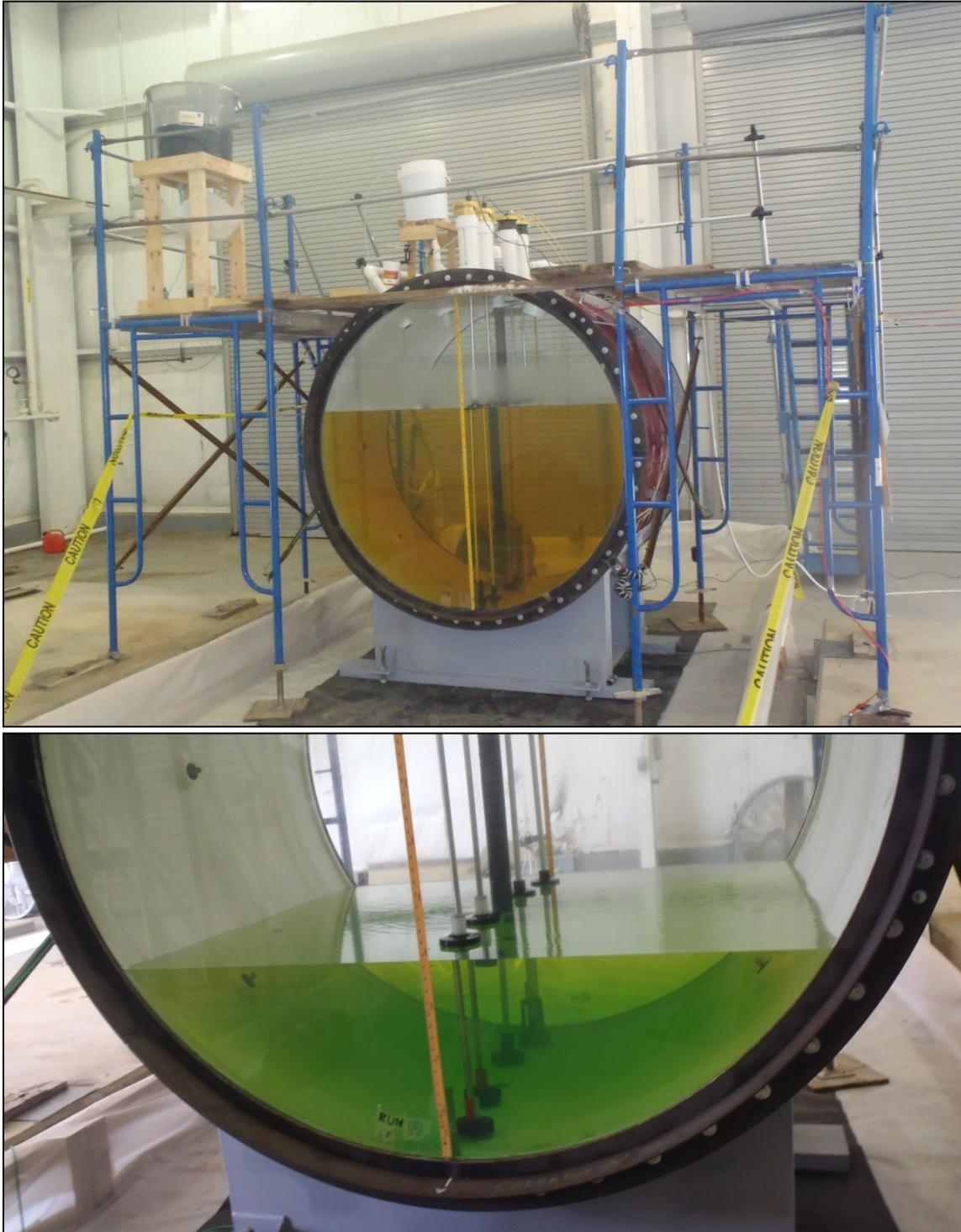
**Figure 3. Photographs of the test vessel at the Battelle West Jefferson facility. Top photo is an exterior view test vessel with scaffolding platform. The vessel is holding E0 at 65% full. Bottom photo shows the technologies during an E15 continuous water ingress run.**
