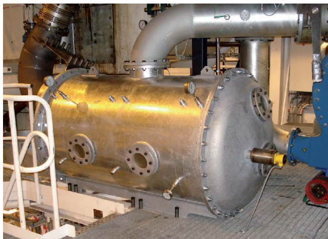
Figure 2-9. MAN Diesel EGR Scrubber
