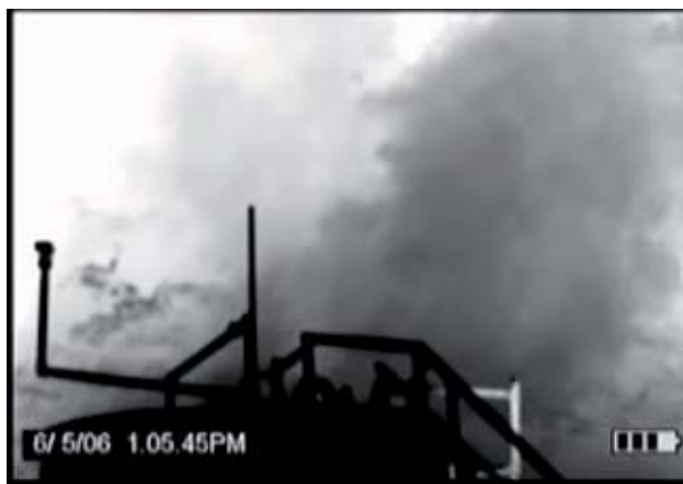
Figure 7: IR Image of Condensate Tank Volatile Organic Compound Emissions
