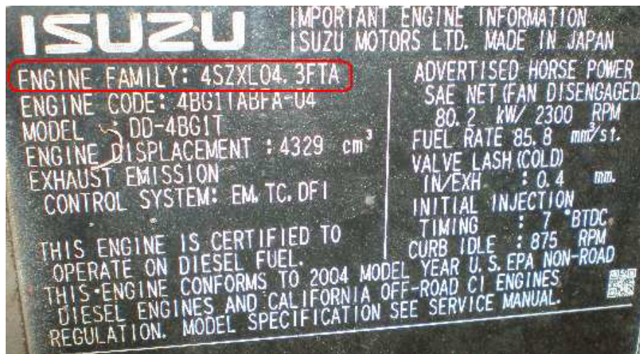
Figure 10. Engine Family Label for Off-road Diesel Equipment (Example 2)
