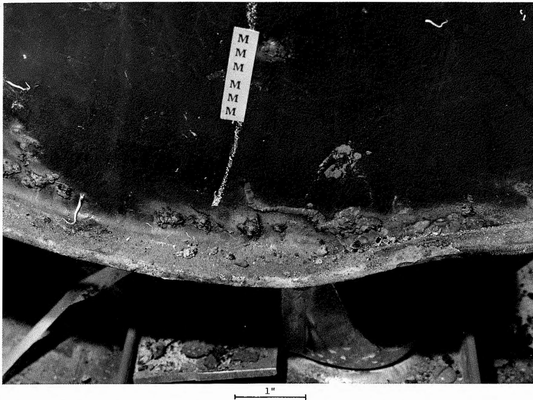
Figure 52. An Example of Filiform Corrosion.
