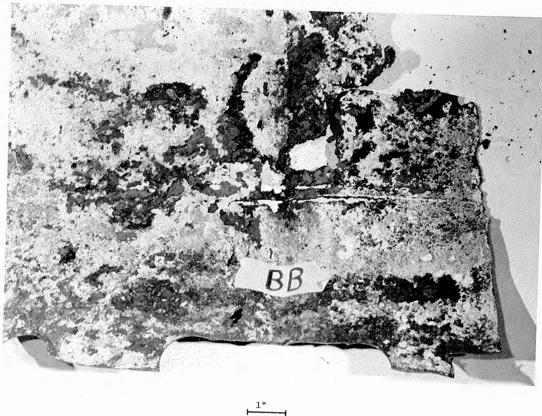
Figure 48. Attack Adjacent to the Weld in the Upper Container.
