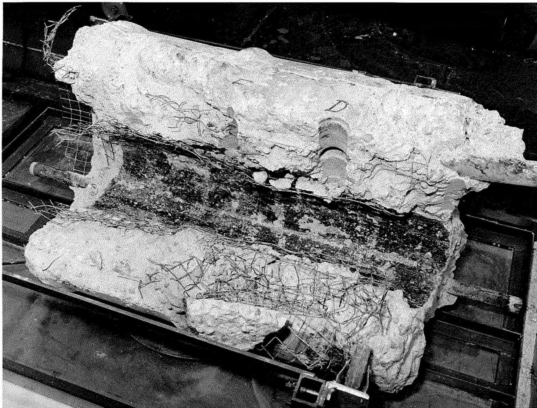
Figure 22. Concrete Waste Form after Removal of the Inner Container.
