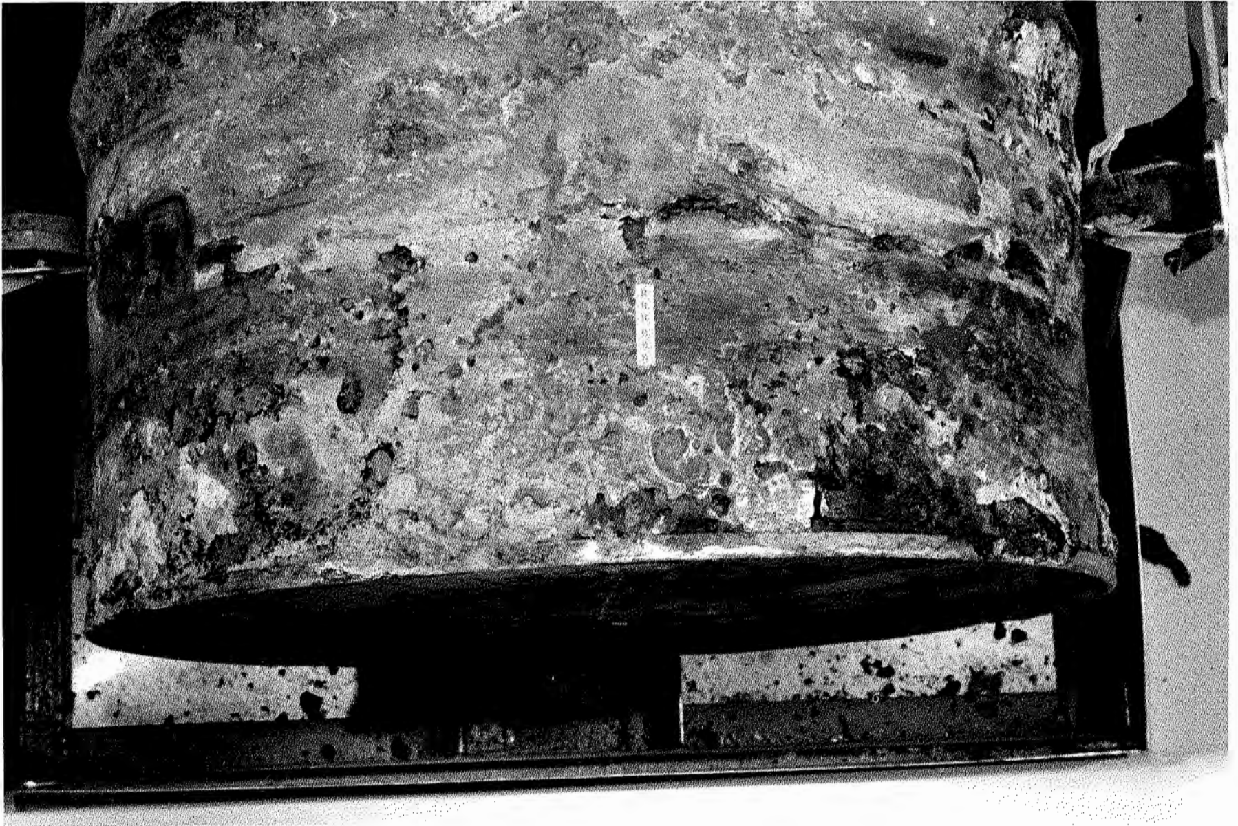
Figure 50. Macroscopic Pits Covering the Carbon S End of the Container.
