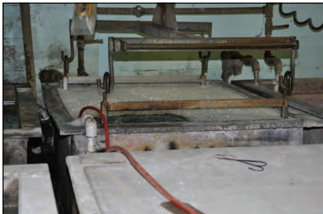
Inside Maracle Industrial Finishing showing the process lines and rinse tanks
