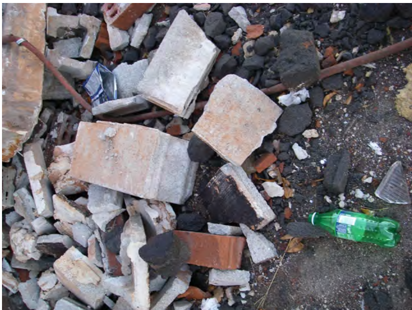
Closeup of asbestos containing material (ACM) applied to cinderblocks that had been demolished at Haynsworth Mill.
