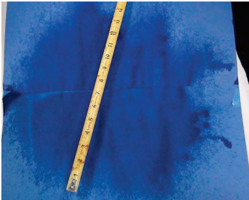
**Figure 1. Spray Pattern from Nozzle 1 Foot Away**
