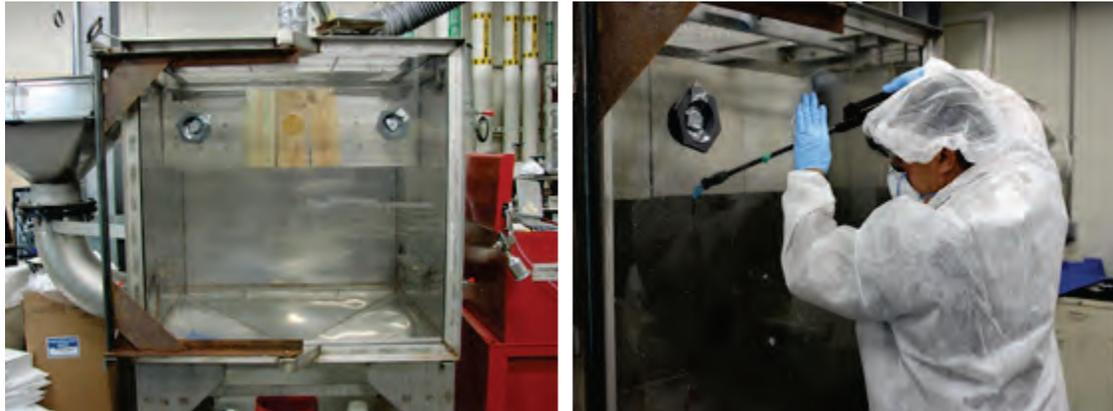
**Figure 2-2. Decontamination Chamber for AHP-Based Decontamination Testing (Left) and Application of AHP Using Backpack Sprayer (Right)**
