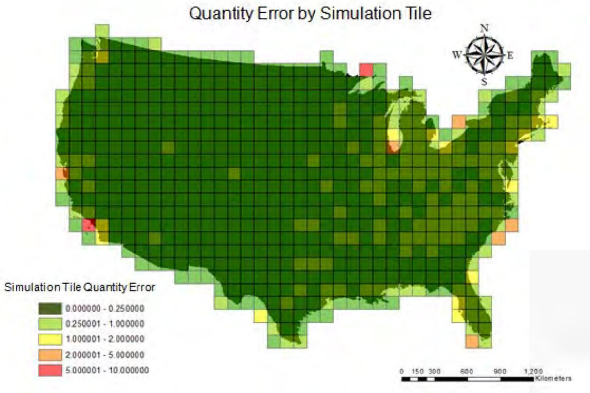
**Figure 5-2. Goodness of fit statistics of quantity-change results of the model when applied to the entire lower 48 states. As measure for goodness of fit the correctness, on a scale of 0 to 1, of 3 x 3 km simulation tiles relative to observed values was used**
