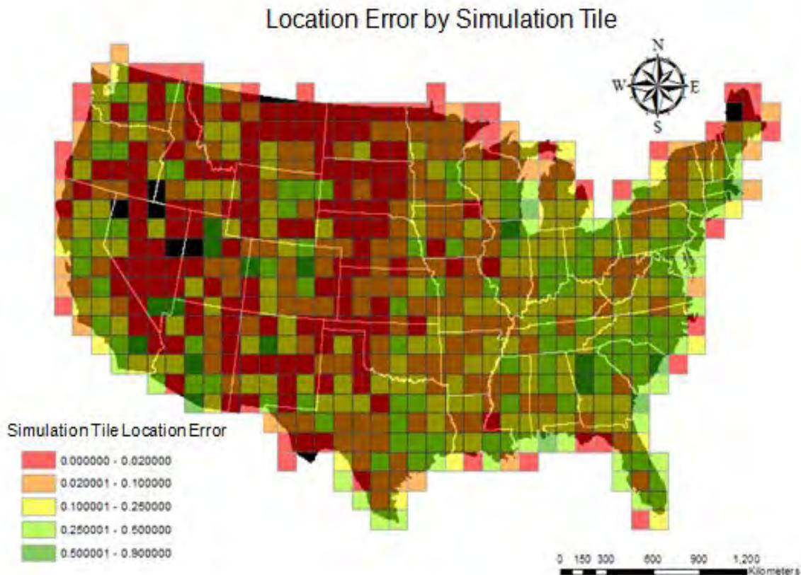
**Figure 5-1. Goodness-of-fit statistics of location-change results of the model when applied to the entire 48 states. As measure for goodness of fit the correctness, on a scale of 0 to 1, of 3 x 3 km simulation tiles relative to observed values was used**
