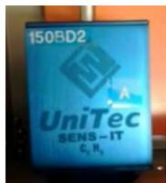
The UniTec Sens-It is a small gas-sensing device that can measure volatile organic compounds (VOCs). This sensor is used to measure VOCs in applications such as urban air quality, roadside pollution, and (solid waste) landfill monitoring. This operating procedure explains what you need to do to collect high-quality VOC data using the Sens-It for your monitoring project.
