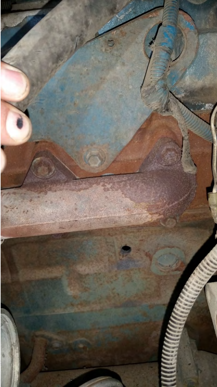
6) Engine block, after hole has been drilled
