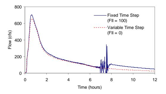
Figure 8-1 Flow Instability Index for a flow hydrograph
