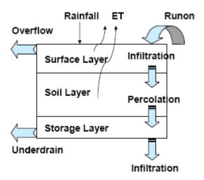
Figure 3-9 Conceptual diagram of a bio-retention cell LID
