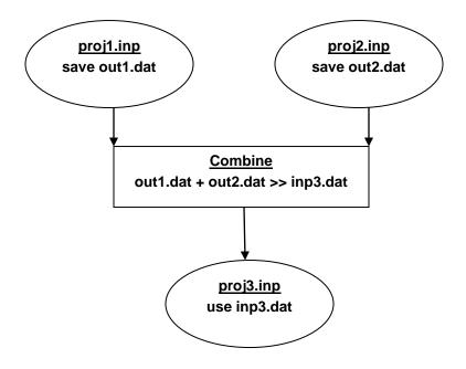
Figure 11-1 Combining routing interface files
