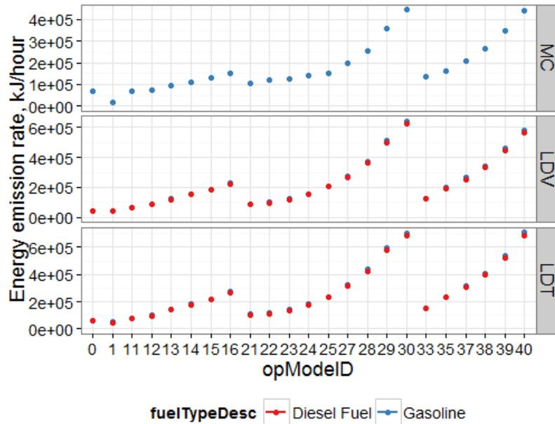
**Figure 2-2. Average energy consumption rates for motorcycle, light-duty vehicles, and light-duty trucks across all running operating modes. 1960-1969 MY have the same energy consumption rates as MY 1970, and the MY 2031-2050 have the same energy rates as MY 2030**
