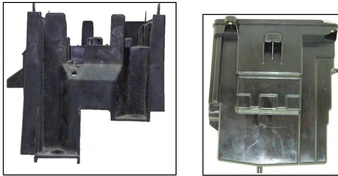
Image 3.18-28: Fuse Box (Support) for the Silverado 1500 and 2500 (Left) and Renault Master 2.3 DCi (Right)
