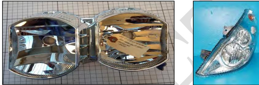
Image 3.17–9: Headlamp inner reflector for the Silverado 1500 (Left) and Renault Master 2.3 DCi (Right)
