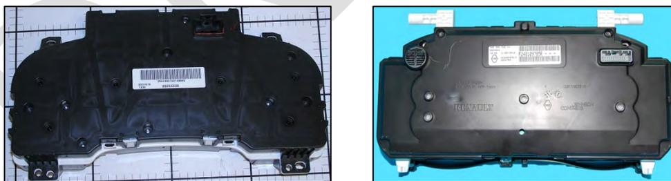
*Image 3.15–16: Cluster Rear Housing for the Silverado 1500 and 2500 (Left) and Renault Master 2.3 DCi (Right)*
