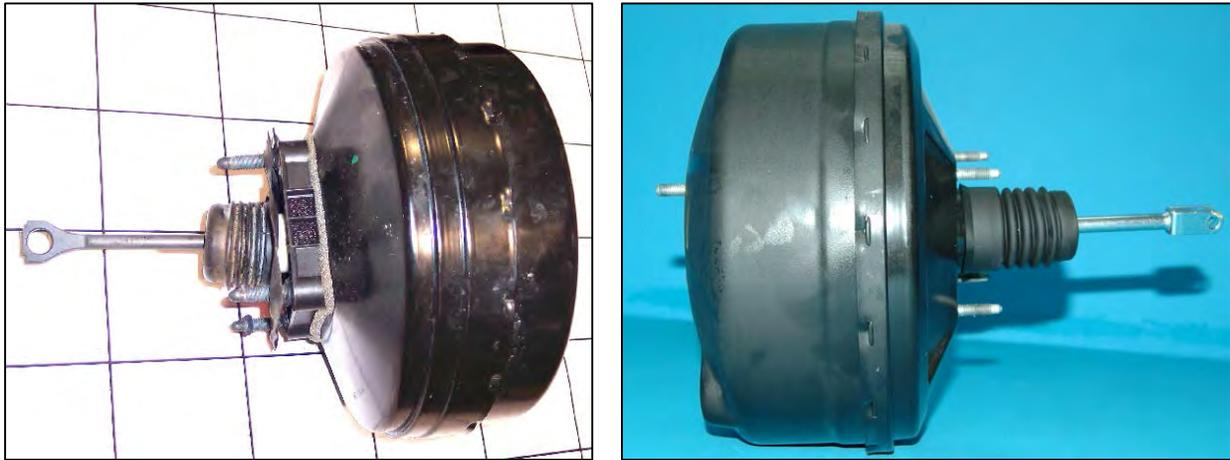
*Image 3.9-21: Vacuum Booster for the Silverado 1500 (Left) and Mercedes Sprinter 311 CDi (Right)*
