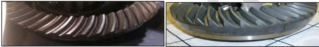
*Image 3.8–12: Front Carrier Ring Gear for the Silverado 1500 (Right) and Silverado 2500 (Left)*
