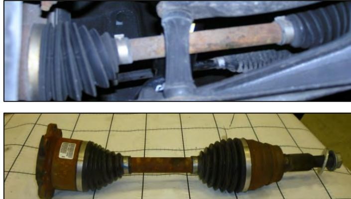
Image 3.8–9: Front Differential Output Shaft with Hub for the Silverado 1500 (Top) and Silverado 2500 (Bottom)
