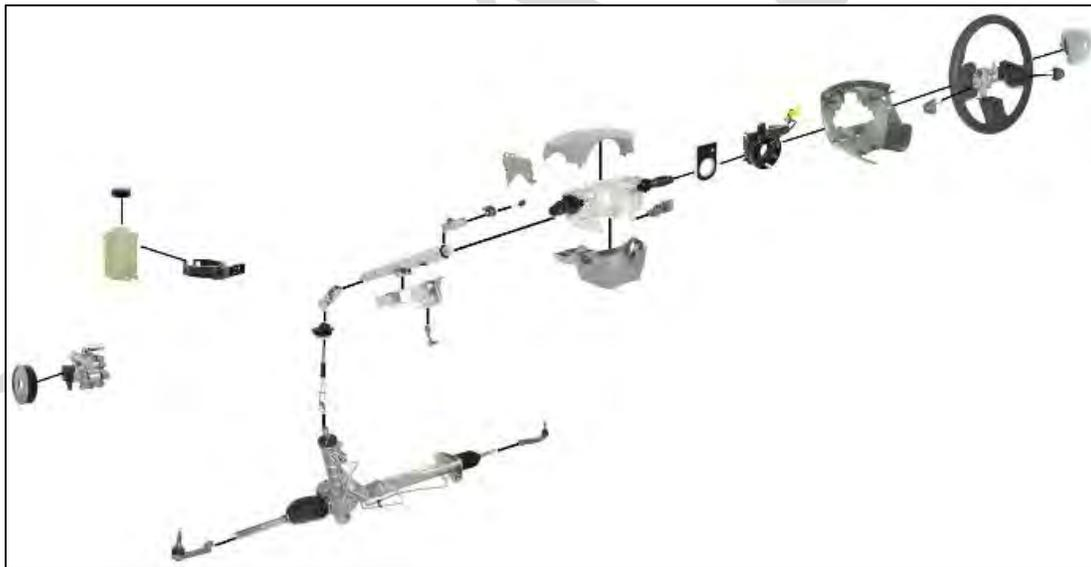
Image 3.13–11: Renault Master 2.3 DCi Steering Components
