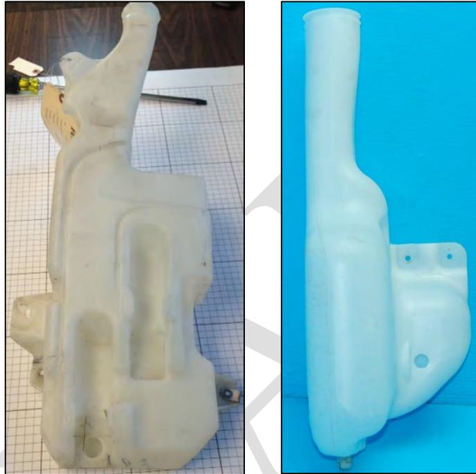
*Image 3.6–7: Washer Tank for the Silverado 1500 (Left) and Mercedes Sprinter 311 CDI (Right)*
