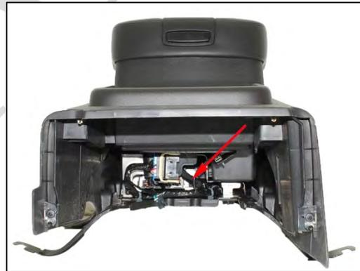
*Image 3.18–17: Center console wiring for the Silverado 1500 and 2500*
