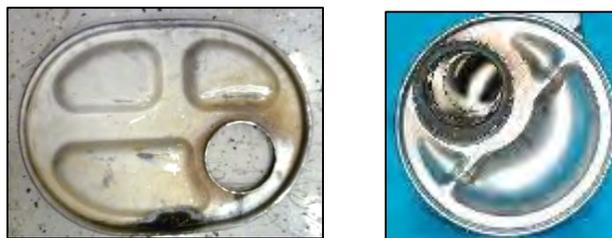
*Image 3.11–19: Muffler end plates for the Silverado 1500 (Left) and Renault Master 2.3 DCi (Right)*
