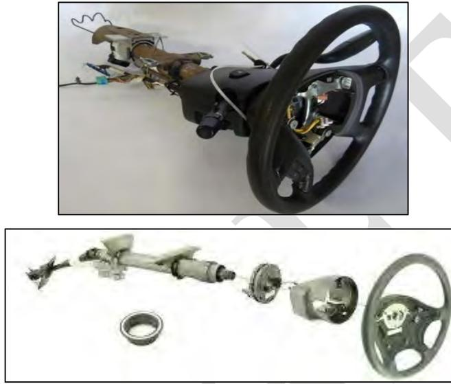
*Image 3.13–9: Steering Column for the Silverado 1500 (Top) and Sprinter 311 (Bottom)*
