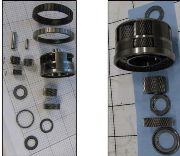
*Image 3.2-3: Planet gears for the Silverado 1500 (Left) and Silverado 2500 (Right)
