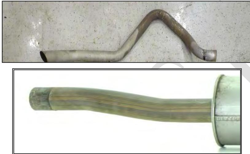
*Image 3.11–14: Muffler pipes for the Silverado 1500 (Top) and Mercedes Sprinter (Bottom)*
