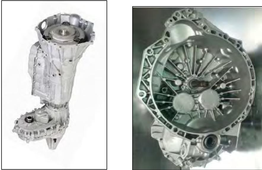
Image 3.2-12: Transmission for the Silverado 1500 (Left) and Renault Master 2.3 (Right)
