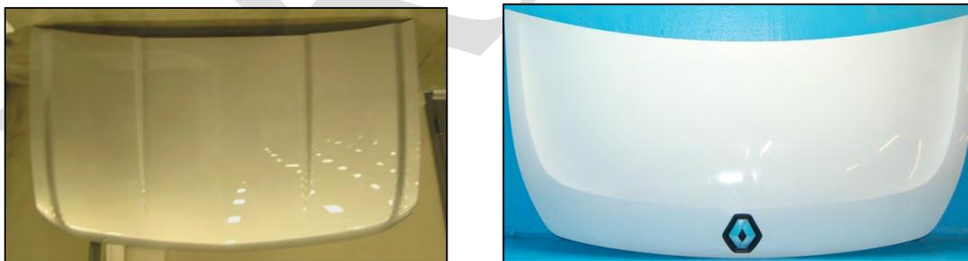
*Image 3.3–27: Hood assembly without hinges for the Silverado 1500 (Left) and Renault Master 2.3 DCi (Right)*
