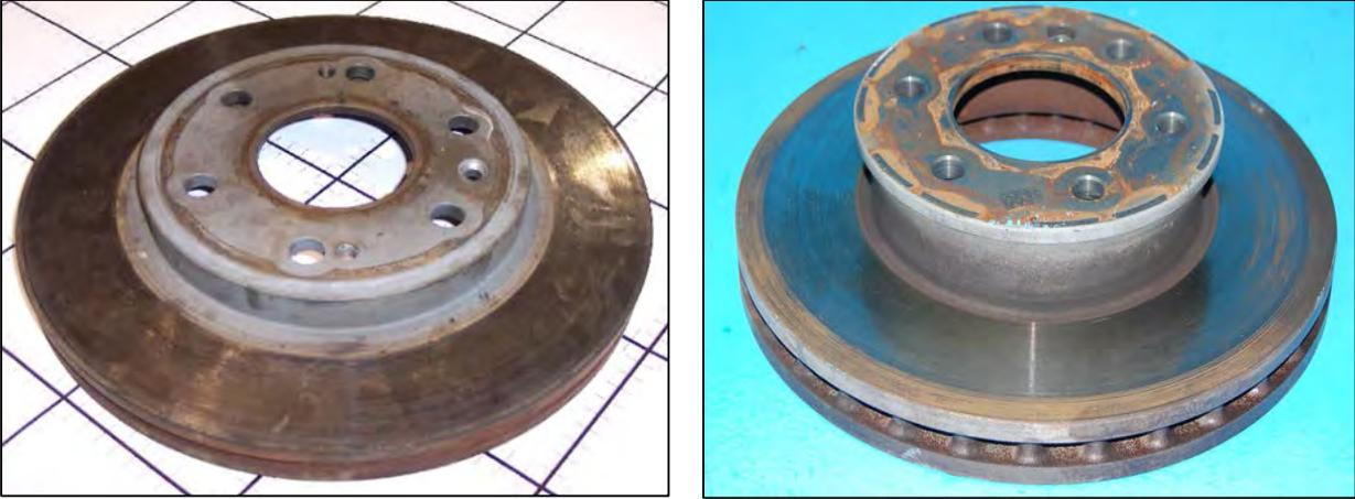
*Image 3.9–13: Front Rotor; 1500 Series (Left), Sprinter Series (Right)*
