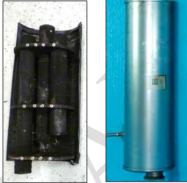
*Image 3.11–18: Muffler skin for the Silverado 1500 (Left) and Renault Master 2.3 DCi (Right)*
