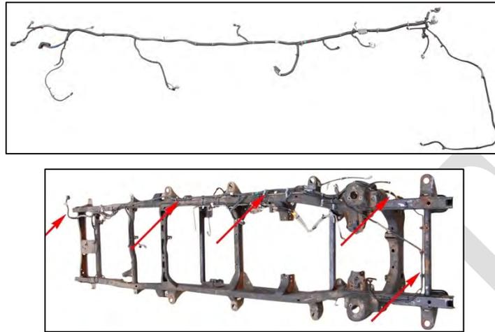
*Image 3.18–11: Under frame/tow harness (wiring on understructure) for the Silverado 1500 and 2500
