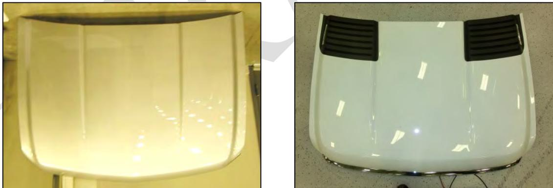
*Image 3.3–10: Hood assembly without hinges, Silverado 1500 (Left) and Silverado 2500 (Right)*
