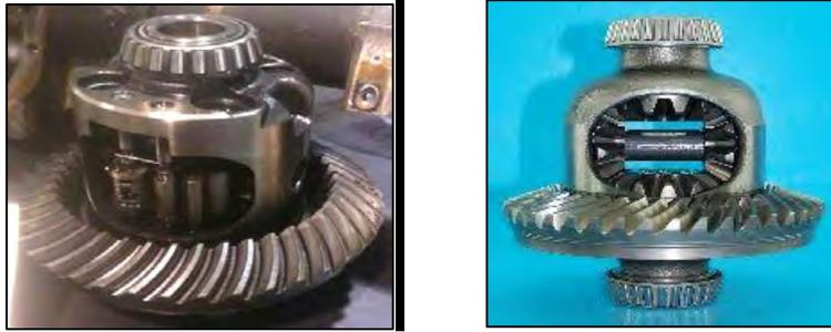
Image 3.8–27: Rear Carrier Casting for the Silverado 1500 (Left) and Renault Master 2.3 DCi (Right)
