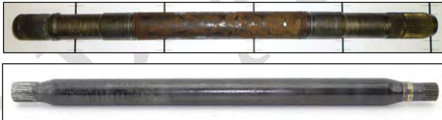
*Image 3.8–18: Rear Axle Shaft for the Silverado 1500 (Top) and Mercedes Sprinter 311 CDI (Bottom)*
