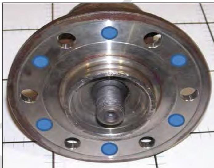
*Image 3.8–15: Front Half Shaft Hub with locations for drilling lightening holes*
