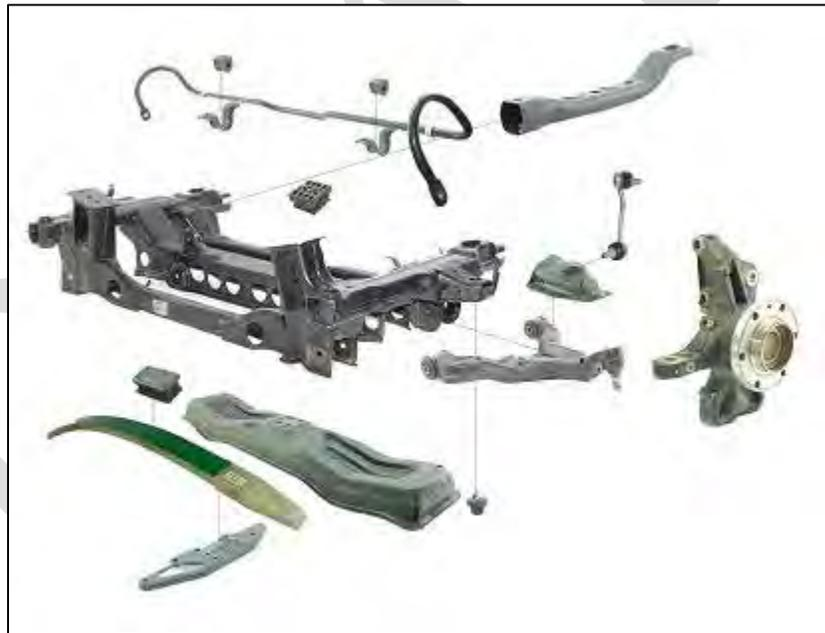
Image 3.7–13: Mercedes Sprinter Front Suspension System
