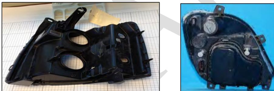
*Image 3.17-5: Headlamp housing for the Silverado 1500 (Left) and Mercedes Sprinter 311 CDi (Right)
