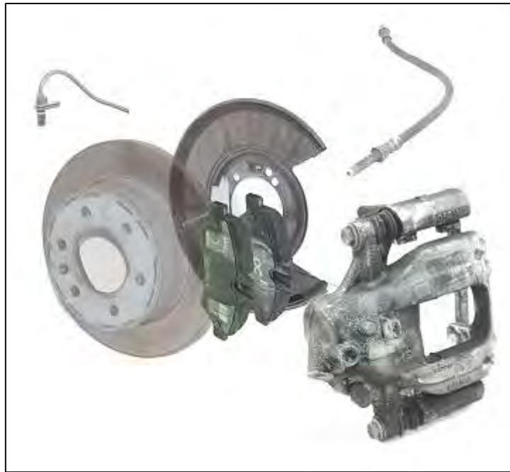
*Image 3.9-12: Mercedes Sprinter Rear Rotor/Drum and Shield Subsystem*
