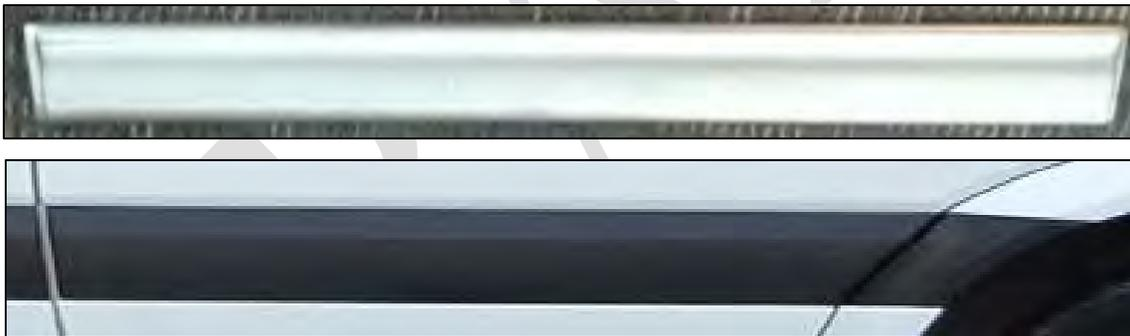
Image 3.5–14: Bumper Guard (Front Door) for the Silverado 1500 (Top) and Mercedes Sprinter 311 CDI (Bottom)
