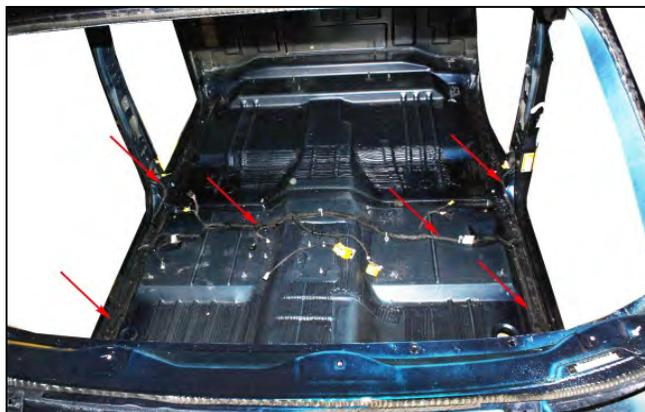
Image 3.18-9: Body and Rear End Wiring (Complete) for the Silverado 1500 and 2500
