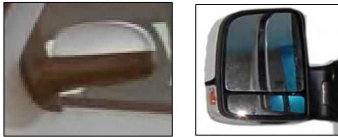
*Image 3.5–15: Exterior Mirror (Driver Side shown; Passenger Side similar) for the Silverado 1500 (Left) and Mercedes Sprinter 311 CDi (Right)*
