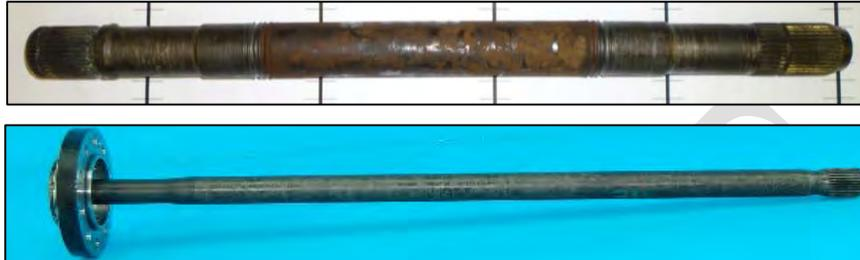
*Image 3.8–25: Rear Axle Shaft for the Silverado 1500 (Top) and Renault Master 2.3 DCi (Bottom)*
