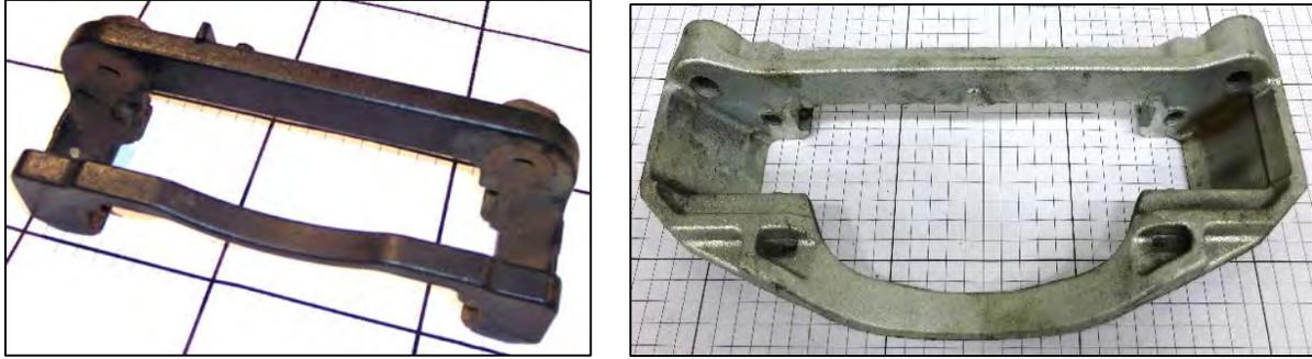
*Image 3.9-5: Front Caliper Mounting Bracket; 1500 Series (Left), 2500 Series (Right)*
