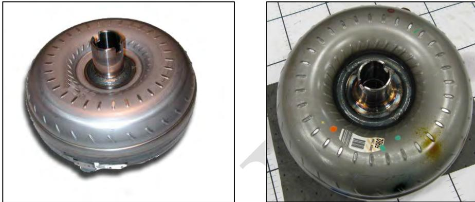
*Image 3.2–5: Steel torque converter for the Silverado 1500 (Left) and Silverado 2500 (Right)*
