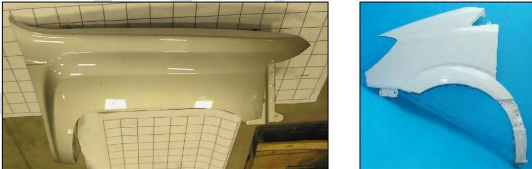
*Image 3.3–19: RH/LH front fenders for the Silverado 1500 (Left) and Mercedes Sprinter 311 CDi (Right)*
