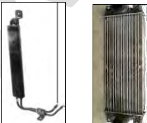
Image 3.13–15: Heat Exchangers for the Silverado 1500 (Left) and Renault Master 2.3 (Right)
