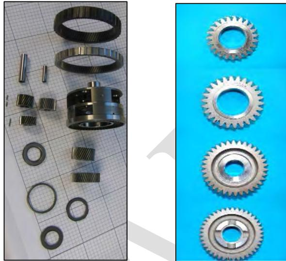
*Image 3.2–10: Planet gears for the Silverado 1500 (Left) and drive gears for the Sprinter 311 (Right)*
