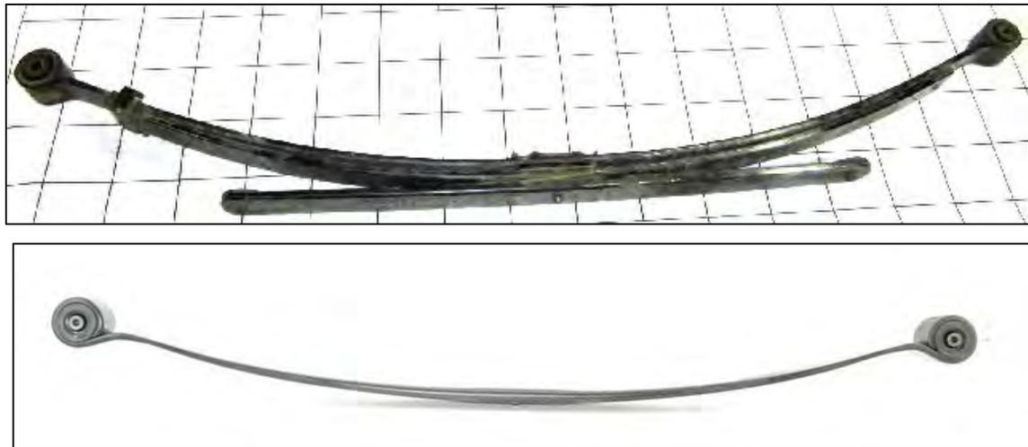
*Image 3.7-22: Leaf Spring Assembly for the Silverado 1500 (Top) and Sprinter (Bottom)*
