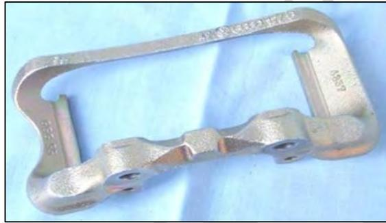
*Image 3.9-6: Front Caliper Mounting Bracket Mass Reduced Component Example*
