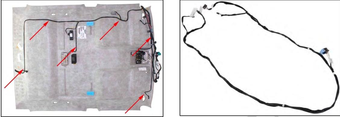
*Image 3.18–30: Headliner wiring for the Silverado 1500 and 2500 (Left) and the Renault Master 2.3 DCi (Right)
