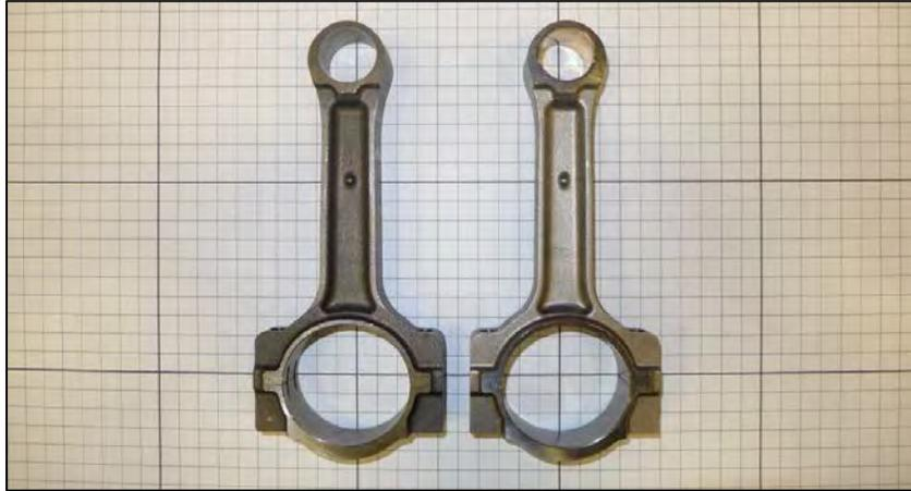
Image 3.1–3: Connecting rod for 5.3 liter LC9 (Left) and 6.0 liter LC8 (Right)
