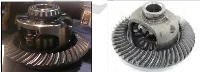
*Image 3.8–20: Rear Carrier Casting for the Silverado 1500 (Left) and Mercedes Sprinter 311 CDi (Right)*
