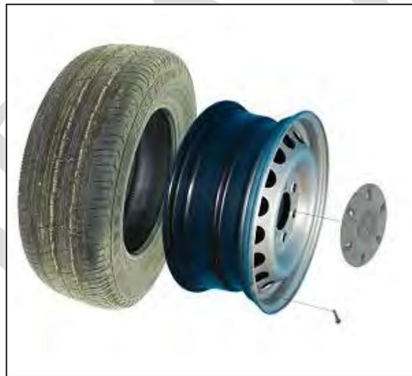
*Image 3.7-15: Mercedes Sprinter Road Wheel Assembly*
