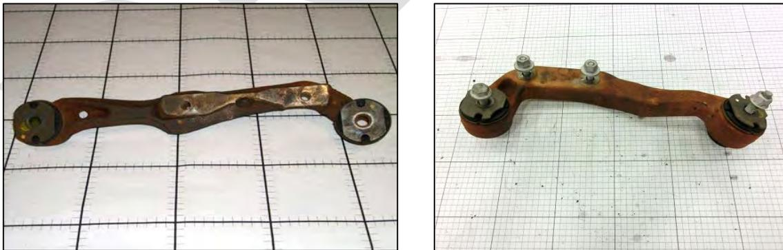
*Image 3.8–13: Front Differential Mounting Bracket RH for the Silverado 1500 (Right) and Silverado 2500 (Left)*
