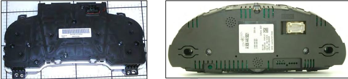
*Image 3.15–10: Cluster Rear Housing for the Silverado 1500 and 2500 (Left) and Mercedes Sprinter 311 CDi (Right)*
