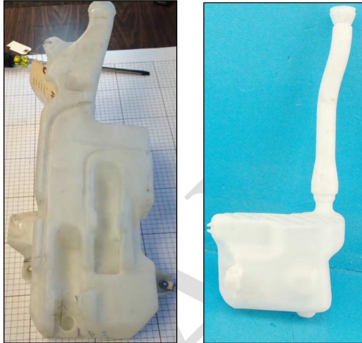
*Image 3.6–9: Washer Tank for the Silverado 1500 (Left) and Renault Master 2.3 DCi (Right)*
