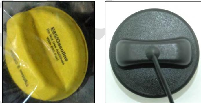
*Image 3.12–14: Fuel Cap for the Silverado 1500 (Left) and Mercedes Sprinter 311 CDi (Right)*
