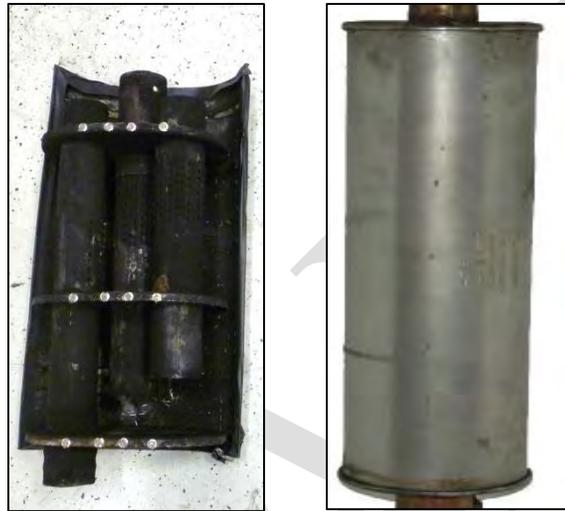
*Image 3.11–12: Muffler skin for the Silverado 1500 (Left) and Mercedes Sprinter (Right)*
