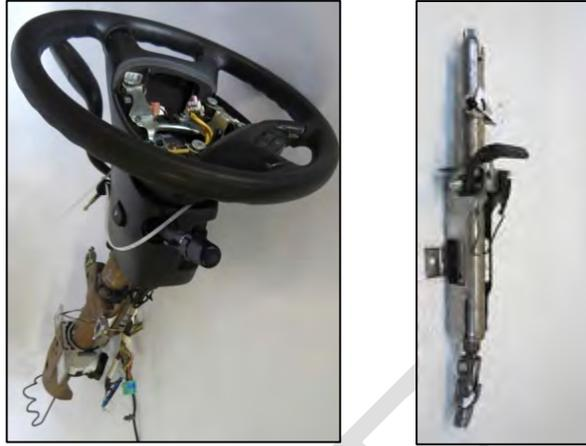
*Image 3.13–16: Steering Column for the Silverado 1500 (Left) Renault Master 2.3 (Right)*
