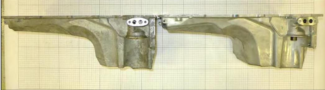
*Image 3.1–10: Oil pan for 5.3 liter LC9 (Left) and 6.0 liter LC8 (Right)*
