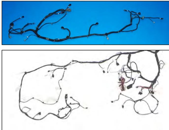
*Image 3.18–22: Front Bumper Harness (Wiring on front module) for the Silverado 1500 and 2500 (Top) and Mercedes Sprinter 311 CDI (Bottom)*
