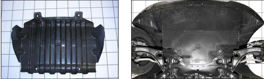
*Image 3.3–24: Front splash shield for the Silverado 1500 (Left) and the Renault Master 2.3 DCi (Right)*
