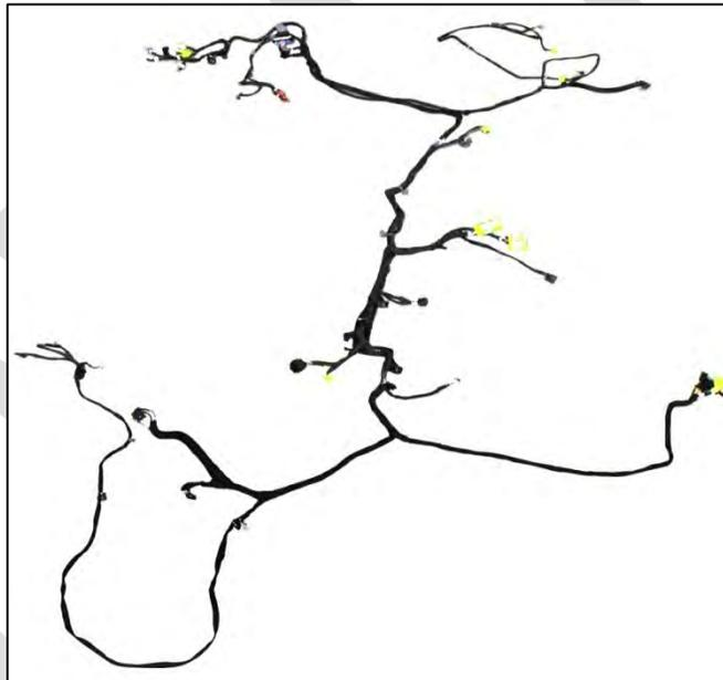
*Image 3.18-8: Body and Rear End Wiring (Complete) for the Silverado 1500 and 2500*
