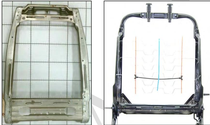
*Image 3.4–14: Seating Subsystem for the Silverado 1500 (Left) and Renault Master 2.3 DCi (Right)*
