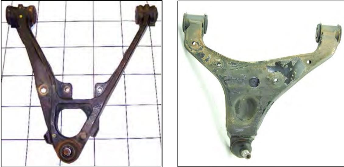
*Image 3.7–18: Lower Control Arm for the Silverado 1500 (Left) and Mercedes Sprinter (Right)*
