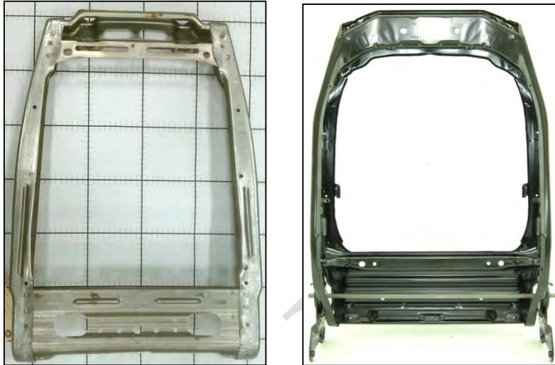
*Image 3.4–9: Seating Subsystems for the Silverado 1500 (Left) and Mercedes Sprinter 311 CDi (Right)*
