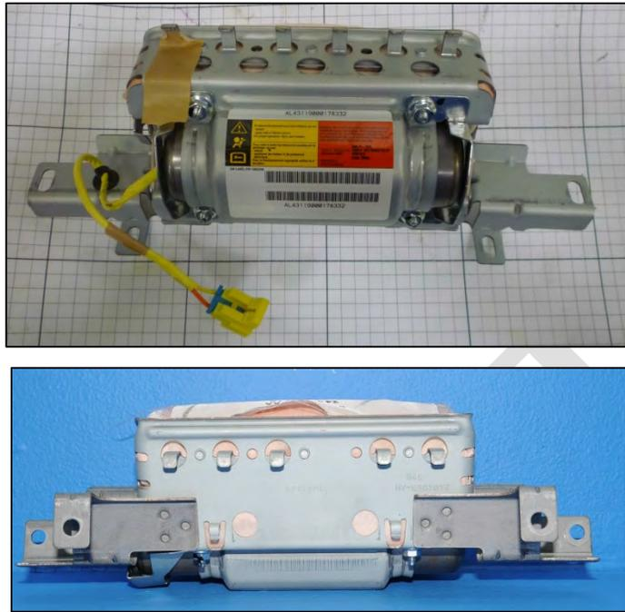
*Image 3.4-11: Occupant Restraining Device Subsystem for the Silverado 1500 (Top) and Mercedes Sprinter 311 CDi (Bottom)*
