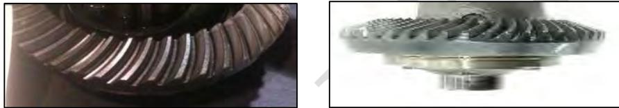
*Image 3.8–22: Rear Carrier Ring Gear for the Silverado 1500 (Left) and Mercedes Sprinter 311 CDi (Right)*
