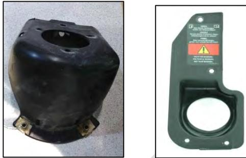
*Image 3.12–13: Fuel Filler Cap Housing for the Silverado 1500 (Left) and Mercedes Sprinter 311 CDi (Right)*
