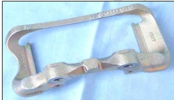
*Image 3.9-18: Front Caliper Mounting Bracket Mass Reduced Component Example*
