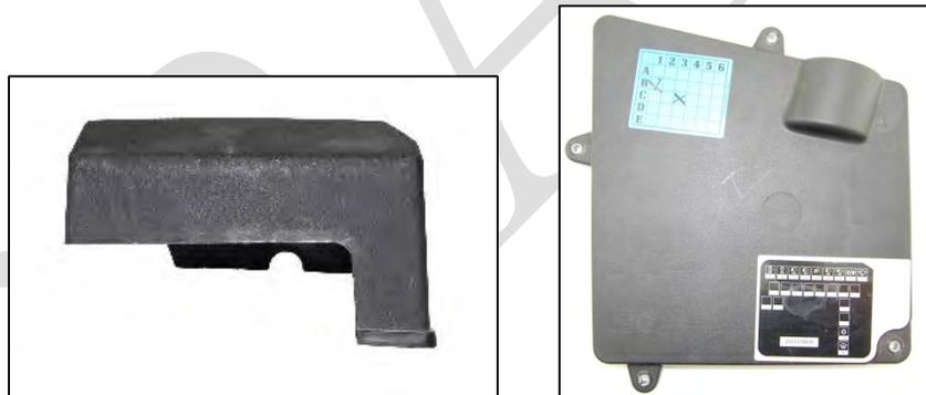
Image 3.18-29: Fuse Box Cover for the Silverado 1500 and 2500 (Left) and Renault Master 2.3 DCi (Right)
