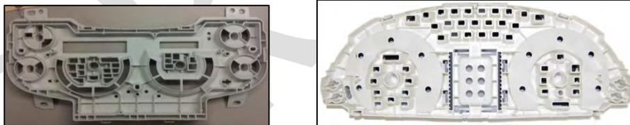
*Image 3.15–11: Display Housing for the Silverado 1500 and 2500 (Left) and Mercedes Sprinter 311 CDi (Right)*
