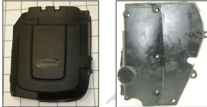
*Image 3.3–18: CDi Engine Cover for the Silverado 1500 (Left) and Mercedes Sprinter 311 CDi (Right)*
