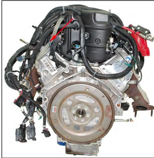
Image 3.18-4: Power train mass cable (ground cable) for the Silverado 1500 and 2500
