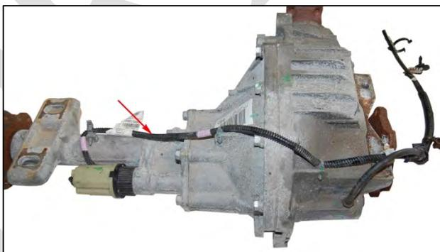
Image 3.18-10: Differential wiring for the Silverado 1500 and 2500
