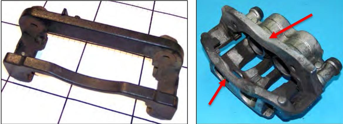
*Image 3.9-17: Front Caliper Mounting Bracket for the Silverado 1500 (Left) and Mercedes Sprinter 311 CDI (Right)*
