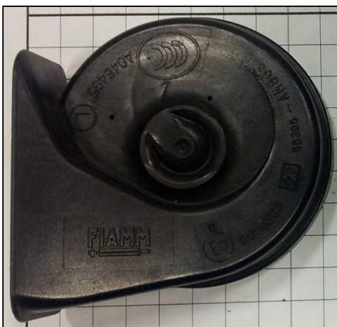
*Image 3.15-5: Horn outer plastic cover (LH/RH) is the same for the Silverado 1500 and 2500
