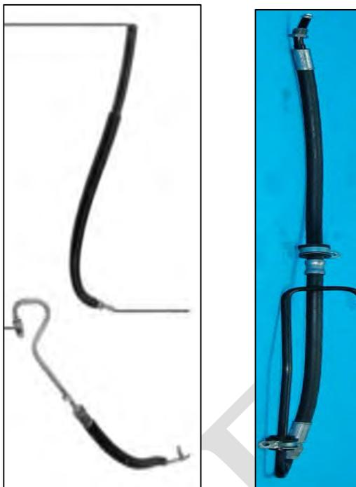
Image 3.13–14: Steering Tubes for the Silverado 1500 (Left) and Renault Master 2.3 (Right)
