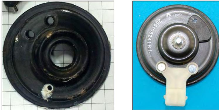
Image 3.15–17: Horn Outside steel cover for the Silverado 1500 and 2500 (Left) and Renault Master 2.3 DCi (Right)
