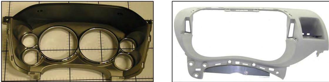
*Image 3.15–15: Cluster Mask Assembly for the Silverado 1500 and 2500 (Left) and Renault Master 2.3 DCi (Right)*
