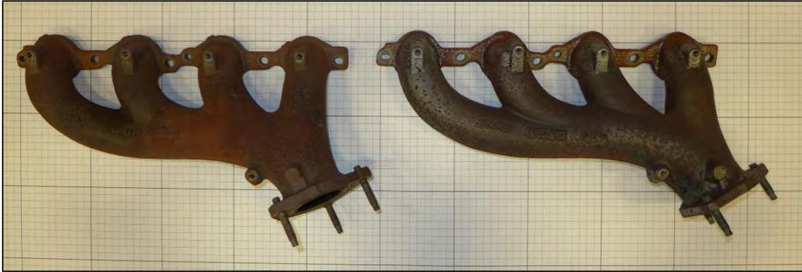
*Image 3.1–5: Exhaust manifold for 5.3 liter LC9 (Left), 6.0 liter LC8 (Right)
