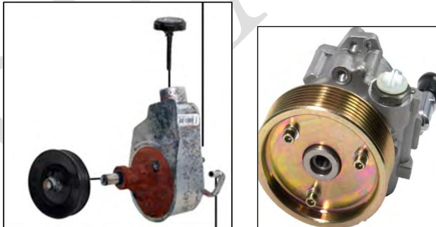
Image 3.13–13: Pump for the Silverado 1500 (Left) and Renault Master 2.3 (Right)
