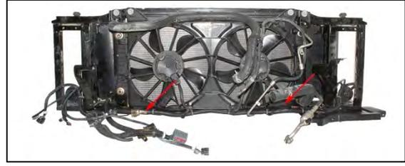
*Image 3.18-2: Front Bumper Harness (Wiring on front module) for the Silverado 1500 and 2500
