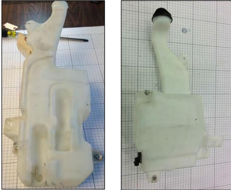
Image 3.6–5: Washer Tank Assembly for the Silverado 1500 (Left) and Silverado 2500 (Right)
