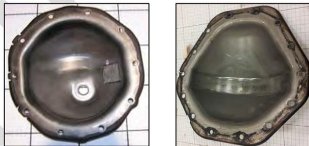
*Image 3.8-5: Rear Axle Cover Plate for the Silverado 1500 (Left) and Silverado 2500 (Right)
