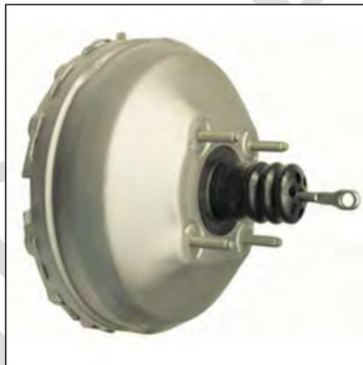
*Image 3.9-22: Vacuum Booster Mass Reduced Sub-Assembly Example*
