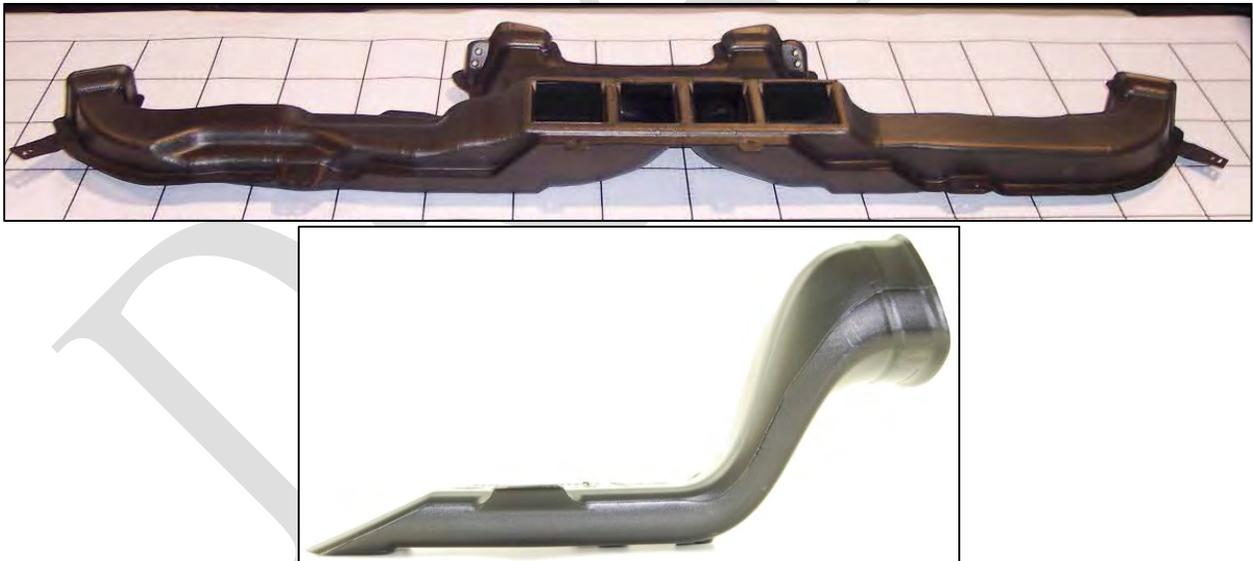
*Image 3.14-8: Air Distribution Duct Components for the Silverado 1500 and 2500 (Top) and Renault Master 2.3 DCi (Bottom)
