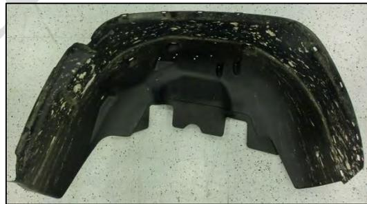
*Image 3.3–5: RH/LH front wheelhouse arch for the Silverado 1500 (Left) and Silverado 2500 (Right)*
