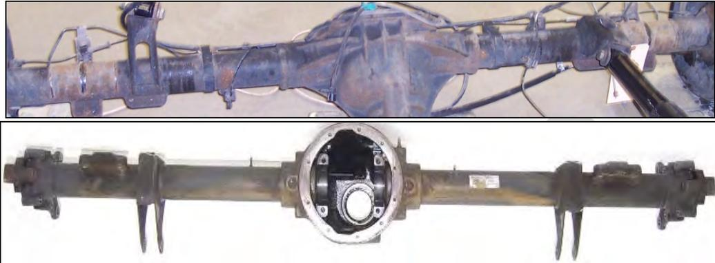
*Image 3.8–17: Rear Axle Sleeve for the Silverado 1500 (Top) and Mercedes Sprinter 311 CDI (Bottom)*
