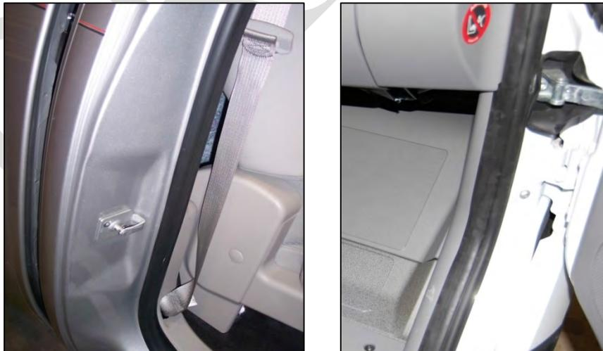
*Image 3.4–8: Sealing Subsystem for the Silverado 1500 (Left) and Mercedes Sprinter 311 CDi (Right)*
