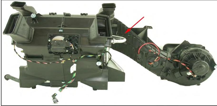
*Image 3.14–6: HVAC Main Unit for Silverado 1500 and 2500 (Top) and Mercedes Sprinter 311 CDI (Bottom)*
