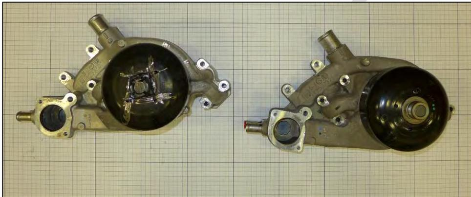
*Image 3.1–12: Water pump for 5.3 liter LC9 (Left) and 6.0 liter LC8 (Right)
