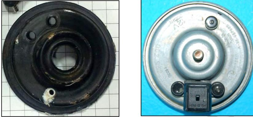
Image 3.15-12: Horn Outside steel cover for the Silverado 1500 and 2500 (Left) and Mercedes Sprinter 311 CDI (Right)
