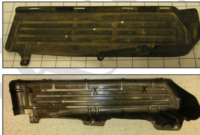
*Image 3.12-3: Fuel Tank Bottom Shield for the Silverado 1500 (Top) and Silverado 2500 (Bottom)*
