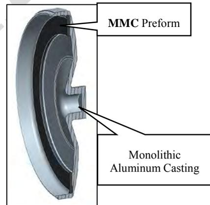
*Image 3.2–6: Example of a cast aluminum converter*
