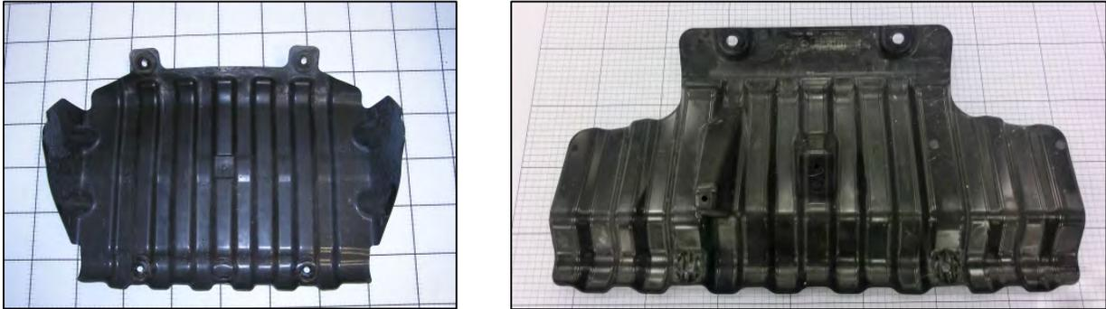
*Image 3.3–6: Front splash shield for the Silverado 1500 (Left) and Silverado 2500 (Right)*
