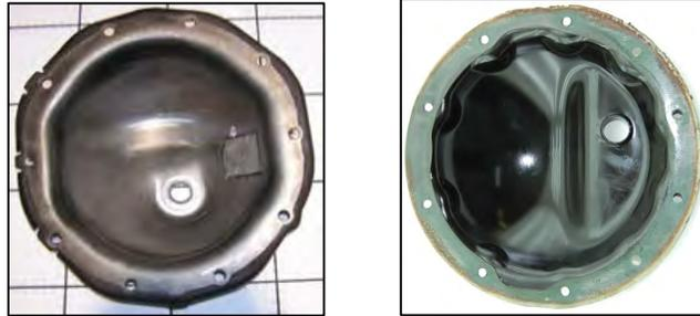
*Image 3.8–19: Rear Axle Cover Plates for the Silverado 1500 (Top) and Mercedes Sprinter 311 CDi (Bottom)*
