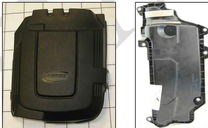
*Image 3.3–25: Engine covers for the Silverado 1500 (Left) and Renault Master 2.3 DCi (Right)*
