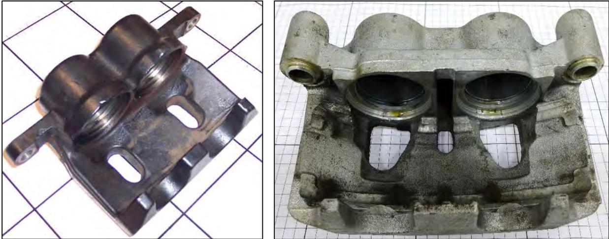
*Image 3.9-3: Front Caliper Housing; 1500 Series (Left), 2500 Series (Right)*
