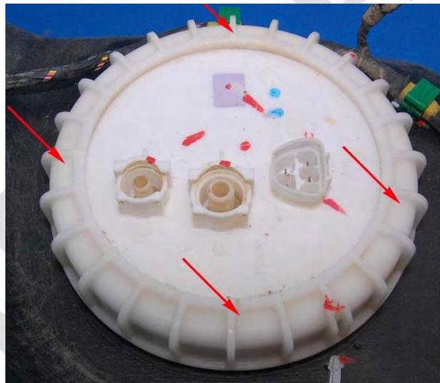
*Image 3.12-5: Example of Plastic POM Fuel Pumping Module Retaining Ring*
