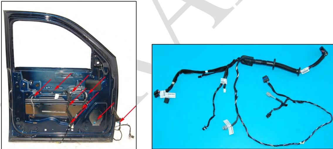
*Image 3.18–31: Front door harness for the Silverado 1500 and 2500 (Left) and Renault Master 2.3 DCi (Right)
