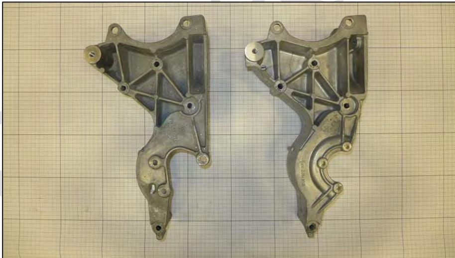
Image 3.1-14: Accessory bracket for 5.3 liter LC9 (Left) and 6.0 liter LC8 (Right)
