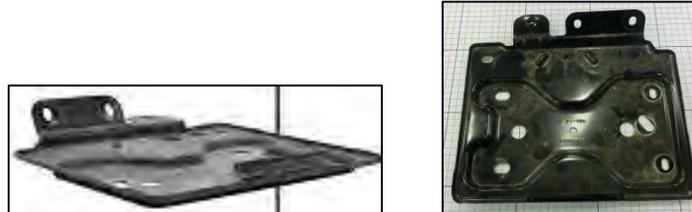
Image 3.16–5: Auxiliary battery tray for the Silverado 1500 (Left) and Silverado 2500 (Right)
