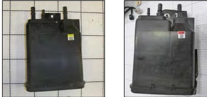
Image 3.12–11: Vapor Canister for the Silverado 1500 (Left) and Silverado 2500 (Right)
