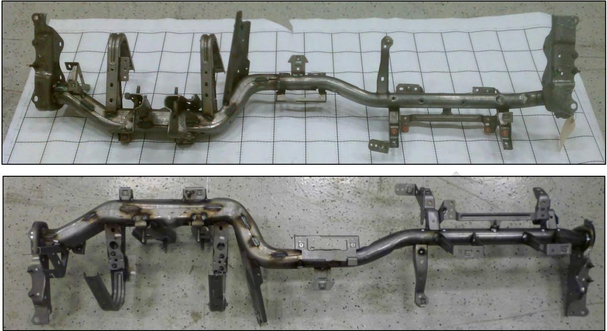
Image 3.4–5: Instrument Panel and Console Subsystem for the Silverado 1500 (Top) and Silverado 2500 (Bottom)
