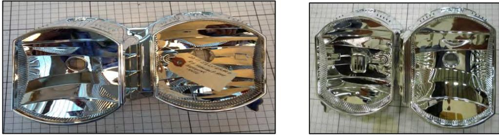
Image 3.17-3: Headlamp inner reflector for the Silverado 1500 (Left) and Silverado 2500 (Right)
