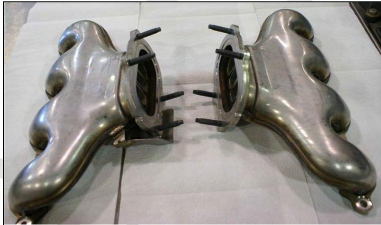
*Image 3.1–6: Fabricated V8 Exhaust Manifold (LS7 Corvette)
