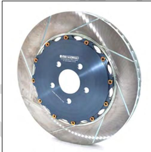
*Image 3.9-2: Front Rotor Mass Reduced Component Example*
