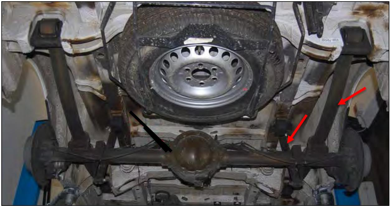
*Image 3.7-14: Mercedes Sprinter Rear Suspension System*
