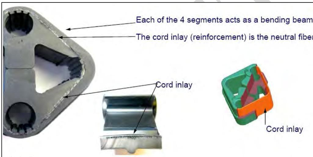
Image 3.11–16: Example of SGF<sup>®</sup> fiber reinforced hanger
