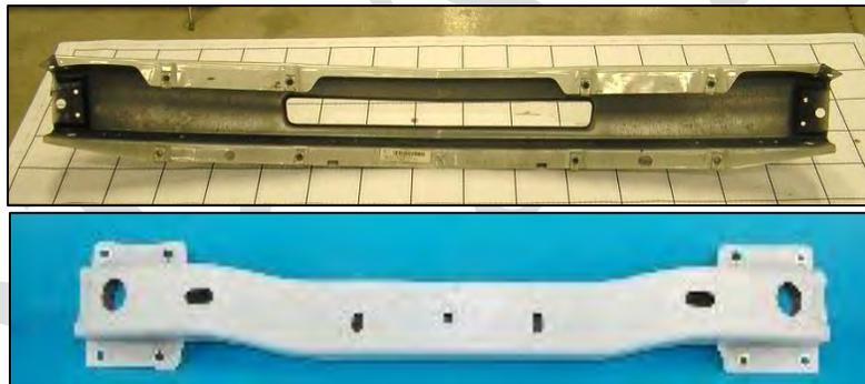
*Image 3.3–29: Front bumper for the Silverado 1500 (Top) and Renault Master 2.3 DCi (Bottom)*
