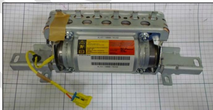
Image 3.4–6: Occupant Restraining Device Subsystem for the Silverado 1500 and Silverado 2500
