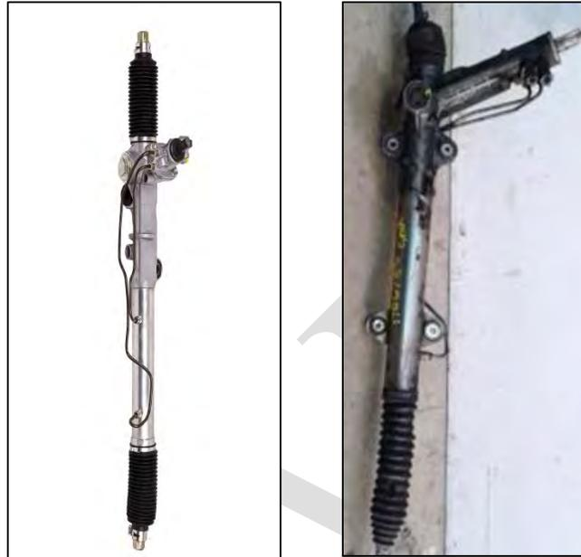
*Image 3.13–6: Steering Gear for the Silverado 1500 (Left) and Sprinter 311 (Right)*
