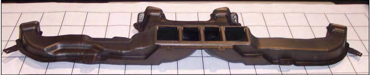
*Image 3.14–2: Air Distribution Duct Components are the same for Silverado 1500 and 2500*
