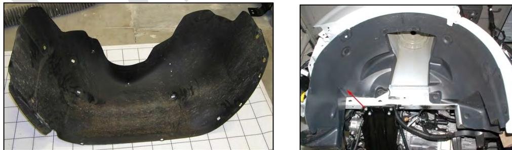
Image 3.3–23: Front wheelhouse arch for the Silverado 1500 (Left) and the Renault Master 2.3 DCi (Right) (Source: FEV, Inc. and www.A2mac1.com)
