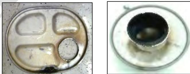
*Image 3.11–13: Muffler end plates for the Silverado 1500 (Left) and Mercedes Sprinter (Right)*
