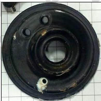
*Image 3.15-6: Horn outside steel cover (LH/RH) is the same for the Silverado 1500 and 2500
