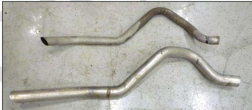
*Image 3.11–10: Muffler pipe for the Silverado 1500 (Top) and Silverado 2500 (Bottom)*
