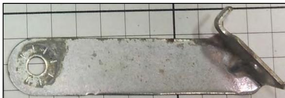
Image 3.15-7: Horn Mounting bracket (LH/RH) is the same for the Silverado 1500 and 2500 (Source: FEV, Inc.)
