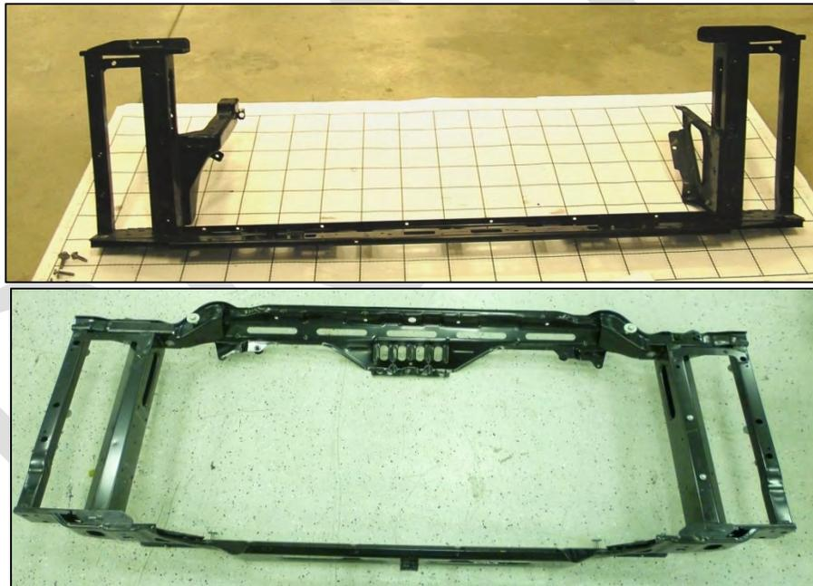
*Image 3.3-3: Radiator structure for the Silverado 1500 (Top) and Silverado 2500 (Bottom)*
