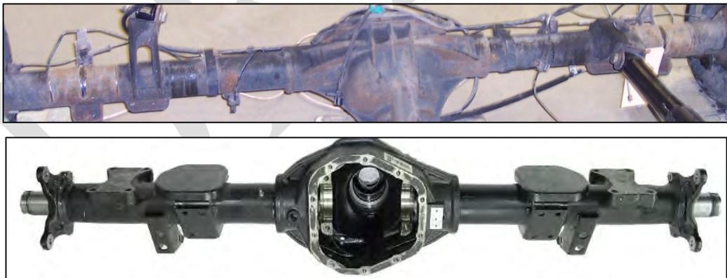
*Image 3.8–24: Rear Axle Sleeves for the Silverado 1500 (Top) and Renault Master 2.3 DCi (Bottom)*
