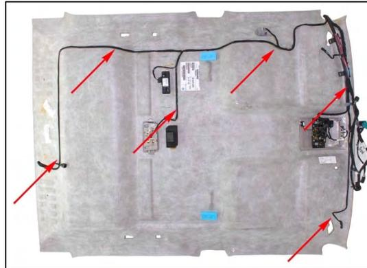
*Image 3.18–18: Headliner wiring for the Silverado 1500 and 2500
