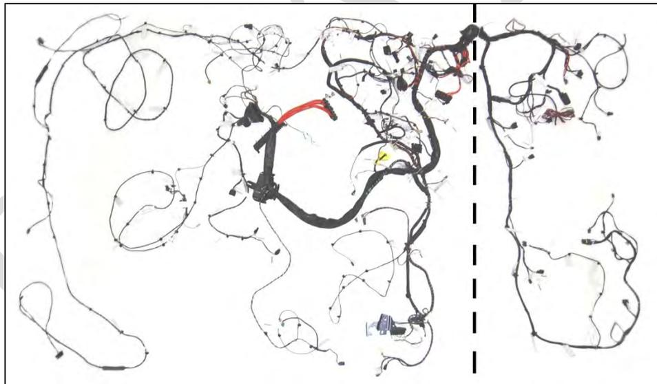
Image 3.18–21: Mercedes Sprinter 311 CDi Electrical Distribution and Electrical Controls System Components (Source: www.A2mac1.com)
