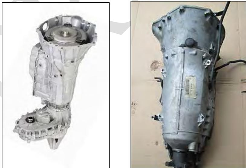
*Image 3.2–9: Transmission for the Silverado 1500 (Left) and Sprinter 311 CDi (Right)*
