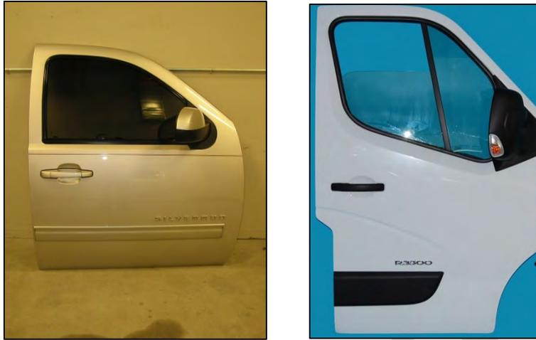
*Image 3.3–28: RH front door assemblies for the Silverado 1500 (Left) and Renault Master 2.3 DCi (Right)*
