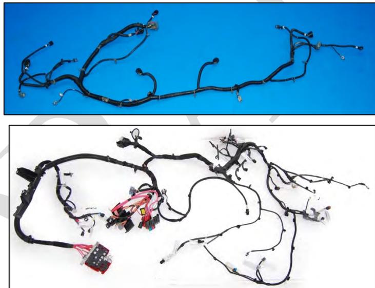
*Image 3.18–26: Engine Wire Harness for the Silverado 1500 and 2500 (Top) and Renault Master 2.3 DCi (Bottom)*
