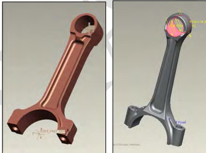
Image 3.1–4: Connecting rod for 5.3 liter LC9 (Left) and C-70 rod (Right)
