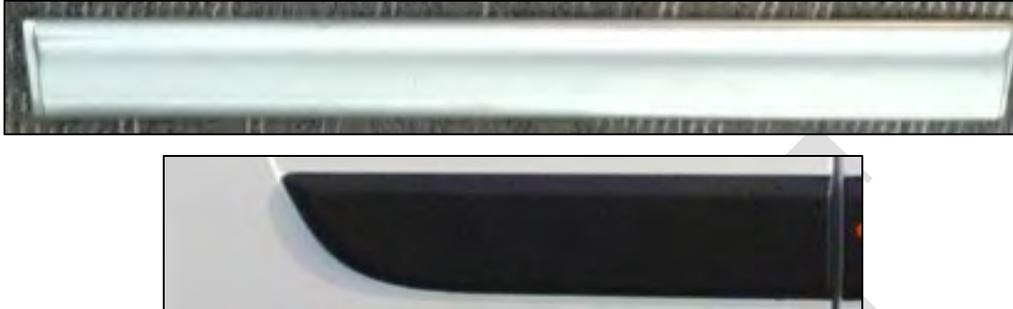
*Image 3.5–20: Bumper Guard (Front Door) for the Silverado 1500 (Top) and Renault Master 2.3 DCi (Bottom)*
