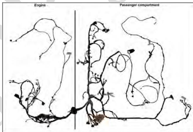
Image 3.18–25: Renault Master 2.3 DCi Electrical Distribution and Electrical Controls System (Source: www.A2mac1.com)
