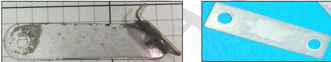
Image 3.15-13: Horn Mounting bracket for the Silverado 1500 and 2500 (Left) and Mercedes Sprinter 311 CDI (Right)
