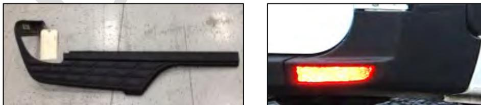
*Image 3.5–17: Rear Bumper Cover (LH/RH) for the Silverado 1500 (Left) and Mercedes Sprinter 311 CDi (Right)*
