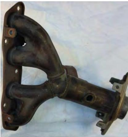
*Image 3.1-7: Fabricated Exhaust Manifold*
