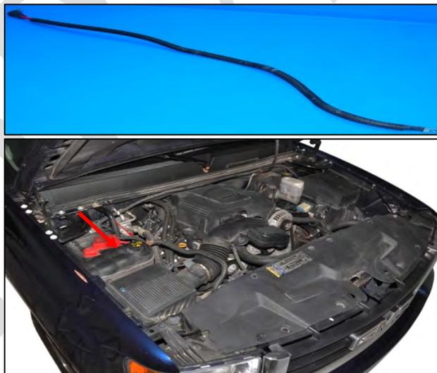
Image 3.18-5: Alternator Power Cable for the Silverado 1500 and 2500
