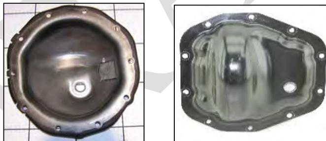
*Image 3.8–26: Rear Axle Cover Plate for the Silverado 1500 (Left) and Renault Master 2.3 DCi (Right)*
