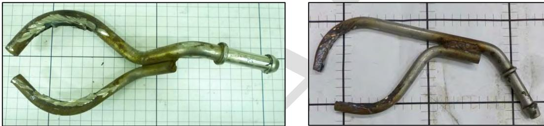
*Image 3.11-4: Steel hanger brackets 1500 (Left), 2500 (Right)*
