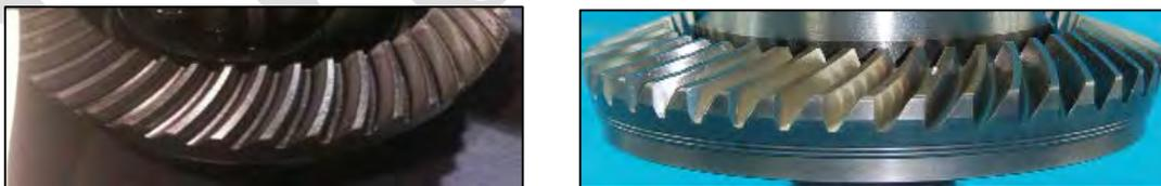
Image 3.8–29: Rear Carrier Ring Gear for the Silverado 1500 (Left) and Renault Master 2.3 DCi (Right)
