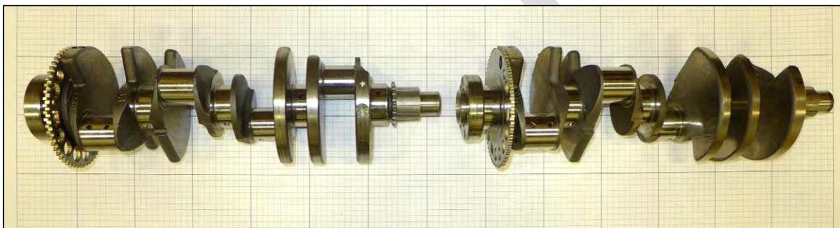
*Image 3.1–8: Crankshaft for 5.3 liter LC9 (Left) and 6.0 liter LC8 (Right)*
