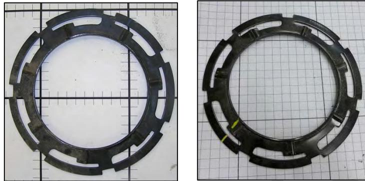
*Image 3.12-4: Fuel Pumping Module Retaining Ring for the Silverado 1500 (Left) and Silverado 2500 (Right)*
