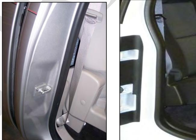
*Image 3.4–3: Sealing Subsystem for the Silverado 1500 (Left) and the Silverado 2500 (Right)*
