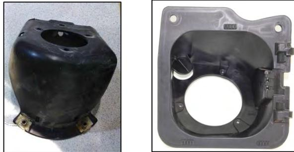
*Image 3.12-16: Fuel Filler Cap Housing for the Silverado 1500 (Left) and Renault Master 2.3 DCi (Right)
