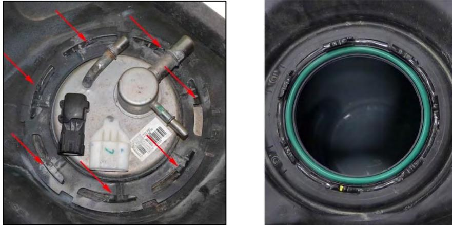
*Image 3.12-2: Fuel Tank Side - Fuel Pump Retaining Ring for the Silverado 1500 (Left) and Silverado 2500 (Right)*
