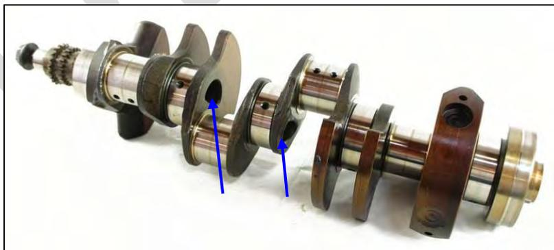
*Image 3.1–9: Cored crankshaft for BMW 4.4L V8*
