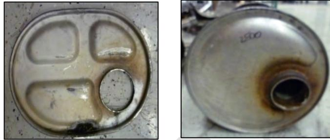
*Image 3.11–9: Muffler end plates for the Silverado 1500 (Left) and Silverado 2500 (Right)*
