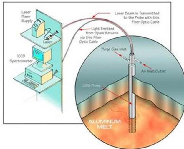
**Figure B.33 Schematic of the LIBS Apparatus<sup>B</sup>**
