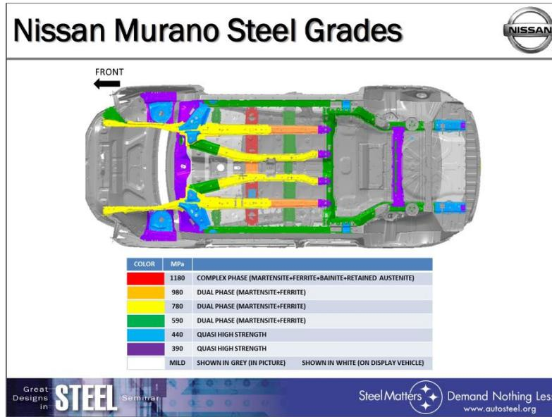
Figure B.15 Nissan Murano Steel Grades for IIHS Compliance - Bottom View<sup>40</sup>
