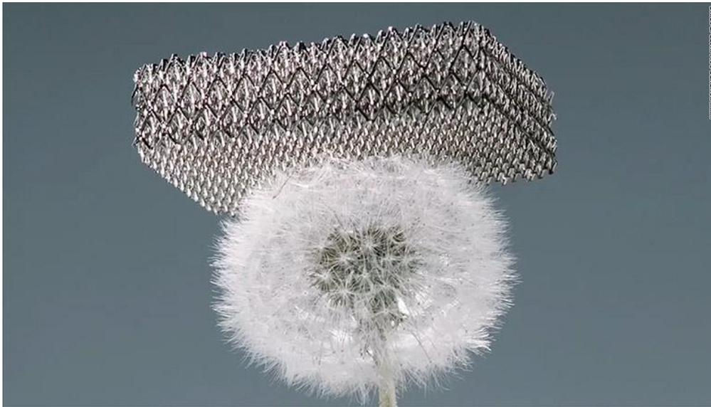
**Figure B.19 Microlattice Material by HRL Laboratories**
