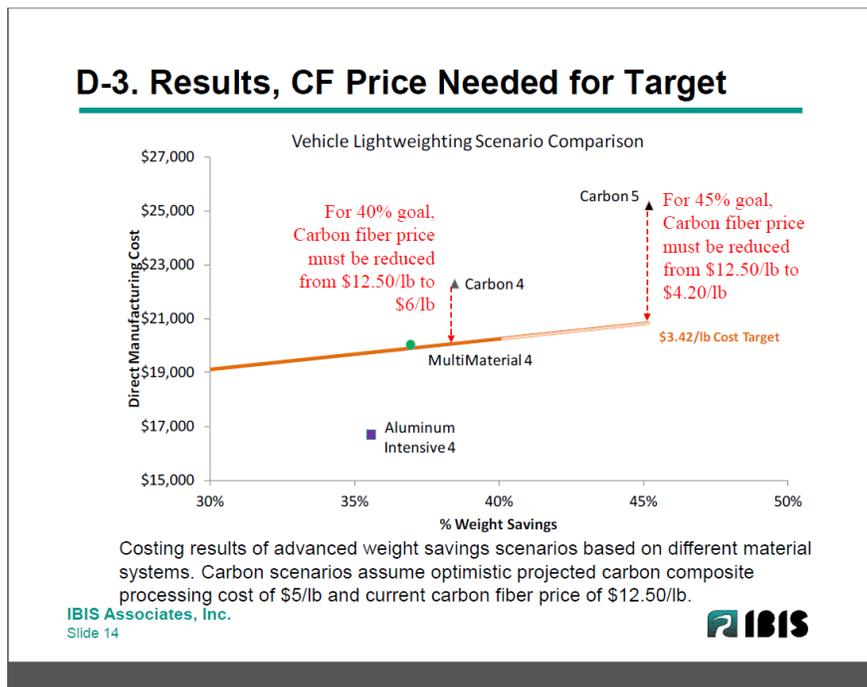
Figure B.51 Technical Cost Modeling for Vehicle Lightweighting 40% and 45% Weight Reduction<sup>117</sup>
