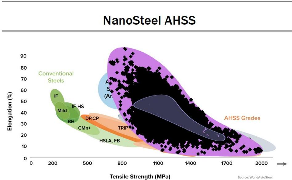
Figure B.17 Comparisons of Established Steel Grades and Potential Nanosteel Grades (in purple)<sup>44</sup>
