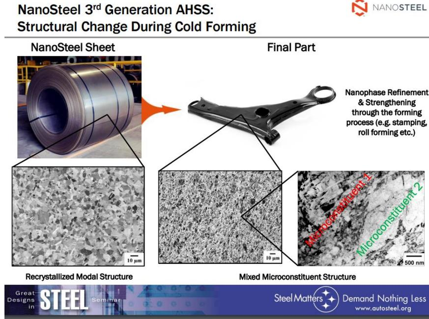
Figure B.18 NanoSteel 3rd Generation AHSS: Structural Change During Cold Forming<sup>44</sup>
