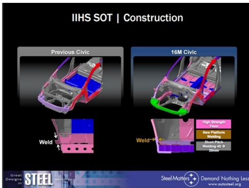
Figure B.16 Honda Civic IIHS Small Overlap Test Construction Upgrades<sup>29</sup>
