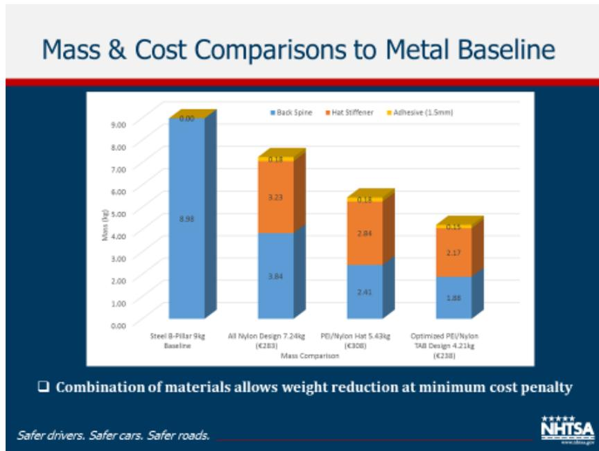
Figure B.54 Mass and Cost Comparisons of Composite Fiber B Pillar to Metal Baseline
