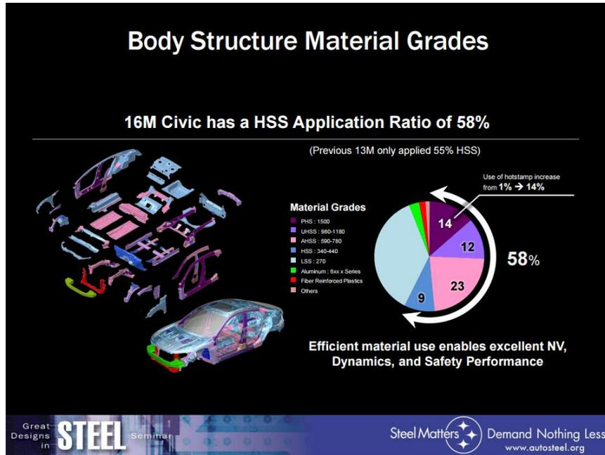
Figure B.8 Body Structure Material Grades for 2016 Honda Civic<sup>29</sup>
