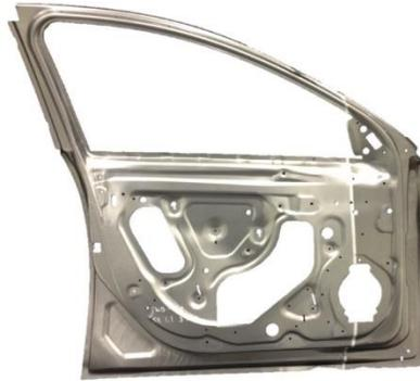
**Figure B.32 Aluminum Door Inner Made with Friction Stir Welding Technique<sup>75</sup>**
