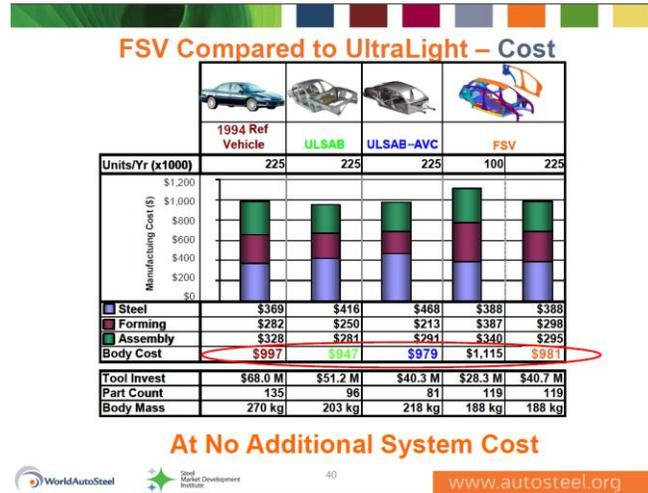
Figure B.12 FSV Comparison to 1994 Reference Vehicle<sup>37</sup>
