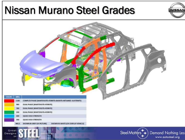
Figure B.14 Nissan Murano Steel Grades used in IIHS Compliance - 3D View<sup>40</sup>
