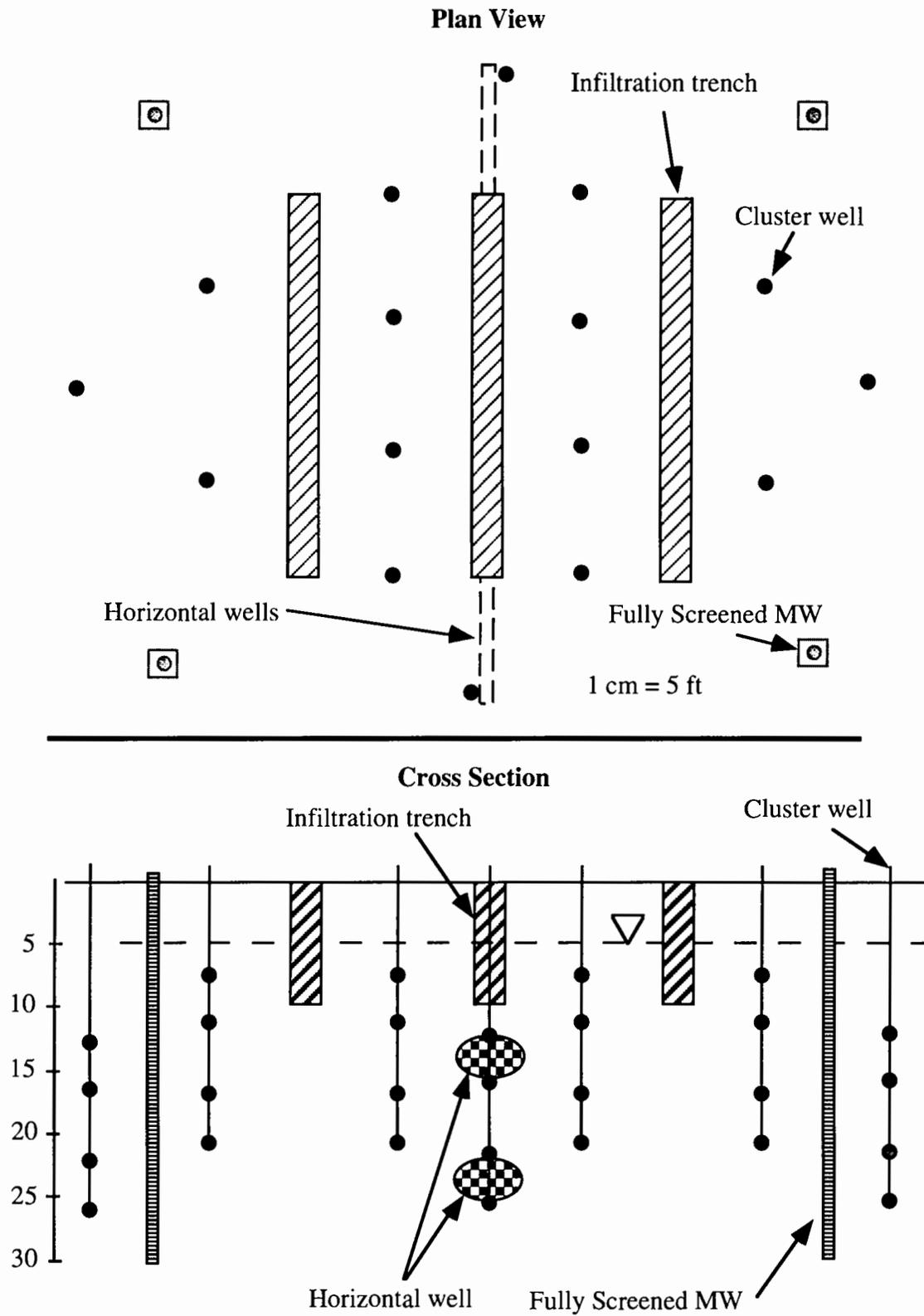
**FIGURE 2.** Schematic of pilot biotreatment system design using infiltration galleries and horizontal wells for extraction/injection, and monitoring system.
