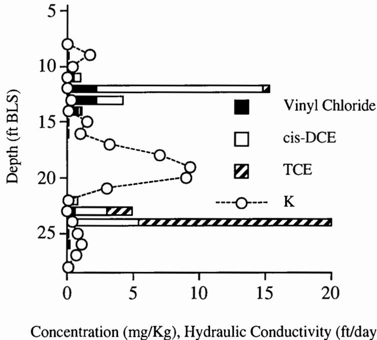
**FIGURE 1.** Absolute hydraulic conductivity of each measured flow interval estimated using a bulk hydraulic conductivity of 2 ft/d obtained near well NEBIOTW-1, and organic contaminant concentrations in soil/pore water samples from composite site cores (PS1 and PS2), vs depth. Depth is relative to top of casing which is approximately land surface.
