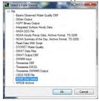
49. Select "WDM Time Series", then "OK". Navigate to the HSPF project folder, and select the file "SDMProject.wdm". It contains the output time series written from HSPF to WDM. [Note: For the pour point simulation, the wdm name should be SDMProject. Although an equivalent \*.wdm file name may be there, do not select met.wdm file.]
