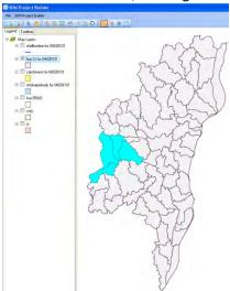
10. Using Zoom In, zoom to this area. Check the "nhdflowline" Map Layer. If it is not at the top of the listing, move it there to ensure it is the outermost projection and will appear on the map.
