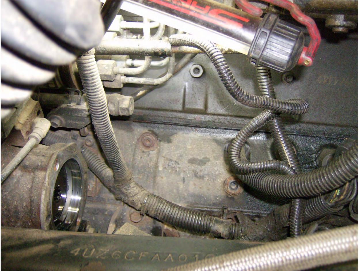
6) Engine block, after hole has been drilled
