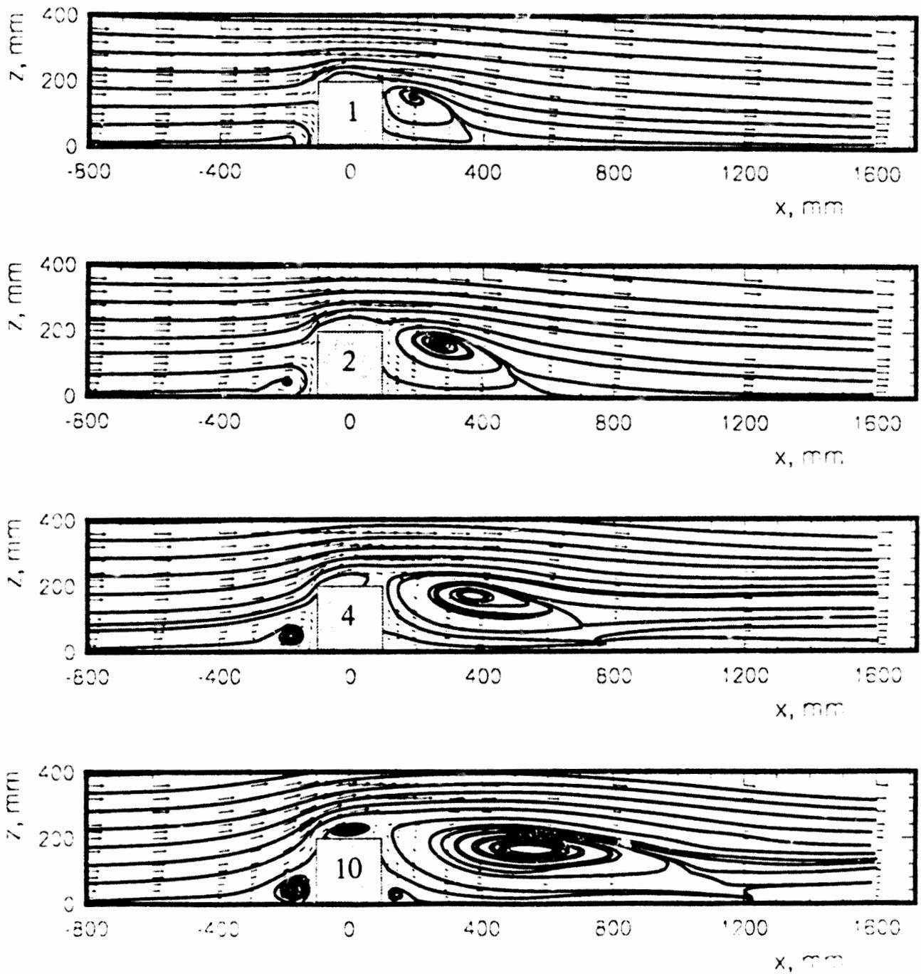
Figure 2. Streamline patterns around buildings of various crosswind widths.
