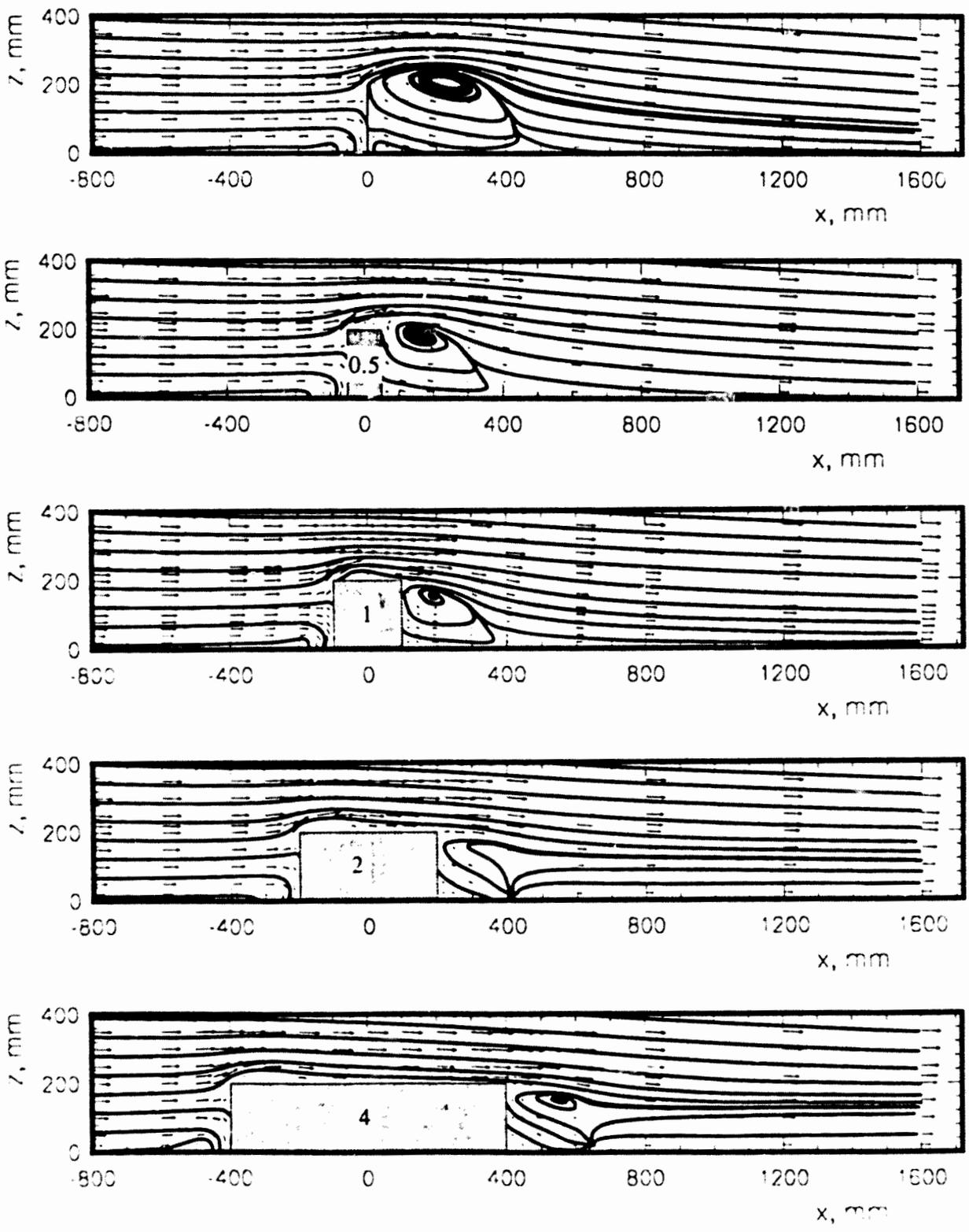
Figure 4. Streamline patterns around buildings of various along-wind lengths. Number on building is L/H. W = H.
