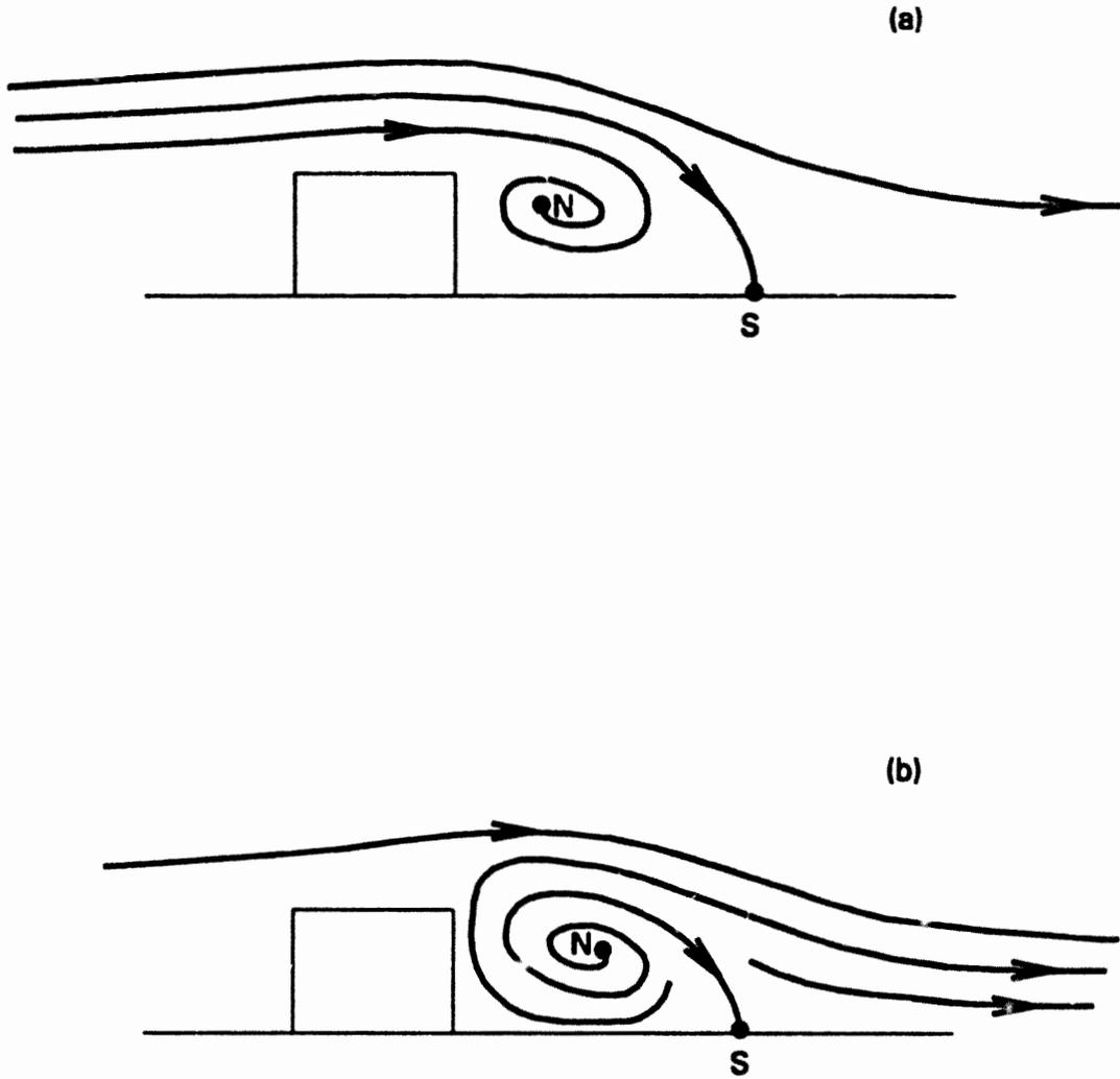
Figure 3. Sketches of basic flow structure as (a) viewed by Hunt et al (1978), where the node N is a separation point, and (b) suggested by current measurements, where the node N is an attachment point.
