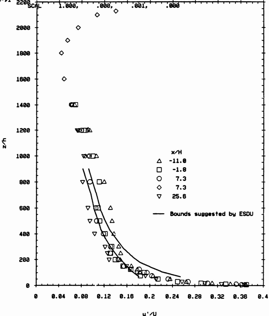
(b) Longitudinal turbulence intensity profiles
