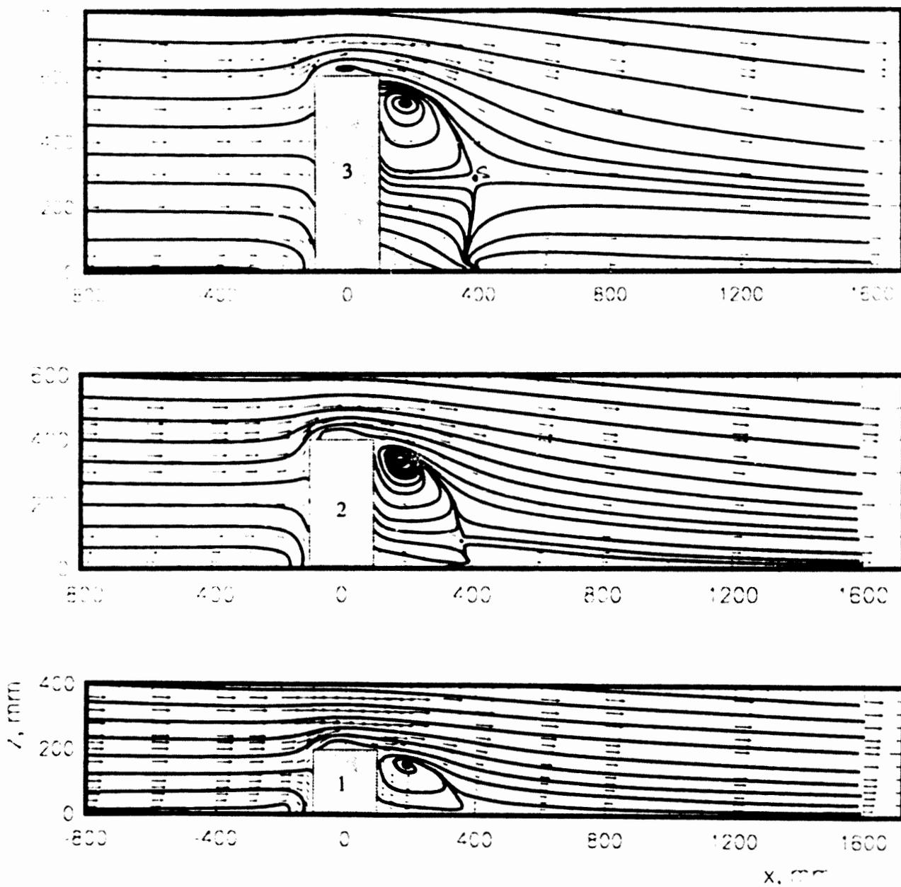
Figure 5. Streamline patterns around buildings of various heights.
