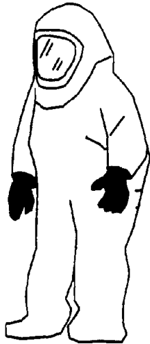
LEVEL A Protection Totally encapsulating vapor-tight suit with full-facepiece SCBA or supplied-air respirator.
