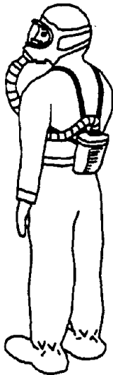
LEVEL C Protection Full-face canister air purifying respirator. Chemical protective suit with full body coverage.
