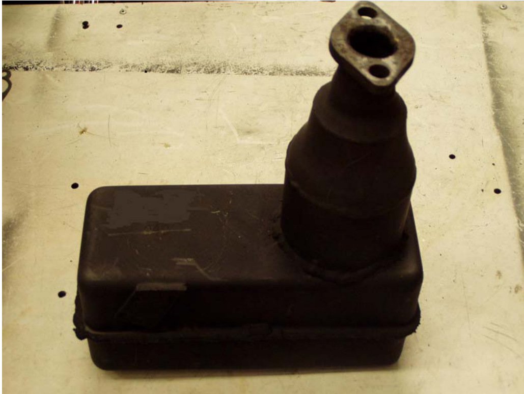
FIGURE A2-31. HIGH EFFICIENCY DUAL CATALYST AHEAD OF MUFFLER
