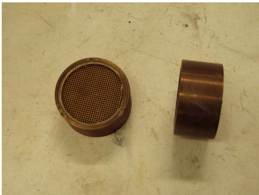
FIGURE A2-14. EPA PROTOTYPE MUFFLER CERAMIC SUBSTRATE FOR HONDA GVC 160
