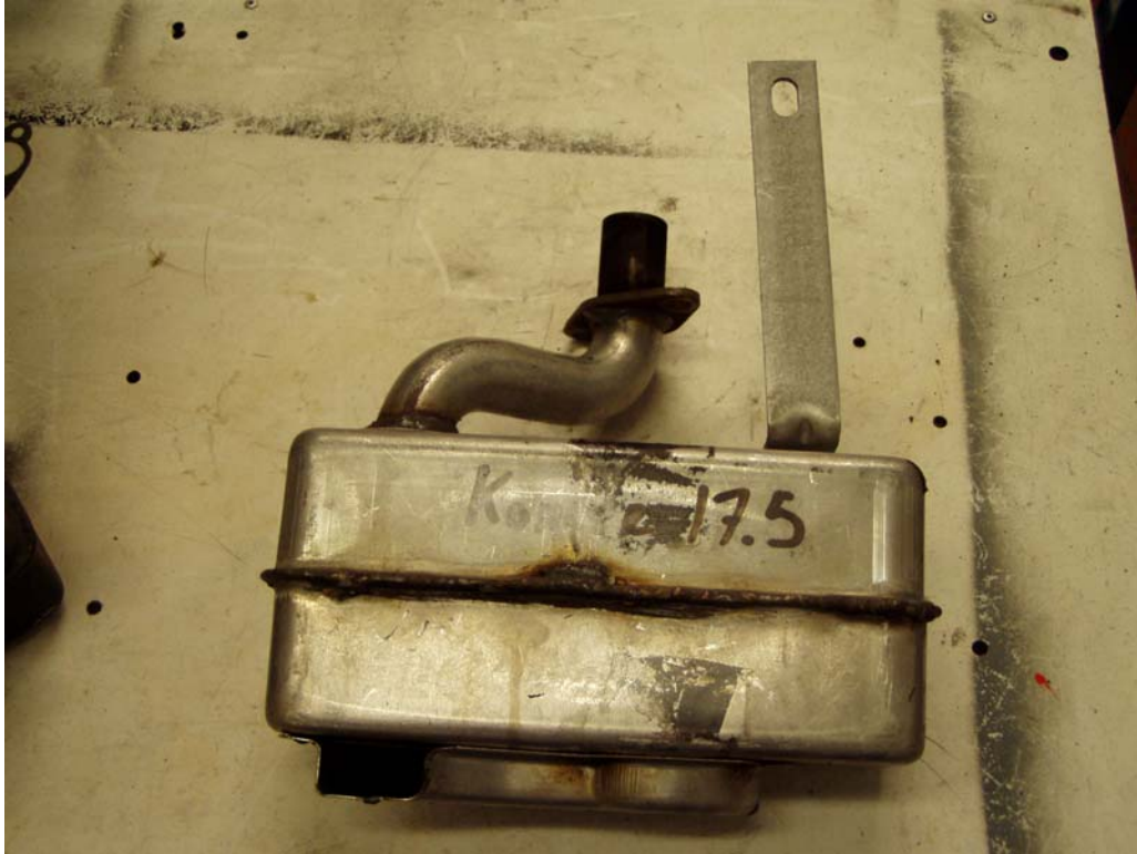
FIGURE A2-29. STOCK MUFFLER WITH INSERTED CATALYST
