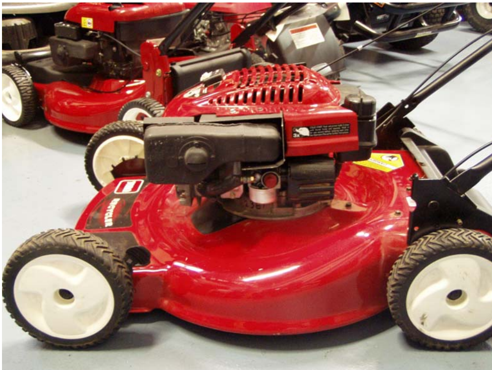
FIGURE A2-24. BRIGGS DUAL METALLIC SUBSTRATE EUROPEAN MUFFLER ON TECUMSEH LV195BA
