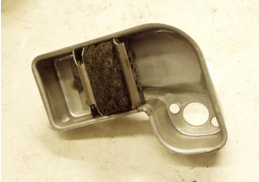
FIGURE A2-17. WIRE MESH CATALYST IN MUFFLER
