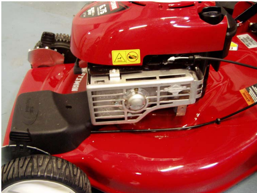
FIGURE A2-20. BRIGGS 6.QUANTUM WITH BRIGGS EUROPEAN CATALYZED MUFFLER
