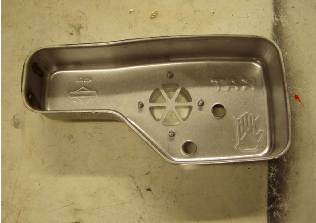
FIGURE A2-5. STOCK BRIGGS QUANTUM SV EUROPEAN CATALYTIC MUFFLER SHROUD
