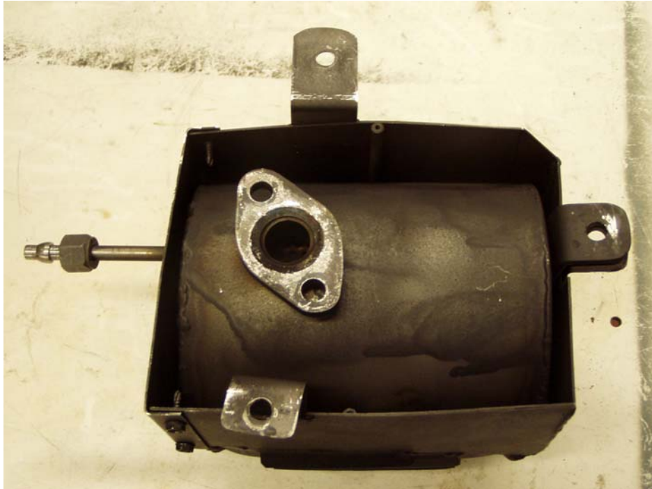
FIGURE A2-11. EPA PROTOTYPE CATALYZED MUFFLER IN SHROUD FOR HONDA GVC 160
