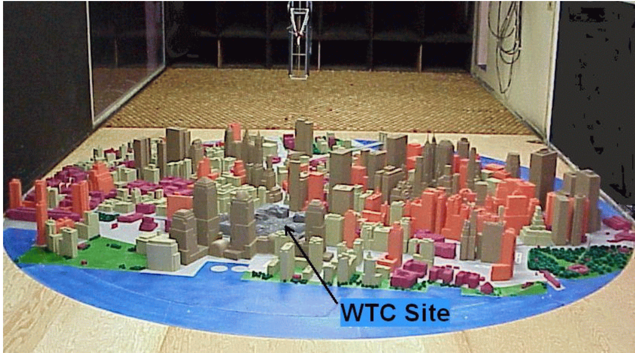
Figure 1. View of scale model in wind tunnel for the 270° wind direction case, looking downstream (toward east).
