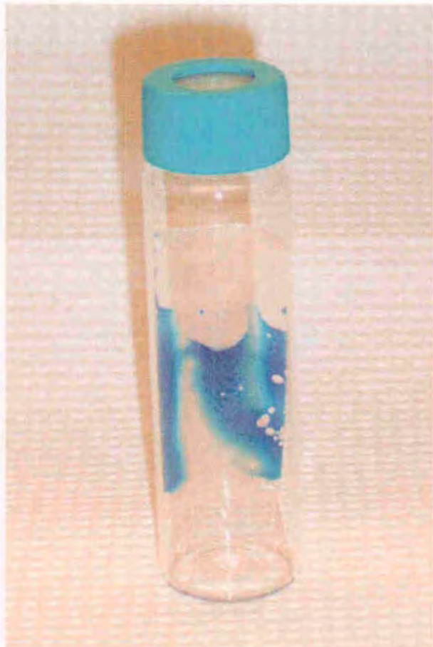
SPMD in 40 mL VOA vial (colored dye added for contrast)
