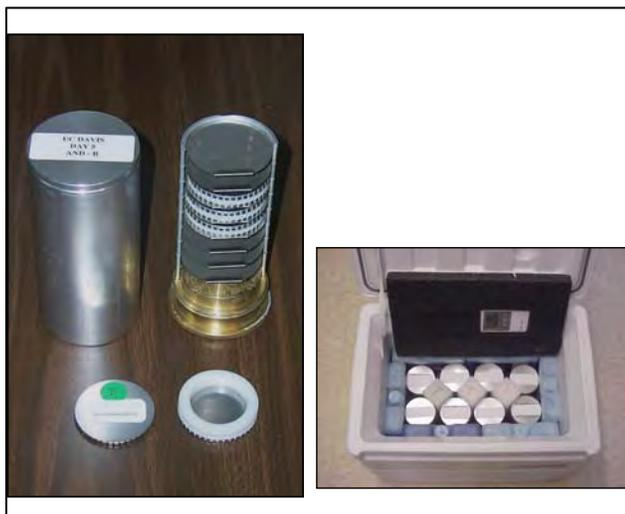
**Figure 3-2.** Photographs of the cassette storage canisters and temperature-controlled coolers.
