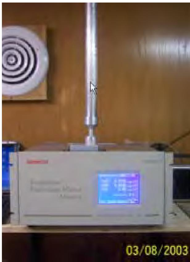
Figure 2-3. Photograph of the Kimoto model SPM-613D beta gauge.
