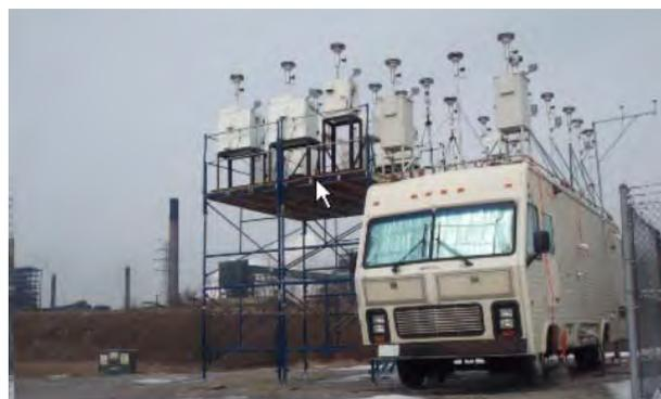
**Figure 3-1.** Photograph of the PM<sub>10-2.5</sub> sampler evaluation platform at the Gary, IN site.
