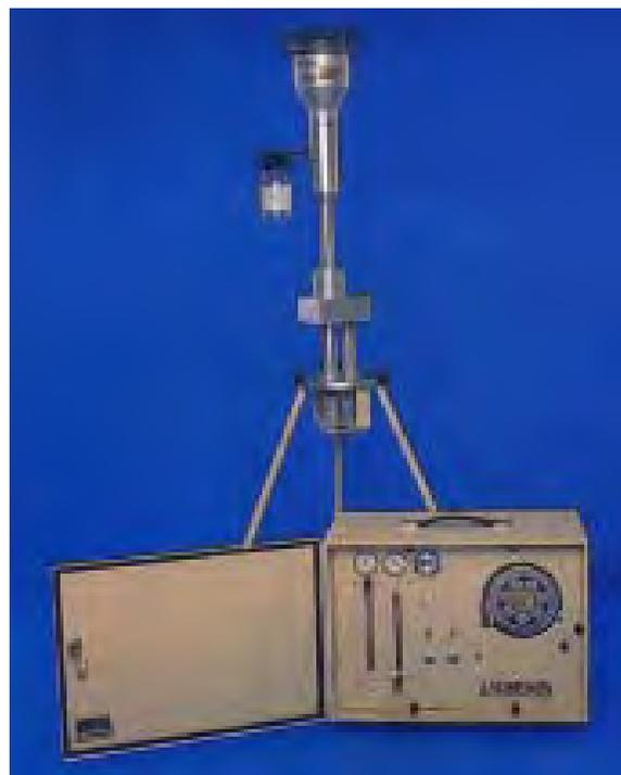
**Figure 2-8.** Photograph of the Sierra-Andersen model 241 dichotomous sampler.
