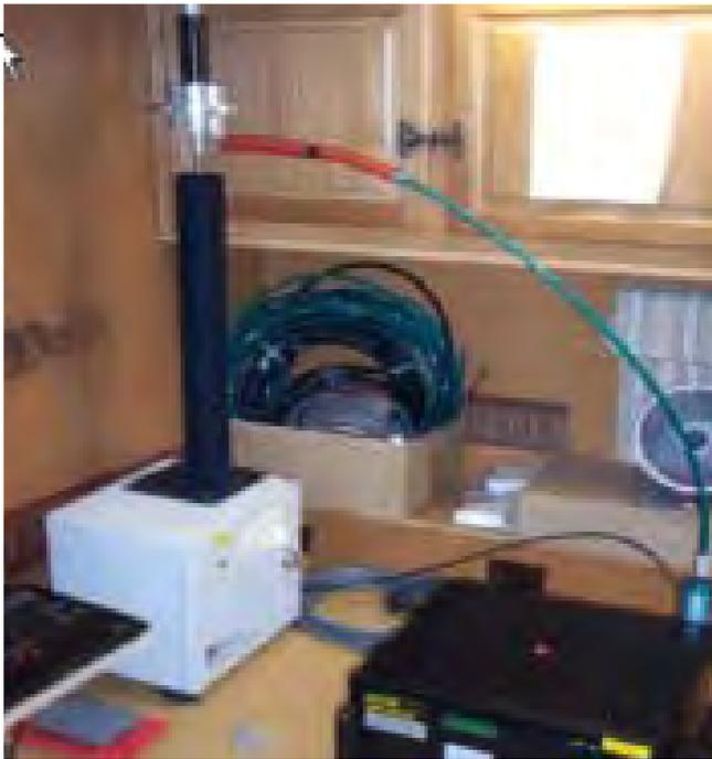
Figure 2-5. Photograph of the R&P PM<sub>10-2.5</sub> TEOM.
