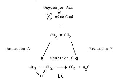
The course of the reaction, either via route A or route B can be directed by proper control of the temperature at the catalyst reaction sites. A brief description of the thermodynamics involved is presented in Table EO-1.
