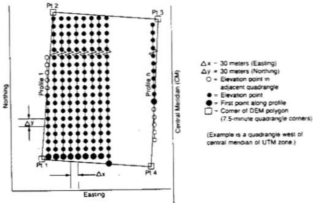
FIGURE 4-1 STRUCTURE OF A 7.5-MINUTE DEM DATA FILE
