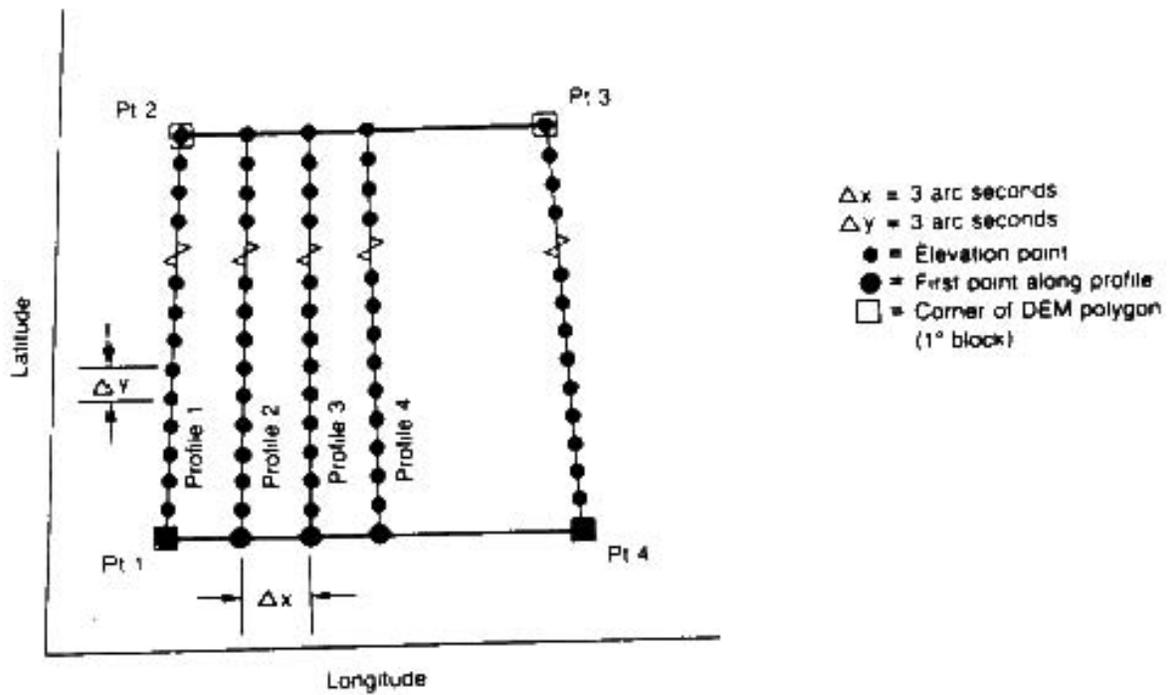
FIGURE 4-2 STRUCTURE OF A 1-DEGREE DEM DATA FILE FOR THE LOWER LATITUDES
