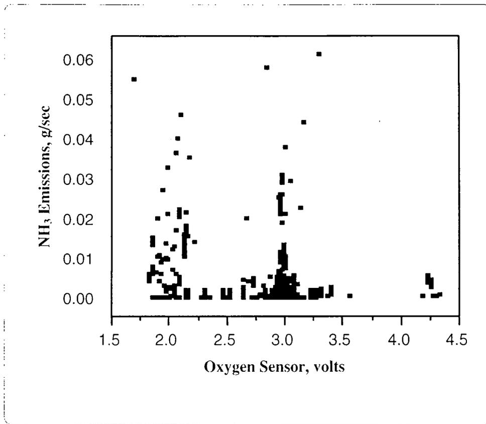
**Figure 10.** The relationship of ammonia emissions for oxygen concentration, reflecting data from only one of the hard acceleration cycles tested.
