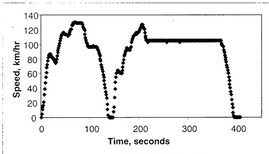
**Figure 4.** Speed versus time trace for the hard acceleration cycle.
