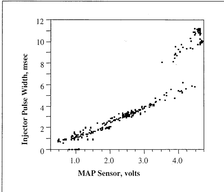
**Figure 5.** The relationship between injector pulse width and the intake manifold absolute pressure. The break in the graph is where enrichment combustion conditions were being commanded by the engine computer.
