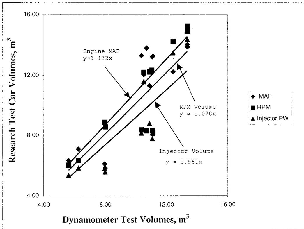
**Figure 6.** Comparison of the air volumes determined using the instrumented vehicle and the air volumes determined by the dynamometer facility.
