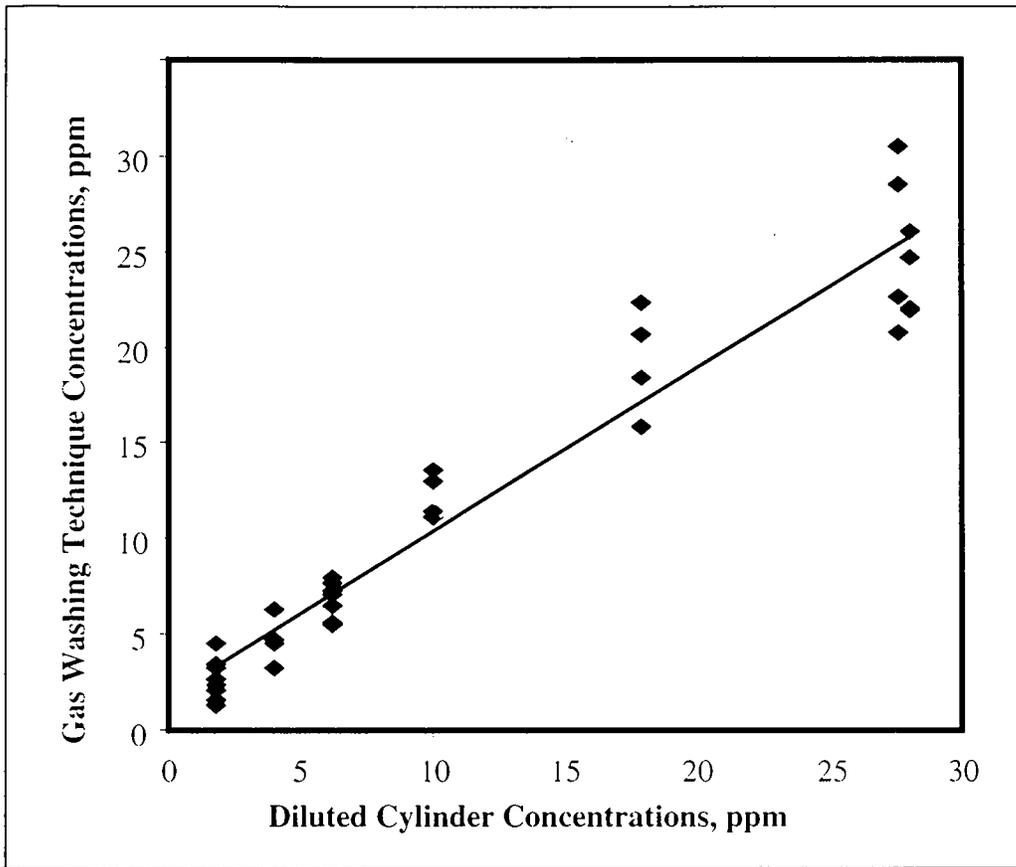
**Figure 1.** Comparison of the gas washing technique measured concentrations to the ammonia gas standard diluted concentrations.
