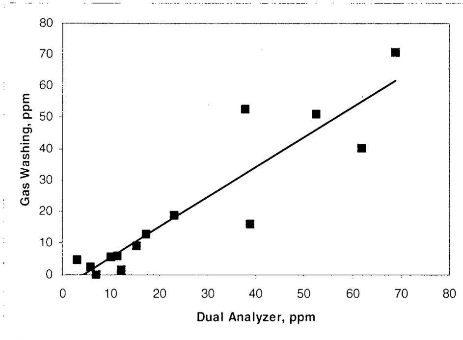
**Figure 3.** Comparison of the dual analyzer technique measured ammonia concentrations to the gas washing technique measured ammonia concentrations.
