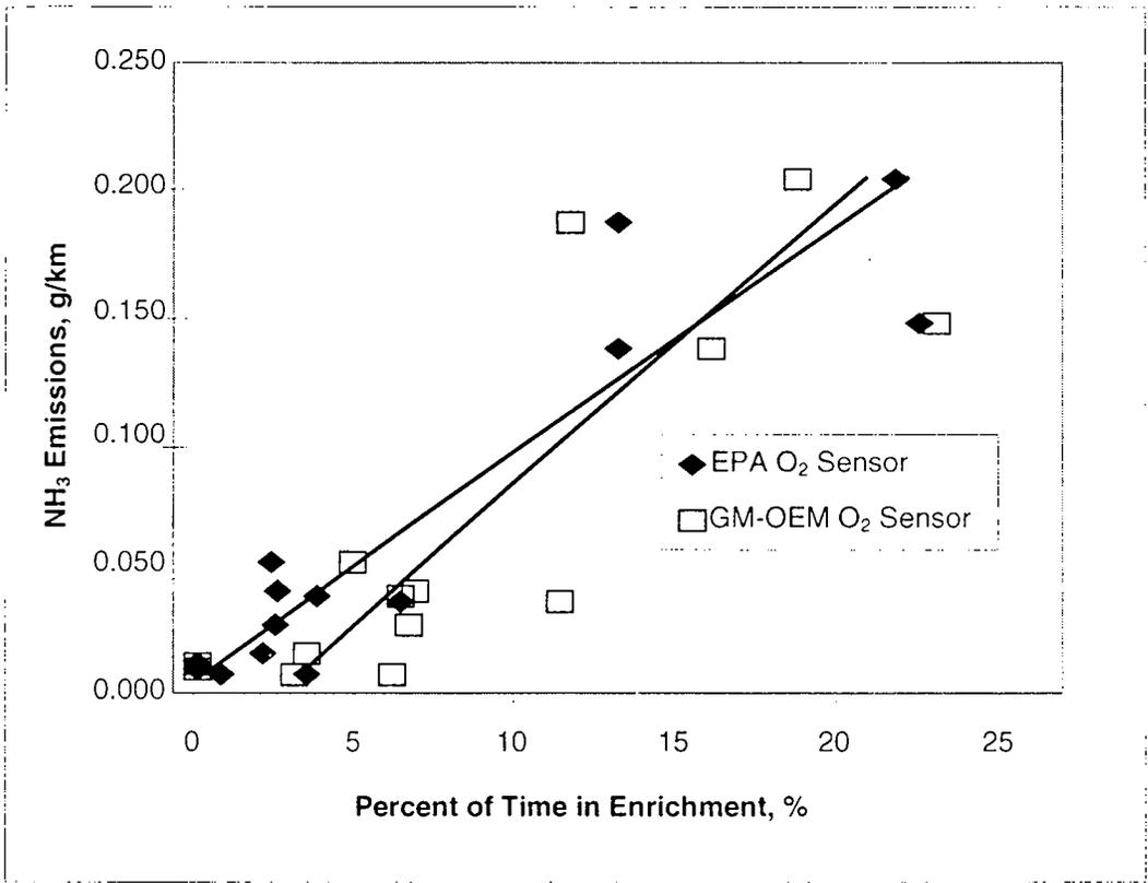
**Figure 8.** Percentage of time that the engine was operated in an enrichment mode as indicated by both the EPA and GM-OEM oxygen sensors.
