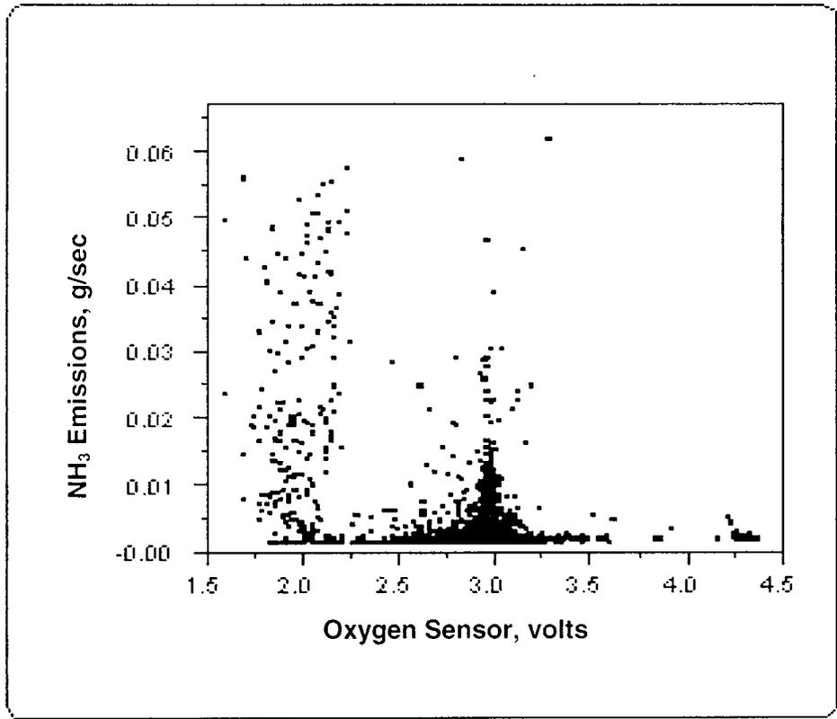
**Figure 9.** The relationship of ammonia emissions for oxygen concentration, reflecting results from all 14 cycles tested.
