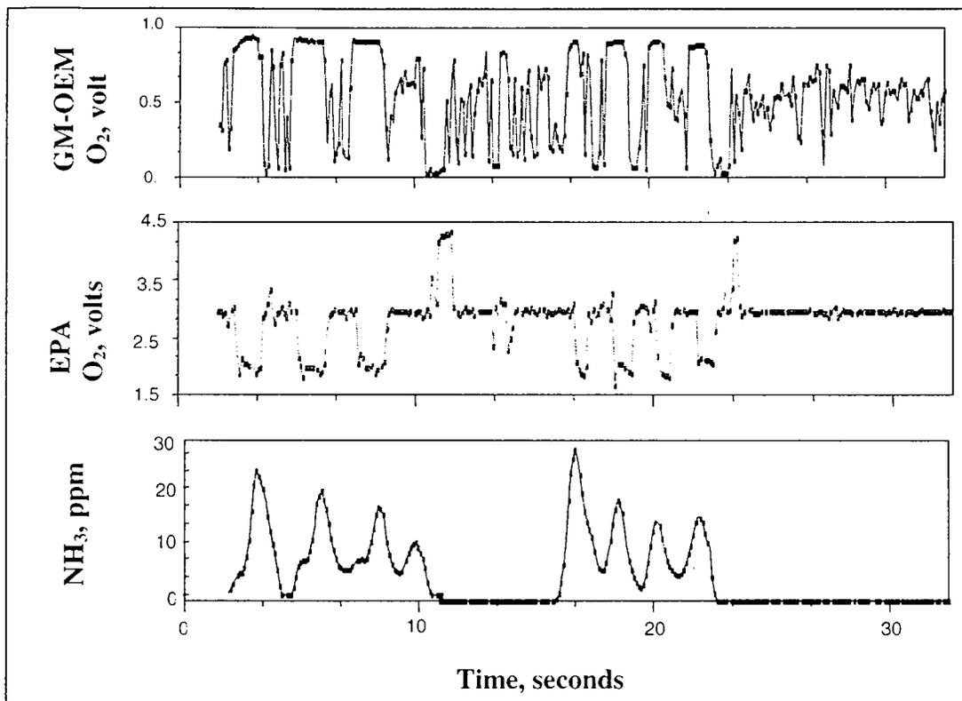
**Figure 7.** Change in oxygen concentration in relationship to the production of ammonia. Also an indication of the signal-to-noise ratio between the original GM-OEM oxygen sensor and the EPA-installed oxygen sensors.
