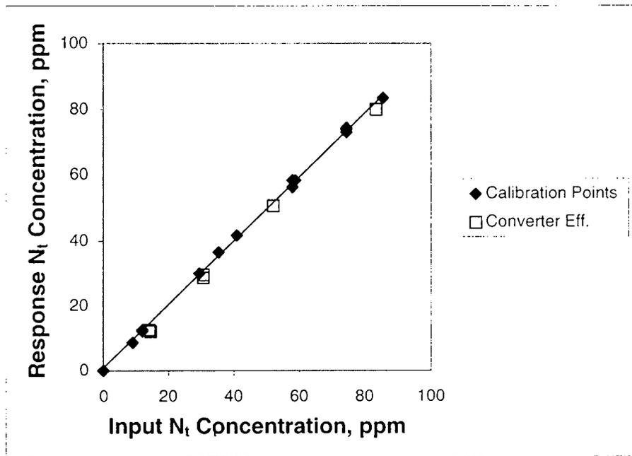
**Figure 2.** Comparison of the Scott Specialty Gases calibration standards and the Teco analyzer response. These data include the calibration responses, converter efficiency checks, and calibration checks conducted between tests.
