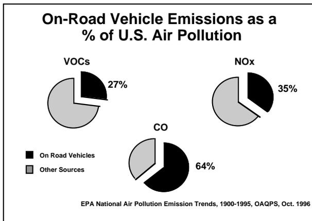
from motor vehicles since the early-1970s. Today's new cars are approximately 95 percent cleaner per mile relative to new cars of the 1960s due to technologies such as catalytic converters, on-board computers, fuel injection systems, and evaporative emission controls. Nevertheless, transportation still accounts for a large part of national air pollution. On-road vehicles
