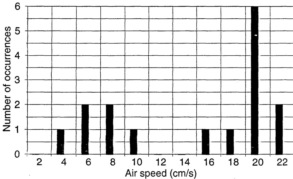
Figure 7 Histogram of air speeds measured 1 cm over wood floor in large chamber.
