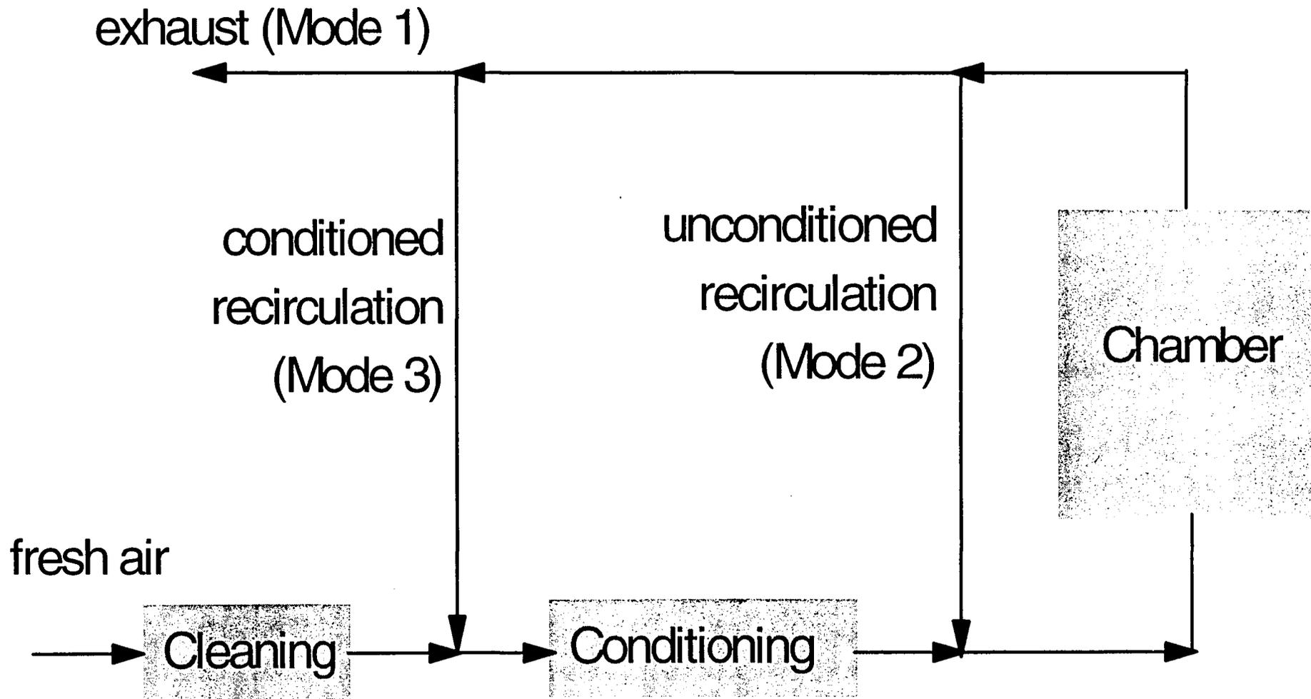
Figure 2 Large chamber flow diagram.
