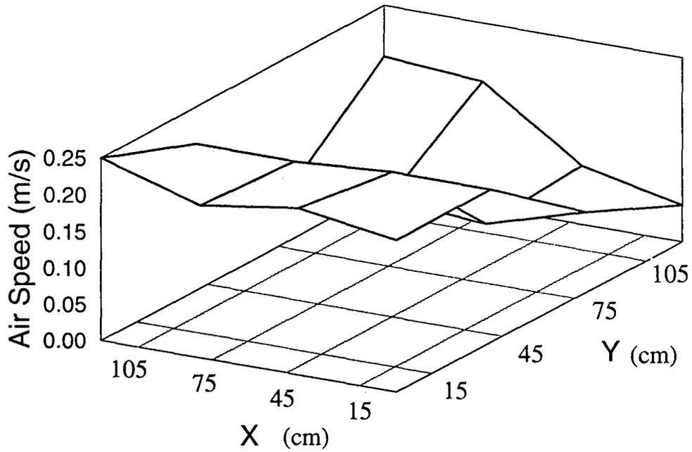
Figure 5 Air speed 1 cm above wood floor placed in center of large chamber floor.
