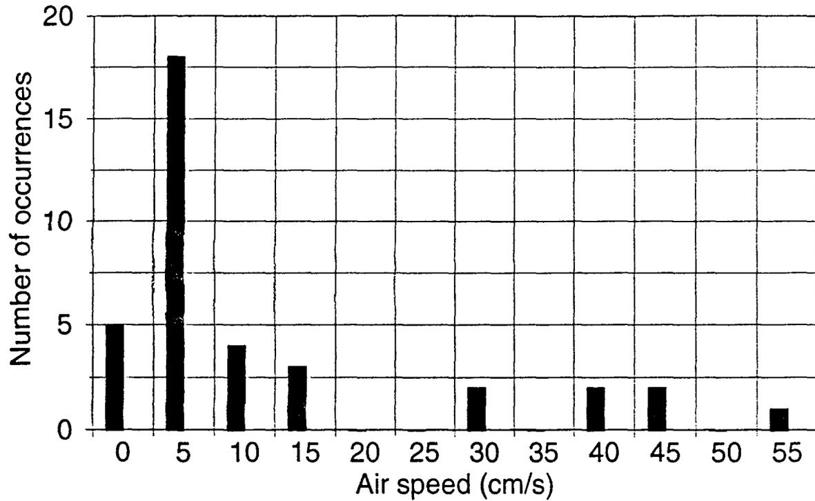
Figure 6 Histogram of air speeds measured 1 cm from test house walls.
