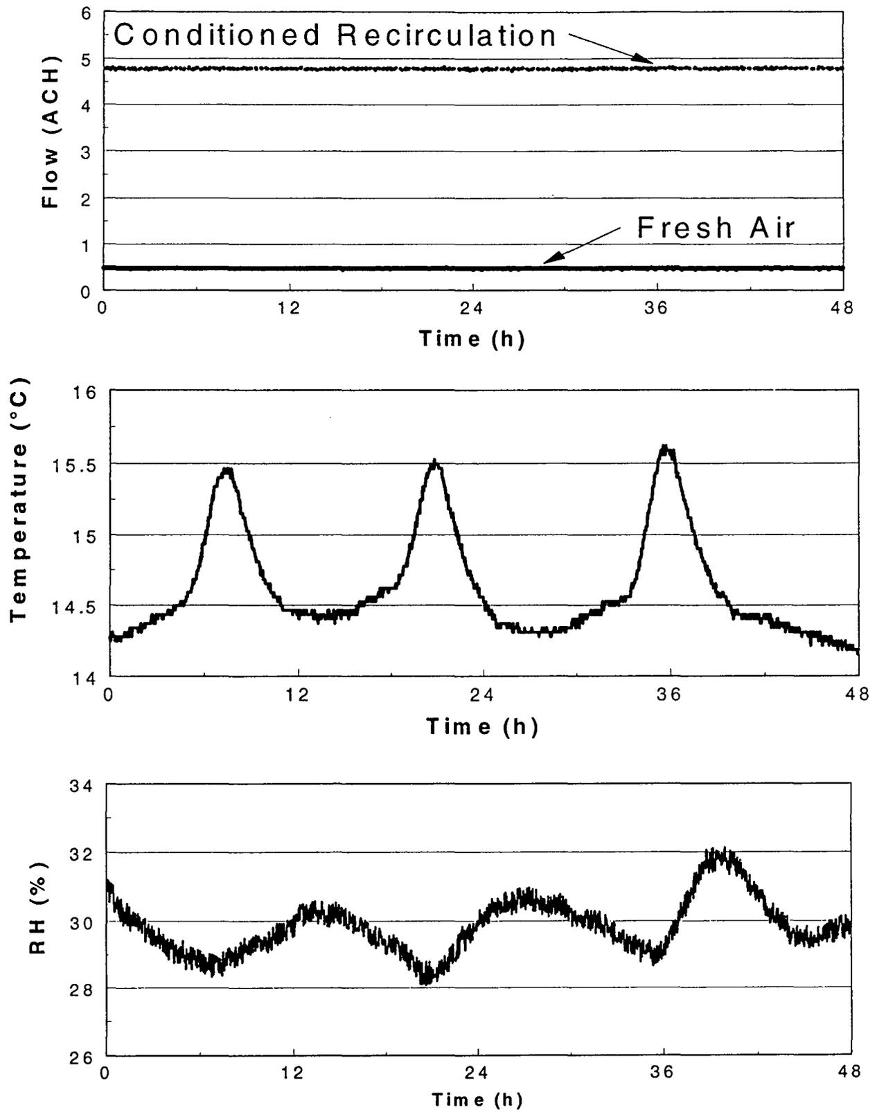
Figure 3 Large chamber control at 15°C and 30% RH.
