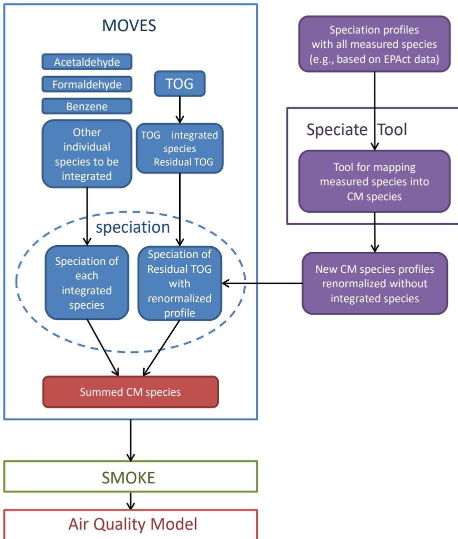
Figure 1. Diagram of the process of TOG speciation for air quality modeling as it occurs with MOVES2014
