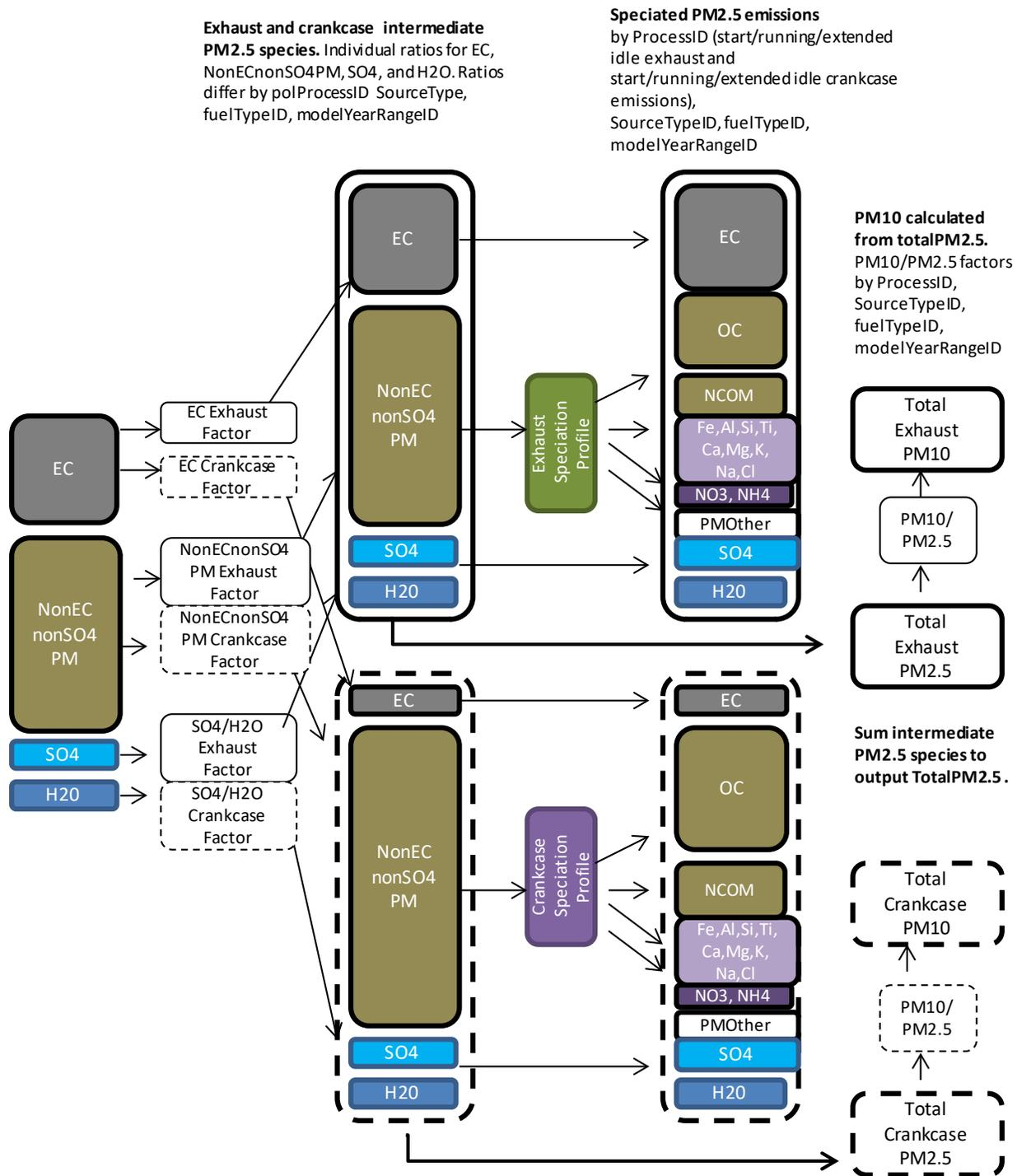
**Figure 3. Flow Chart of Calculation of exhaust and crankcase PM<sub>2.5</sub> and PM<sub>10</sub> emission rates, and PM<sub>2.5</sub> exhaust and crankcase speciation**
