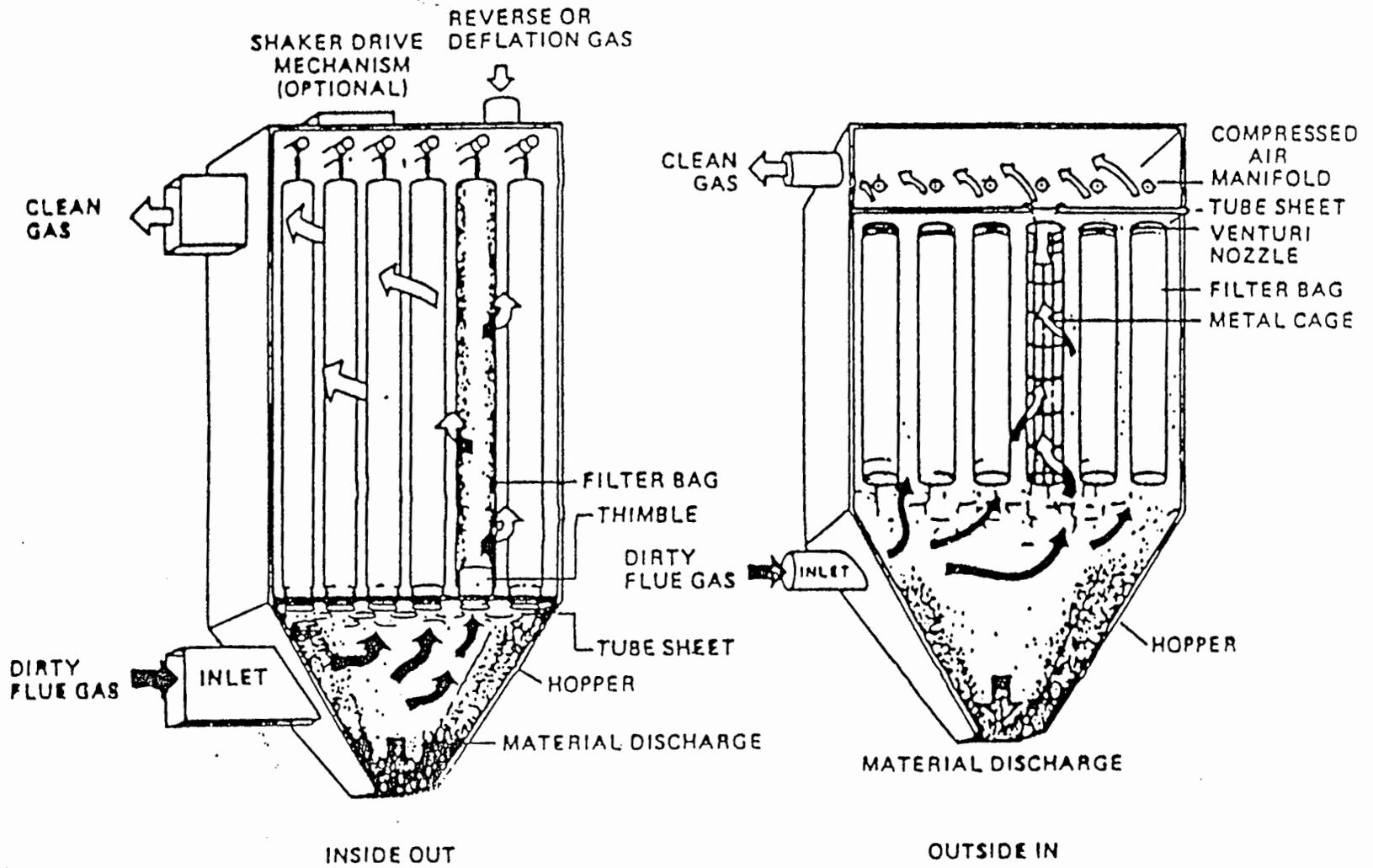
Figure 4. Reverse Air and Pulse Jet Baghouses
