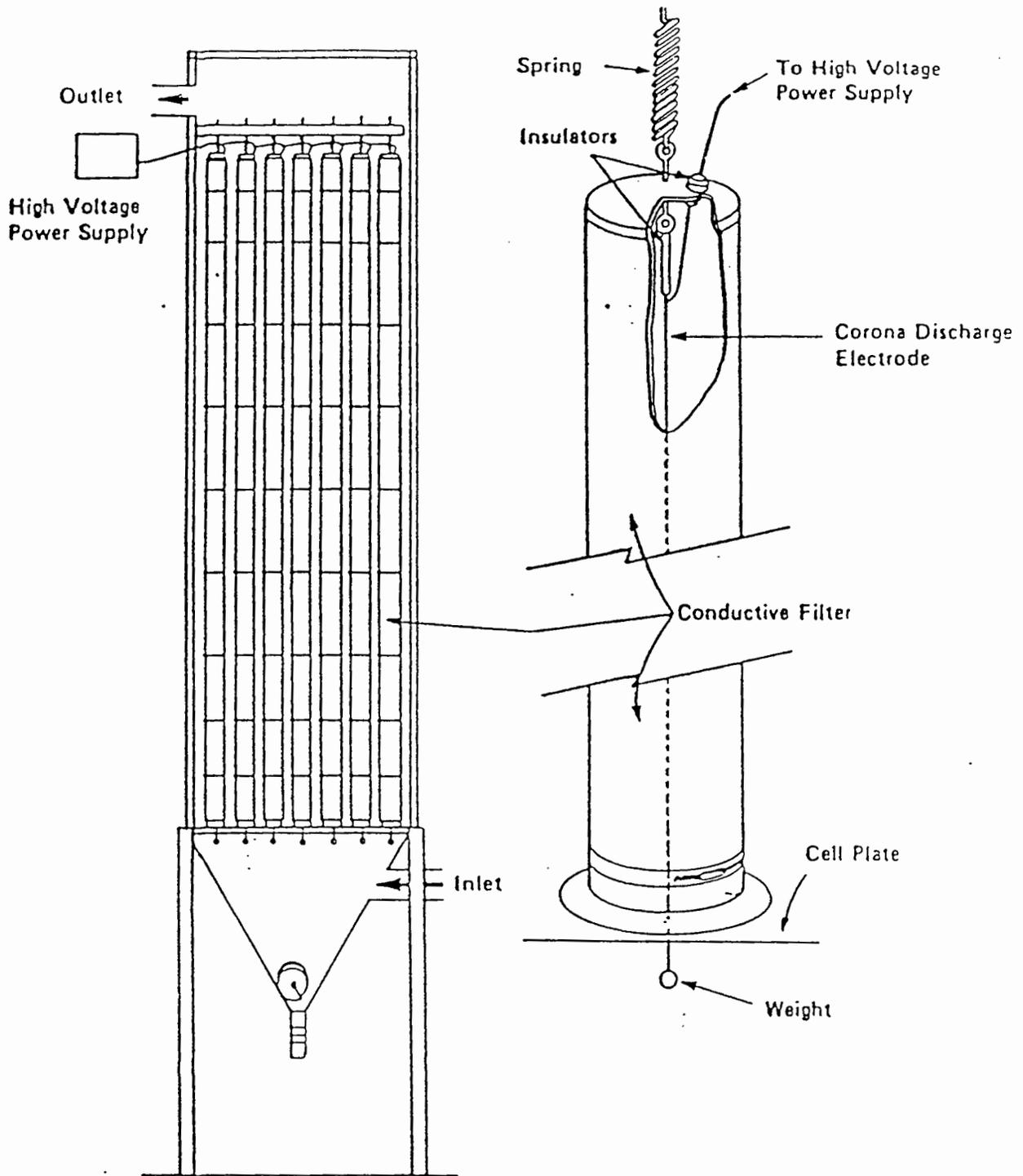
**Figure 5. Electrostatically Augmented Reverse Air Baghouse**
