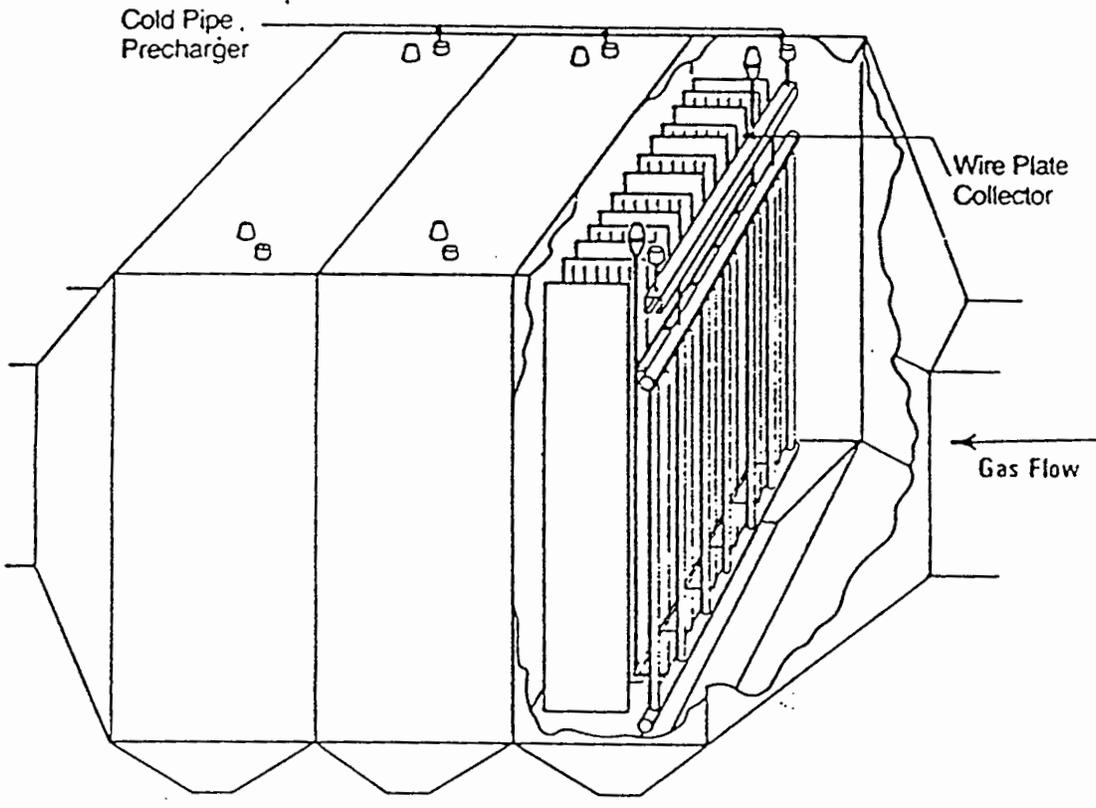
**Figure 2. Multi-Stage Electrostatic Precipitator**
