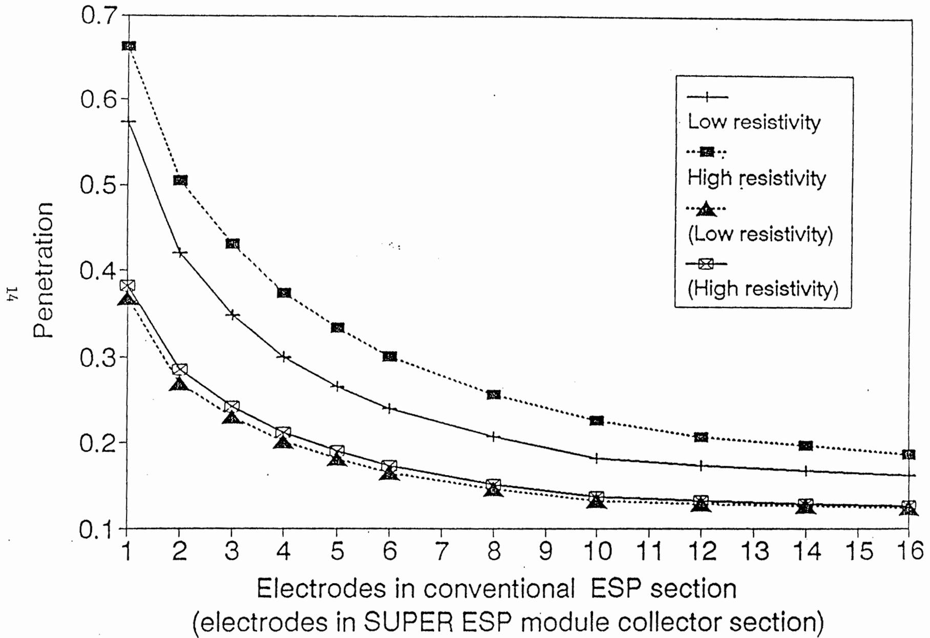
Figure 3. Predicted Super ESP and Conventional ESP Performance
