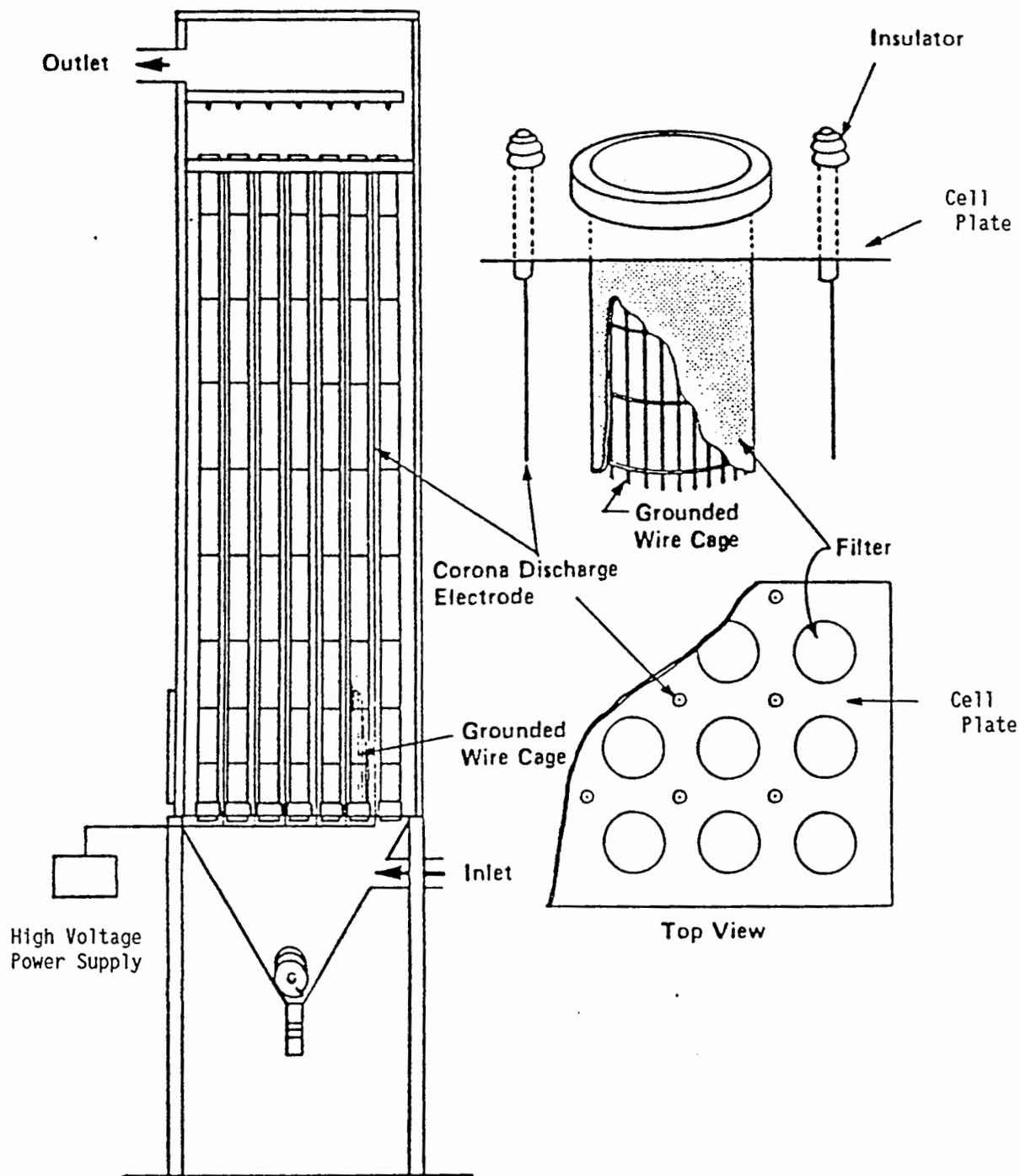
**Figure 6. Electrostatically Augmented Pulse Jet Baghouse**
