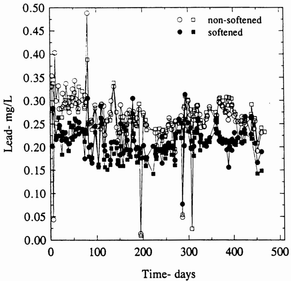
Figure 10. Lead leached from lead-pipe loops.
