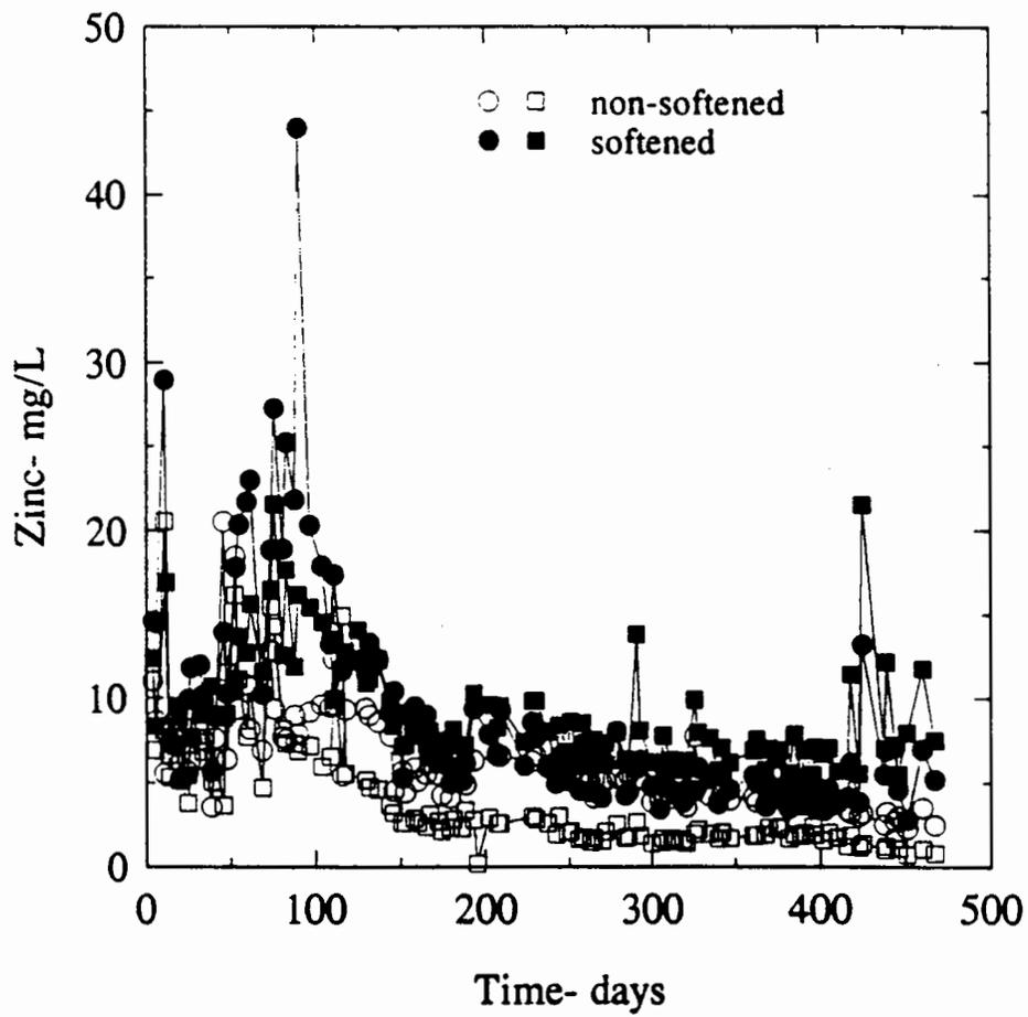
Figure 16. Zinc leached from galvanized pipe loops.
