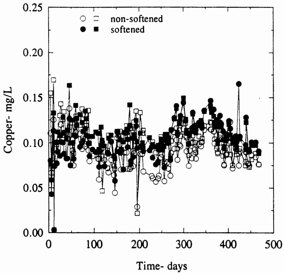
Figure 13. Copper leached from copper tubing loops.
