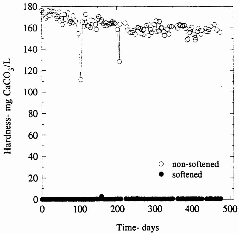
Figure 6. Hardness concentration (as CaCO<sub>3</sub>) of the unsoftened and softened water.
