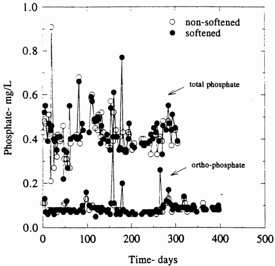
Figure 8. Total and ortho-phosphate concentration of the unsoftened and softened water.
