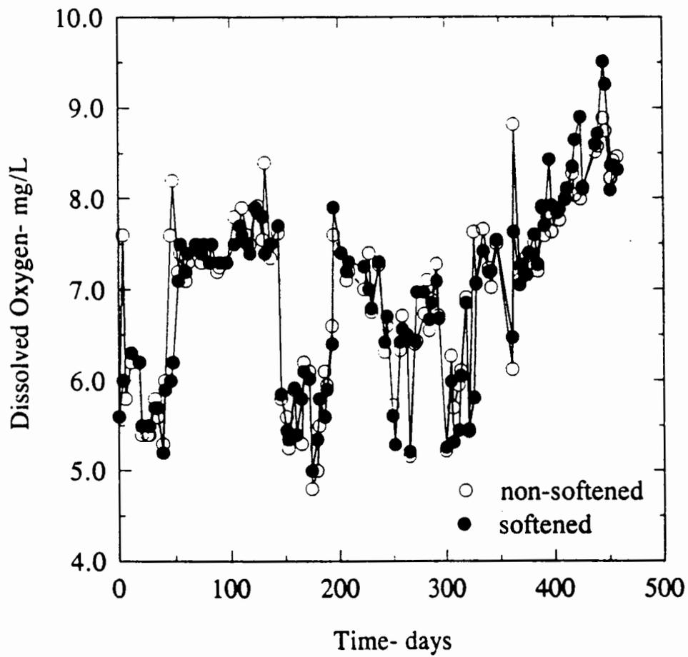
Figure 5. Dissolved oxygen concentration of the unsoftened and softened water.
