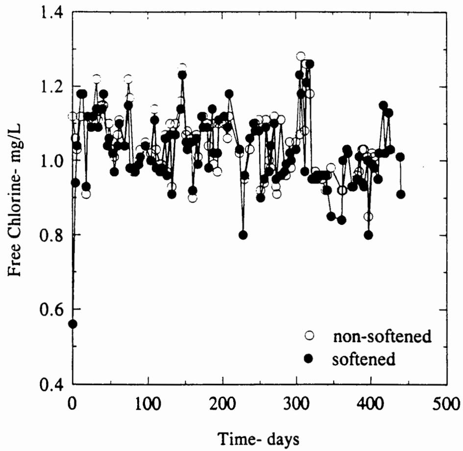
Figure 7. Chlorine (total) concentration of the unsoftened and softened water.
