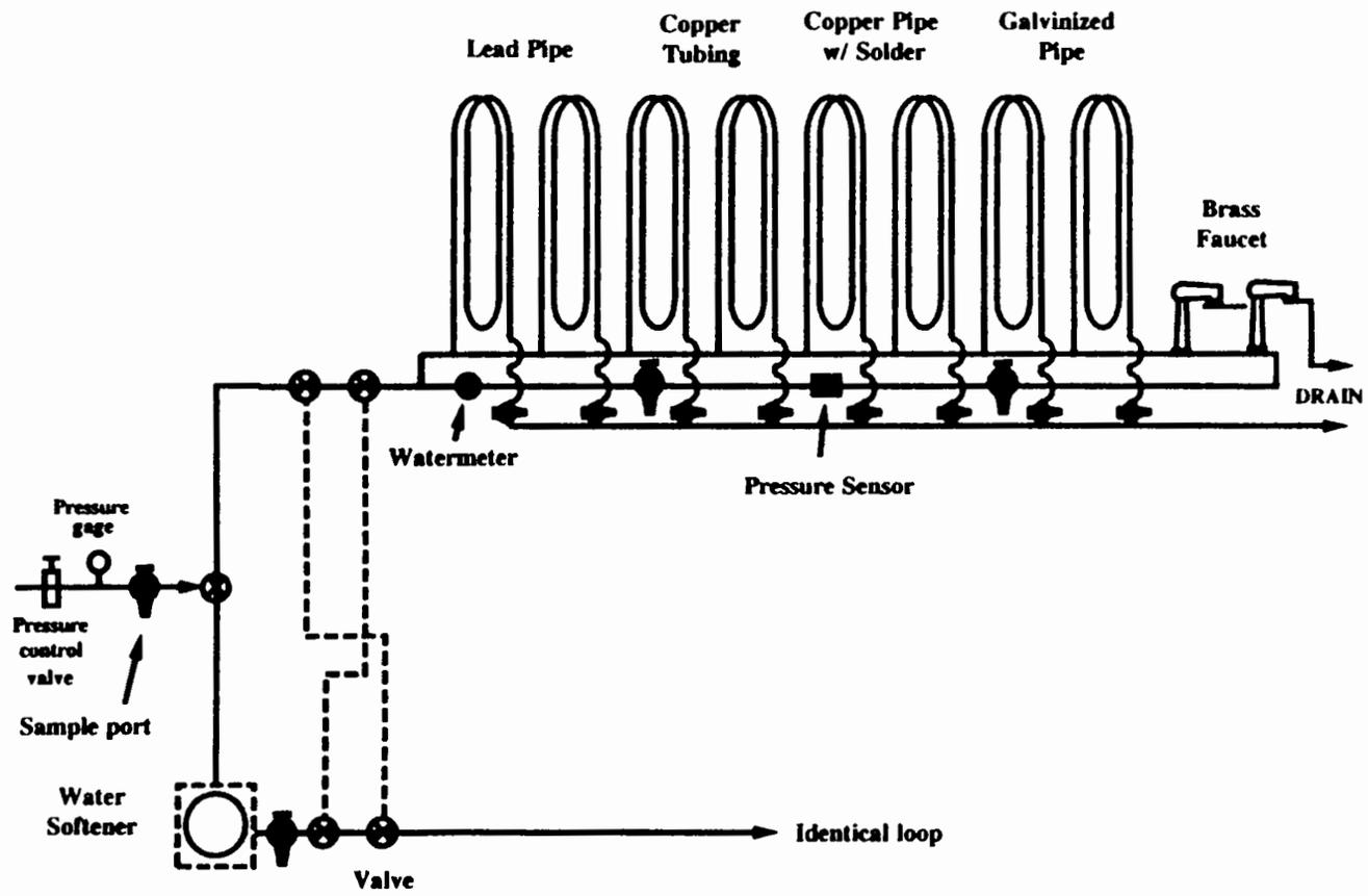
Figure 1. Pipe Loop System.
