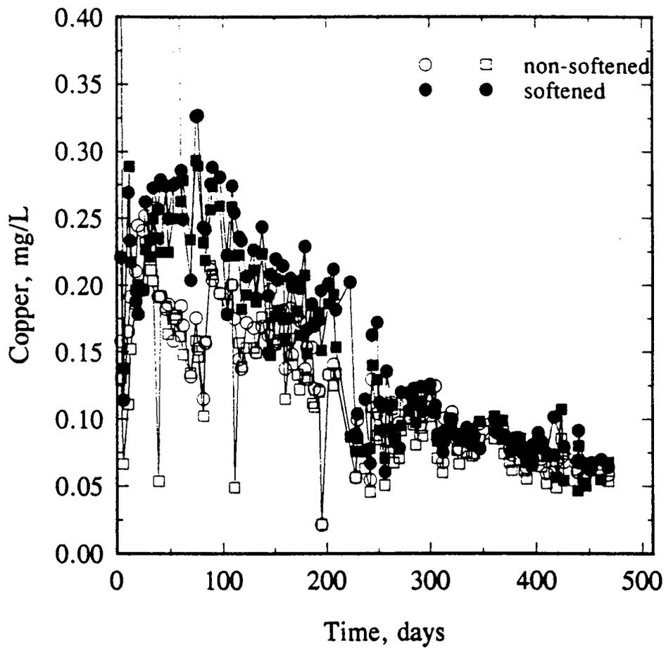
Figure 14. Copper leached from copper/solder pipe loops.
