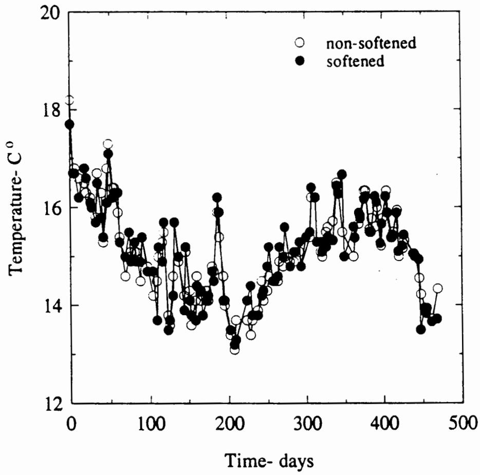
Figure 4. Temperature of the unsoftened and softened water.
