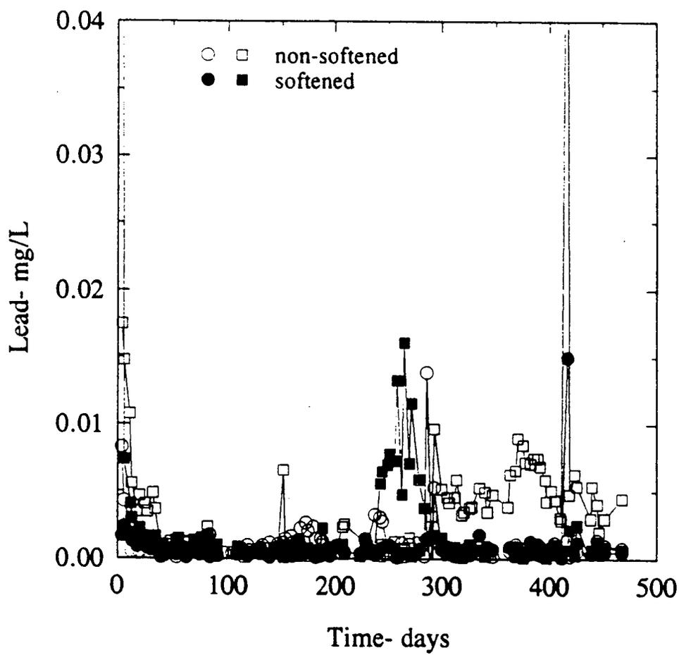
Figure 11. Lead leaching from copper/solder pipe loops.
