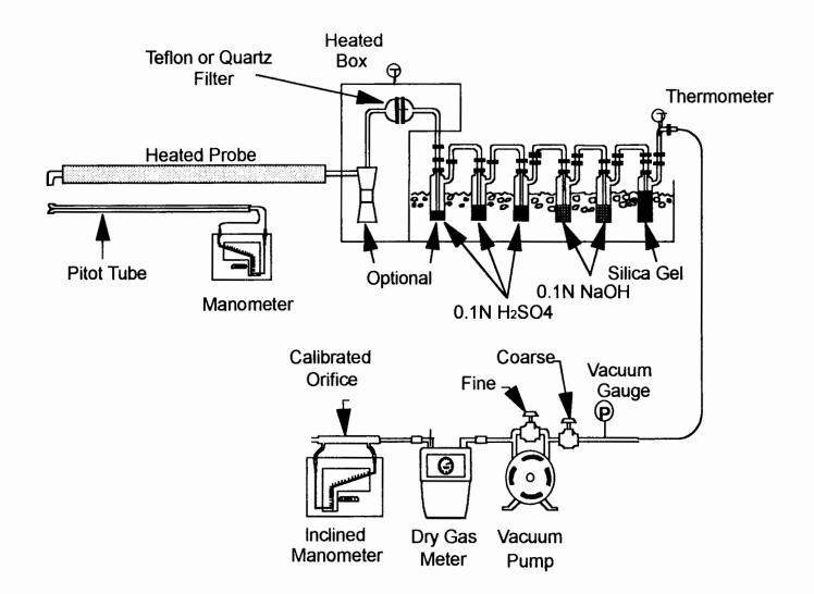
Figure 1. Sampling Train for Methods 0050 and 26A.
