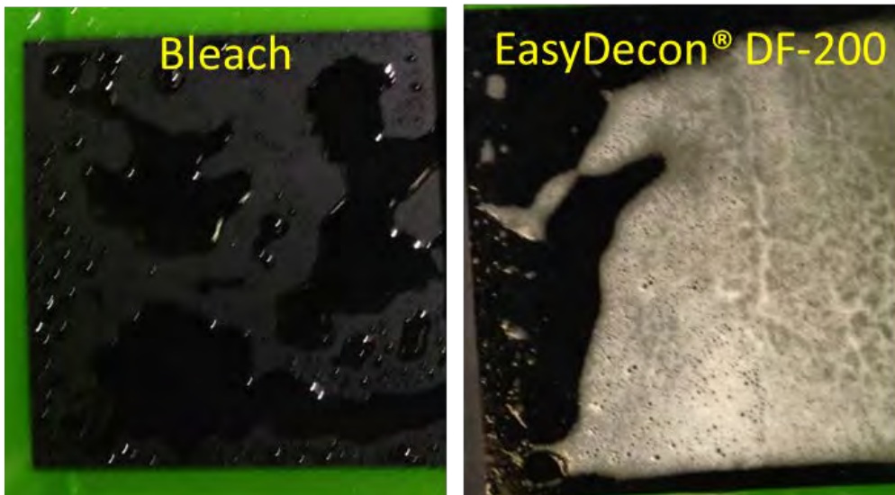
Figure 10: Decontaminant applied to rubber coupon
