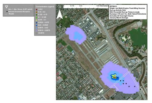
Figure C-5 January-March 3-month average lead air concentrations ( $\mu g/m^3$ ) at the model airport from run-up mode alone using the 95th percentile run-up duration.
