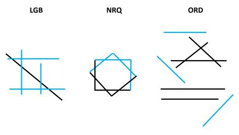
Figure B-10. Multi-runway airports with unique operational profiles. Black lines represent runways not serving piston-engine aircraft and blue lines represent runways serving piston-engine aircraft
