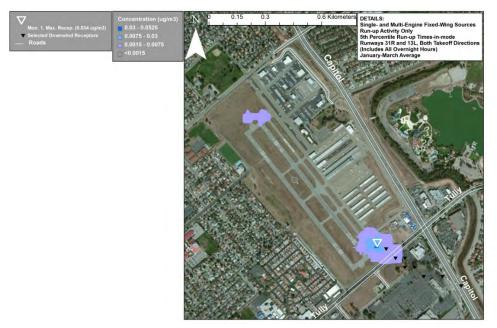
Figure C-3 January-March 3-month average lead air concentrations ( $\mu g/m^3$ ) at the model airport from run-up mode alone using the 5<sup>th</sup> percentile run-up duration.
