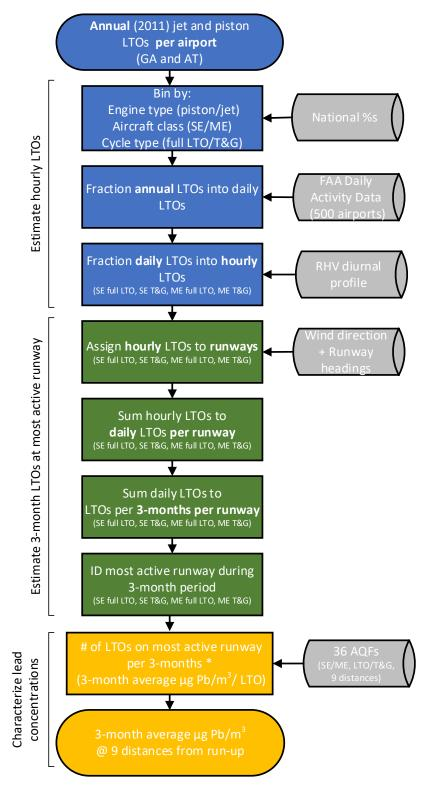
Figure 2. Overview of method to estimate piston-engine aircraft activity at airports nationwide. Center rectangles represent main calculation steps, while colors denote different spatial granularity. Grey cylinders represent input datasets. See Table 2 for details.
