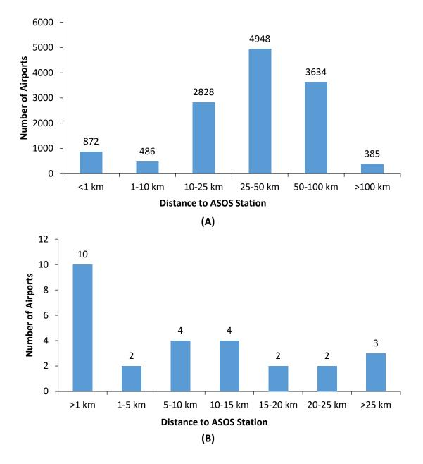
Figure B-11. Distribution of the number of airports by distance to the closest ASOS station for airports in the national analysis (A), and airport-specific activity analysis (B). In both analyses, ASOS stations provided wind direction data that was used to identify the active runway end for piston-engine aircraft. Results from both analyses have greater uncertainty for airports with a longer distance to an ASOS station compared to airports closer to an ASOS station.
