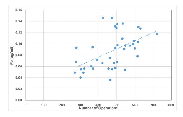
Figure 4. Example of the relationship between monitored lead concentrations and piston-engine aircraft activity.<sup>50</sup>
