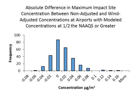
Figure 8. The absolute change in 3-month maximum concentration at the maximum impact site from accounting for average inverse wind speed at airports with concentrations greater than ½ the NAAQS for Lead.
