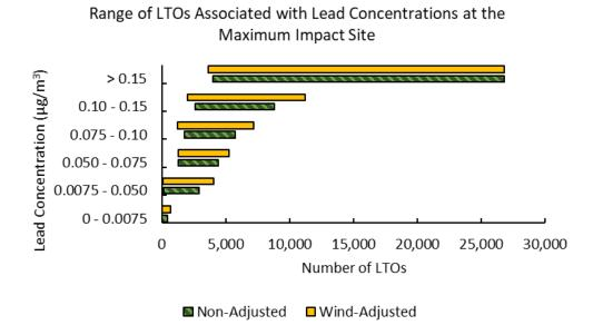
Figure 6. Average 3-month model-extrapolated concentrations versus the number of piston-engine LTOs during the same 3-month period at the maximum impact area runway end. Concentrations are generally categorized relative to the lead NAAQS (e.g., greater than the standard of 0.15  $\mu$ g/m<sup>3</sup>, less than half the standard, 0.075  $\mu$ g/m<sup>3</sup>, less than concentrations generally detected by monitors, 0.0075  $\mu$ g/m<sup>3</sup>, etc).
