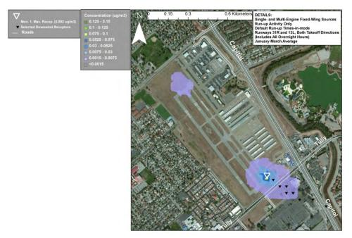
Figure C-4 January-March 3-month average lead air concentrations ( $\mu g/m^3$ ) at the model airport from run-up mode alone using the default run-up duration.
