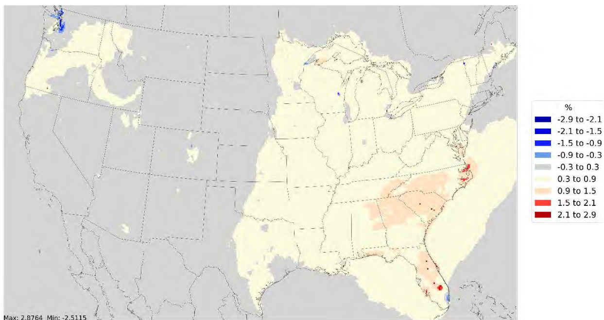
Figure 7.2 Percent change in concentrations of 8-hour maximum average ozone between “pre-RFS” and “with-RFS” scenarios
