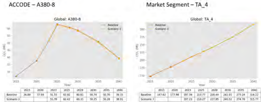
Figure 5-10 – CO 2 emissions of A380-8 and market segment TA_4 for the baseline and Scenario 3
