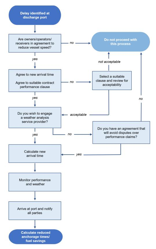
Figure 1. Virtual Vessel Arrival Process
