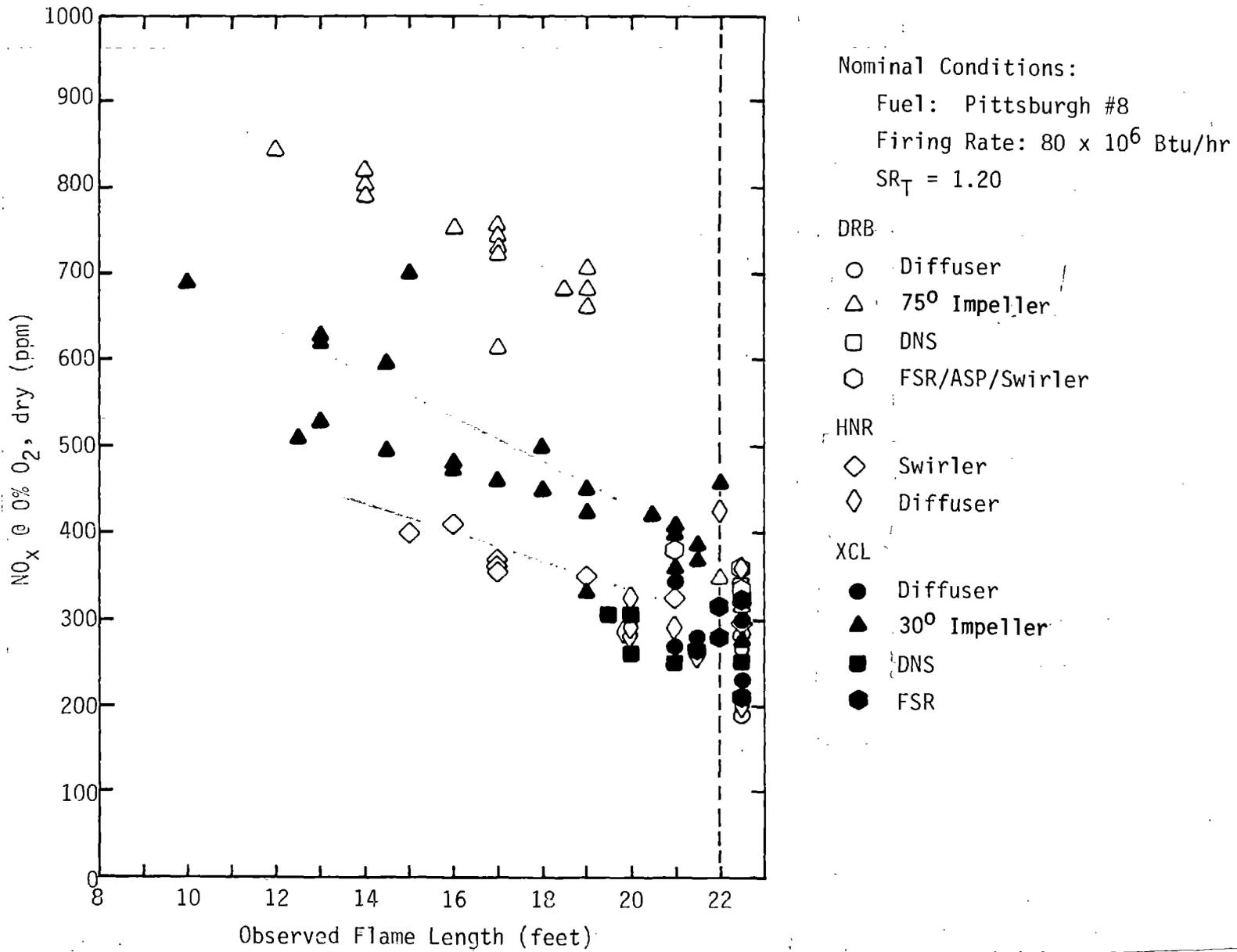
Figure 4-32. Correlation of  $NO_x$  emissions with flame length.
