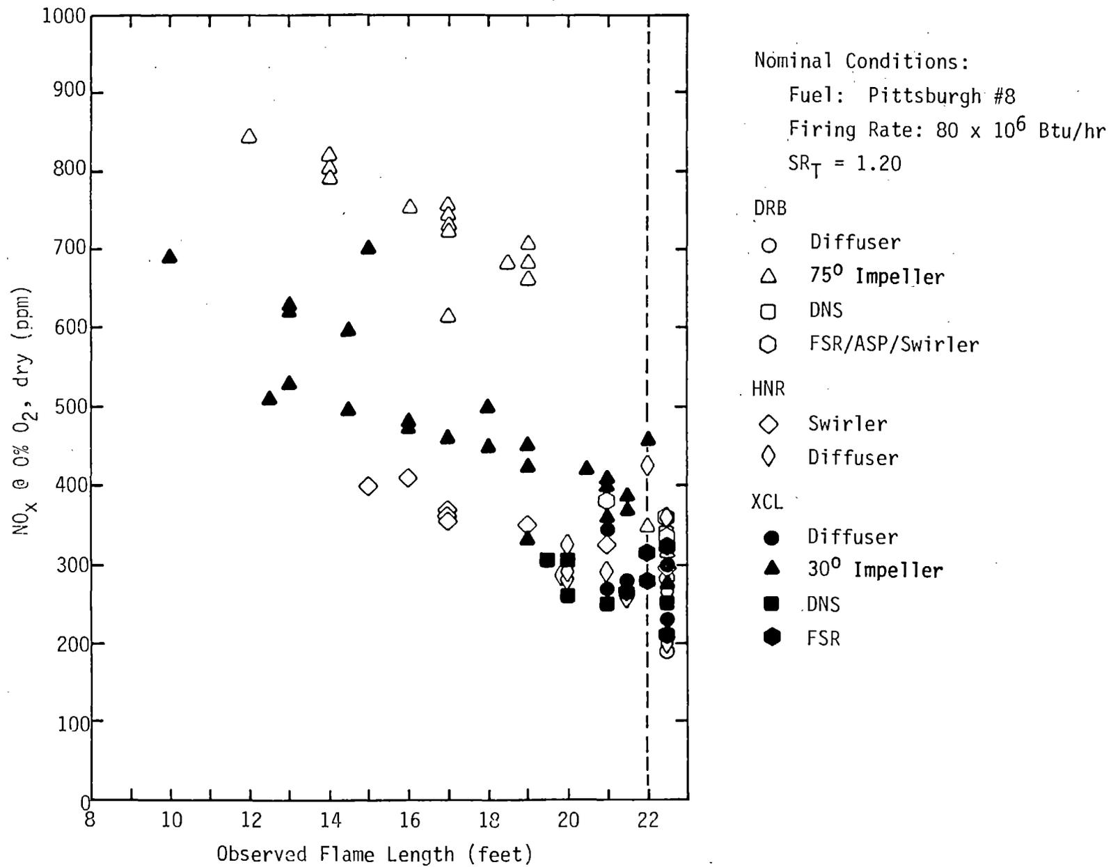
Figure 1-1. Correlation of NO<sub>x</sub> emissions with flame length.
