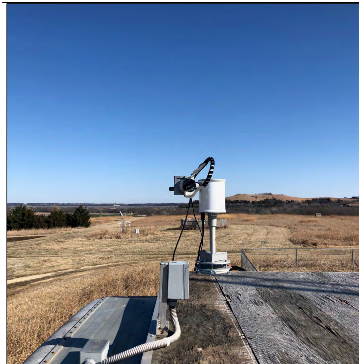
Figure 15. The Pandora spectrometer located at Konza Prairie.
