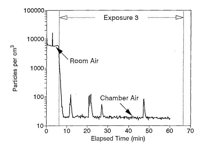
Figure 3-9. Particle counting data for Sample A in Test 1.
