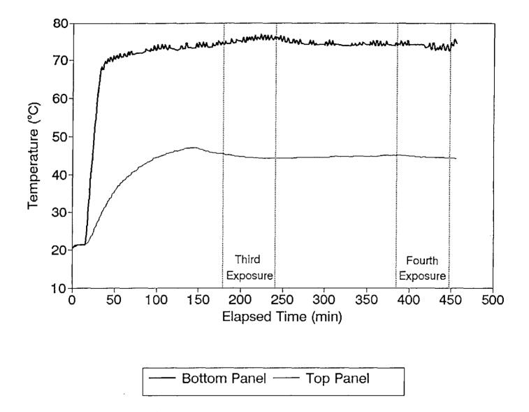
Figure 3-6. Temperature profiles for Test 4; Chamber panel temperature on Day 2.
