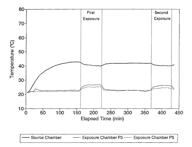
Figure 3-1. Temperature profiles for Test 4; Air temperature on Day 1.
