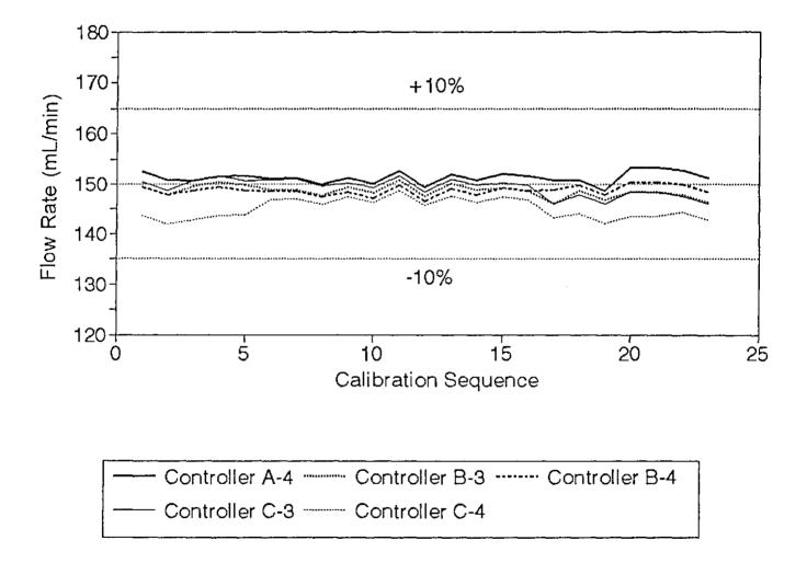
Figure 4-4. Calibration of mass flow controllers (1) Flow rate = 150 mL/min.
