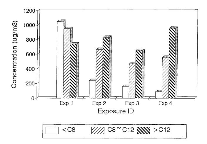
Figure 5-3. The change of TVOC composition during exposure; Sample A, Test 1.
