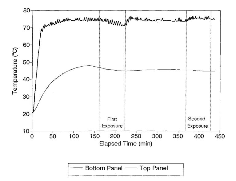
Figure 3-5. Temperature profiles for Test 4; Chamber panel temperature on Day 1.
