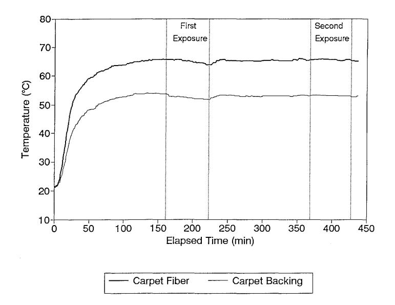
Figure 3-3. Temperature profiles for Test 4; Sample surface temperature on Day 1.
