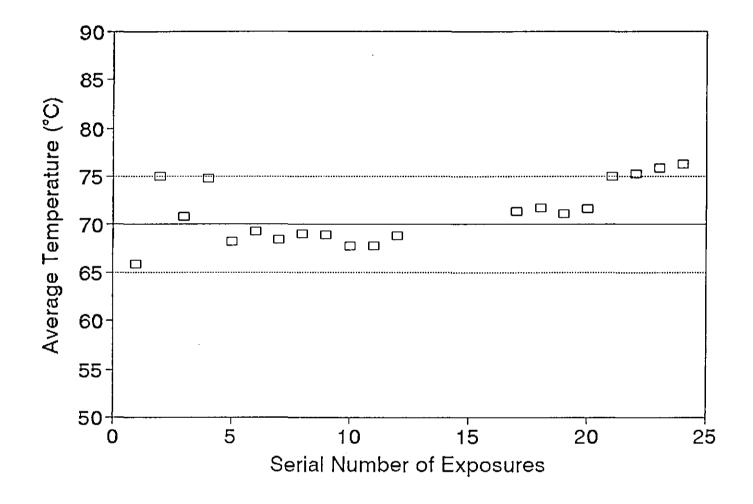
Figure 4-1. Results of temperature control; Chamber bottom panel.
