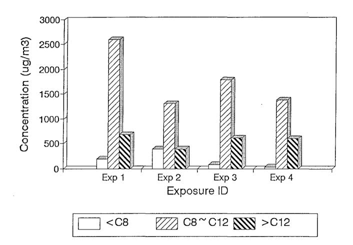
Figure 5-8. The change of TVOC composition during exposures; Sample C, Test 5.
