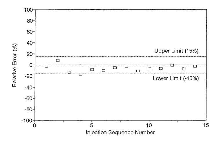
Figure 4-8. GC daily QC check results (2) Envirochem II/Liquid Tolucne standard.
