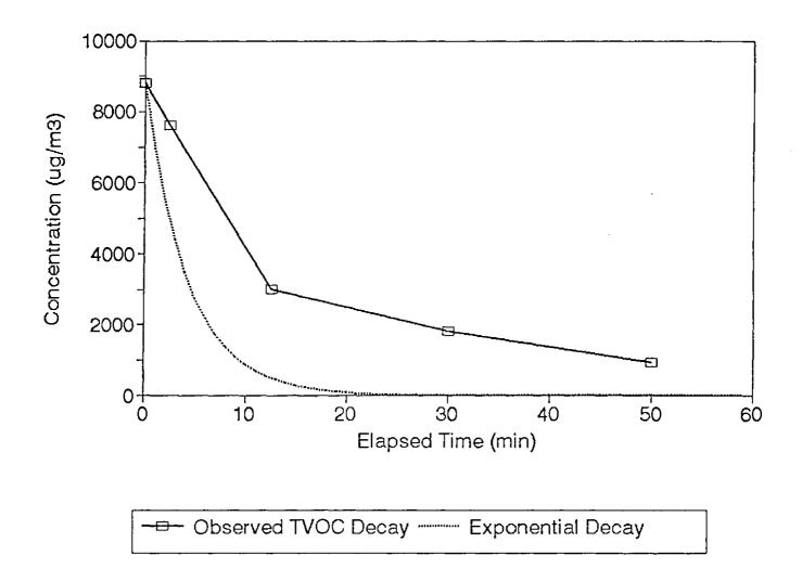
Figure 3-8. Observed TVOC concentrations vs. exponential decay (Exposure 1, Test 1).
