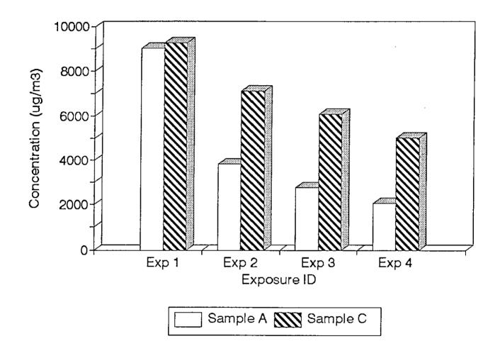
Figure 5-1. Initial TVOC concentrations in the source chamber.
