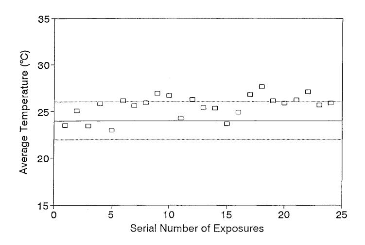
Figure 4-3. Results of temperature control; Air in the exposure chamber.
