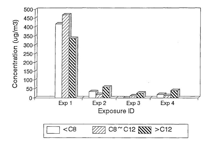
Figure 5-6. The change of TVOC composition during exposures; Sample B, Test 3.
