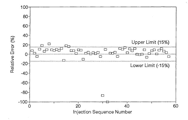
Figure 4-7. GC daily QC check results (1) Envirochem I/Liquid Toluene standard.
