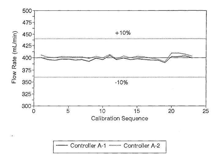
Figure 4-5. Calibration of mass flow controllers (2) Flow rate = 400 mL/min.
