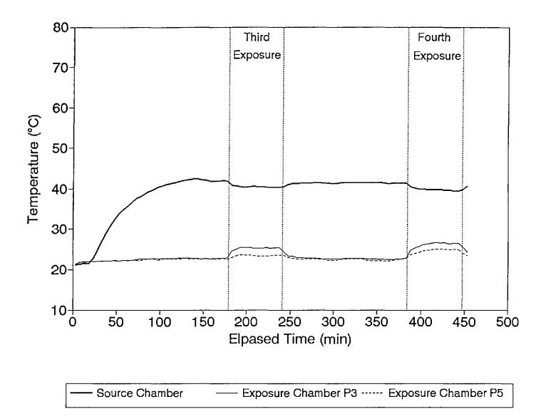
Figure 3-2. Temperature profiles for Test 4; Air temperature on Day 2.
