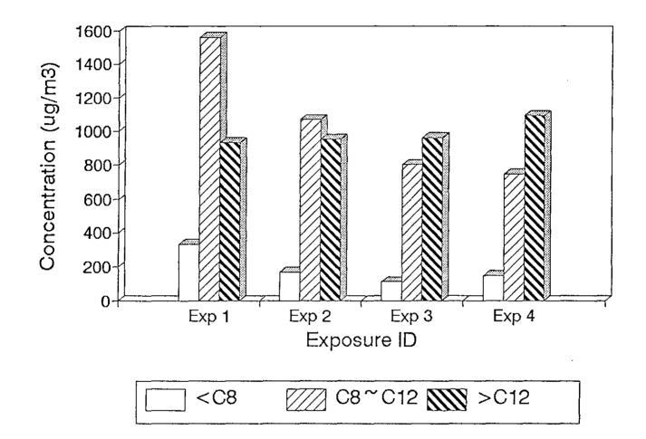
Figure 5-4. The change of TVOC composition during exposures; Sample A, Test 6.
