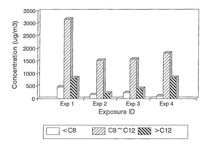
Figure 5-7. The change of TVOC composition during exposures; Sample C, Test 4.
