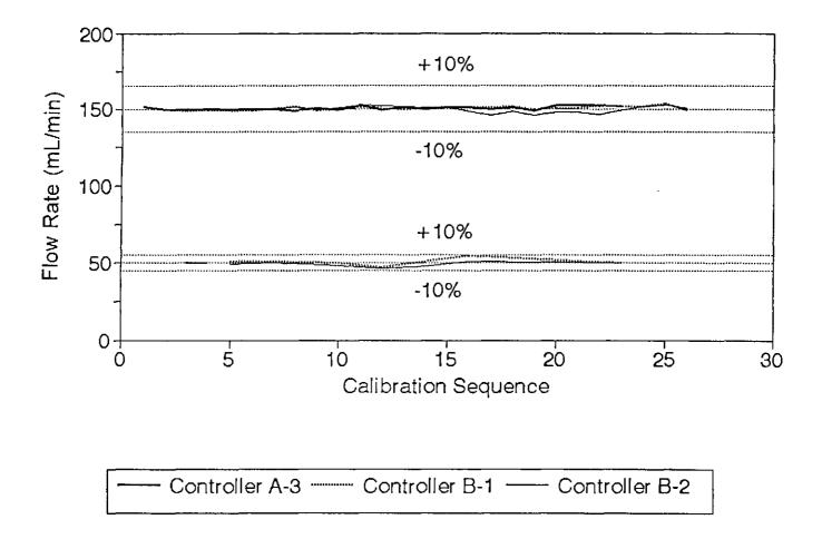
Figure 4-6. Calibration of mass flow controllers (3) Used at two flow rates.
