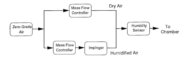
Figure 2-3. The air humidifying system.
