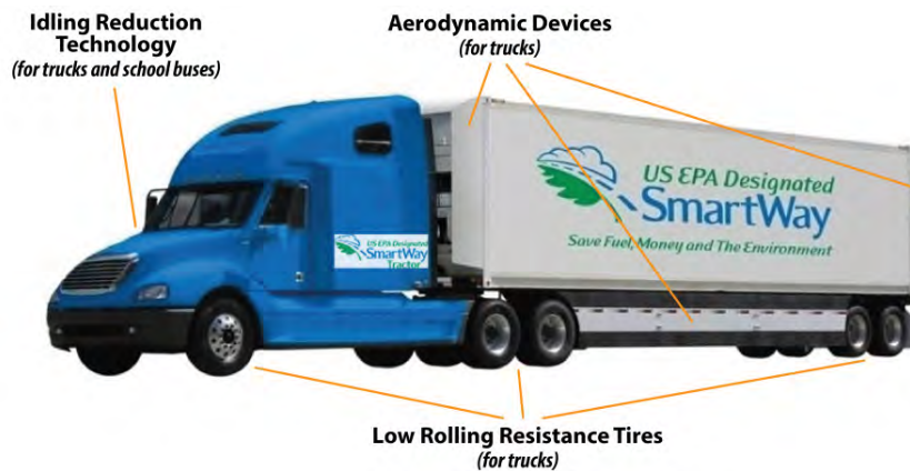
A trailer equipped with side skirts, gap fairings, and a rearboat tail
