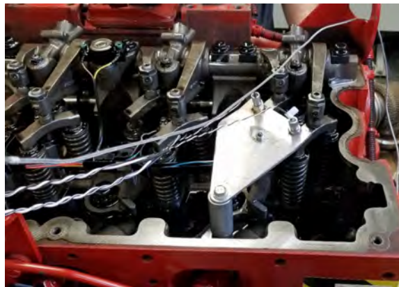
Figure 3-14: Variable reluctance sensor for valve position measurement. The final installation will include valve position measurement at the valve bridges for each of the six cylinders.
