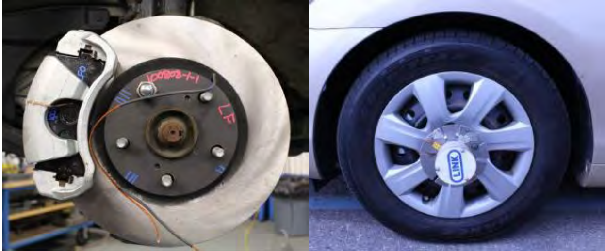
Figure 4. Brake Thermocouples and wireless hub transmitter installed on the Camry test vehicle
