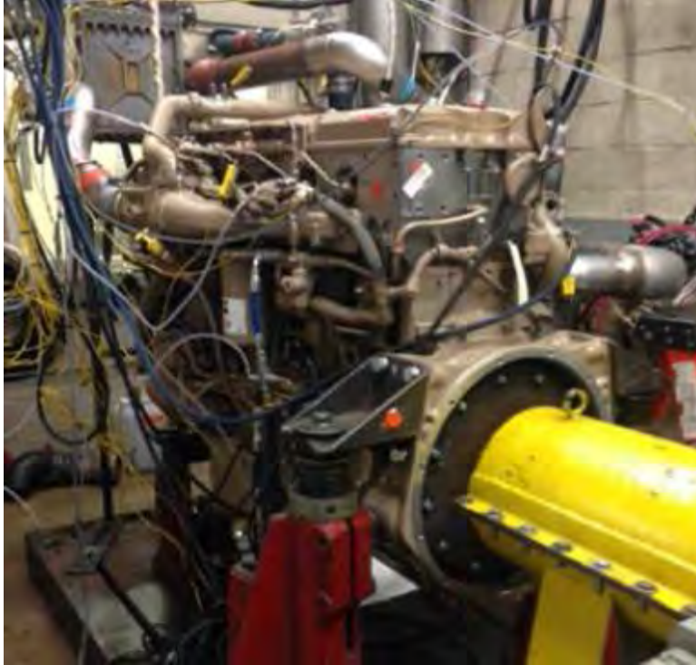
Figure 3-1: Developmental Cummins X15 Engine equipped with individual cylinder deactivation undergoing engine dynamometer testing as part of the CARB Stage 3 research at SwRI.
