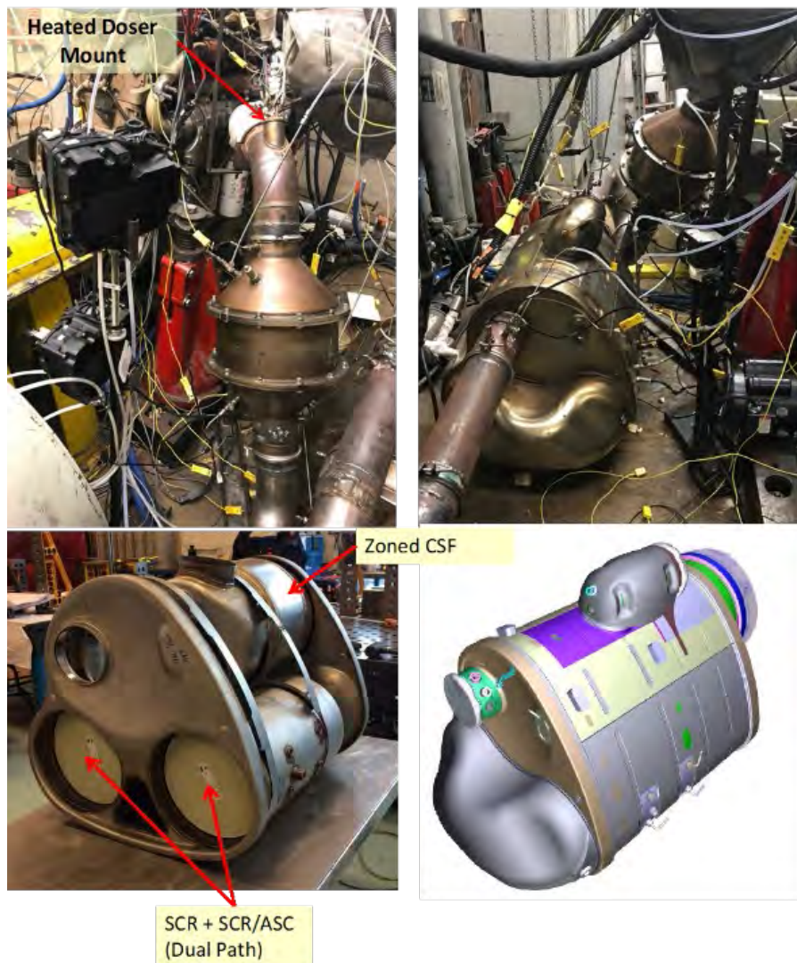
Figure 3-3: Developmental EAS with light-off SCR installed in engine dynamometer test cell at SwRI (upper left, upper right) and details of the downstream, single "box" unit (lower left, lower right).
