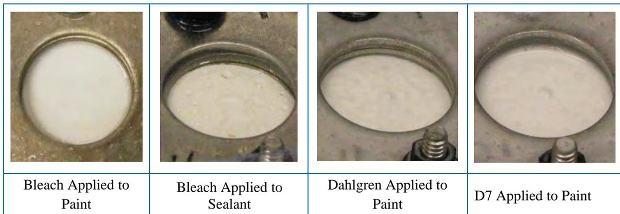
**Figure 19. Decontaminant Observations when Applied to Film Coupons**
