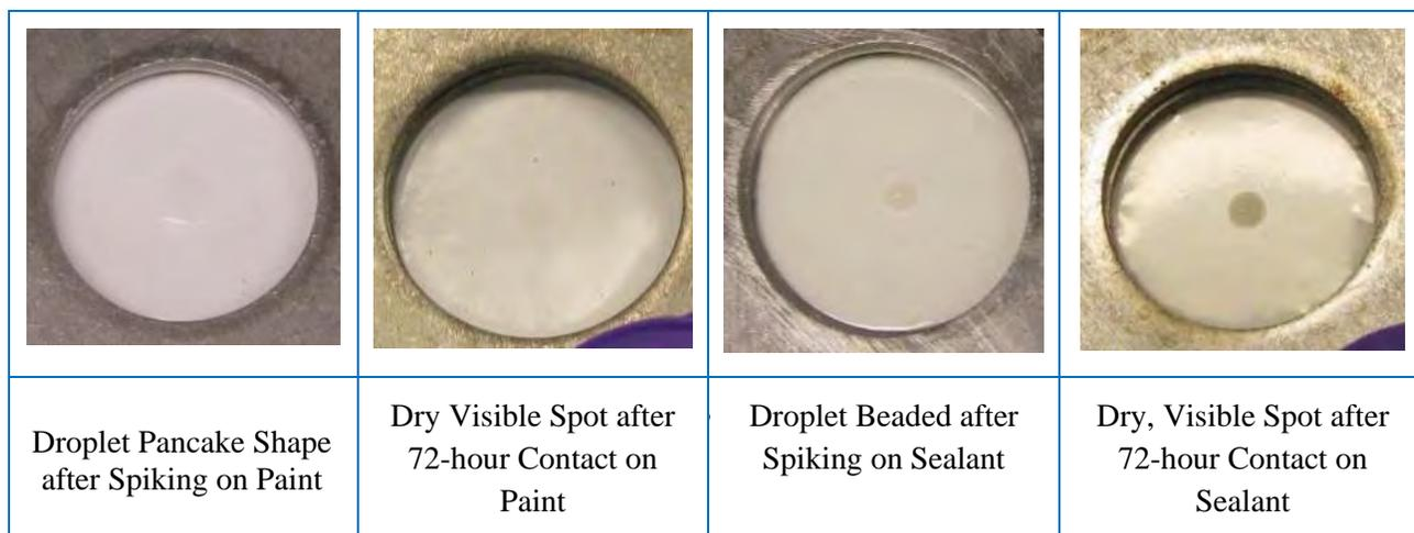
**Figure 16. Fipronil Interactions on Paint and Sealant Films**
