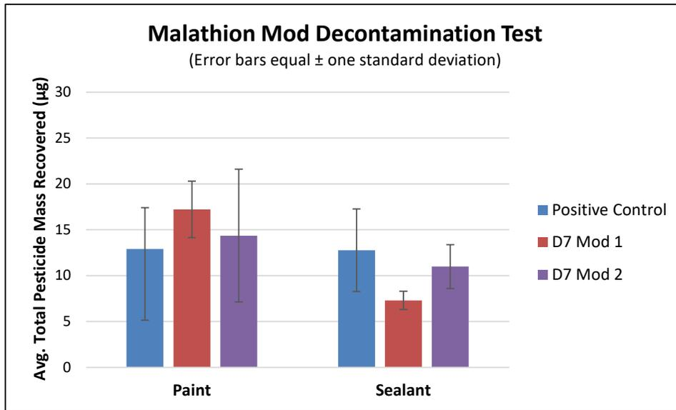
**Figure 38. Malathion Modification Decontaminant Test, Average Total Mass Recoveries**
