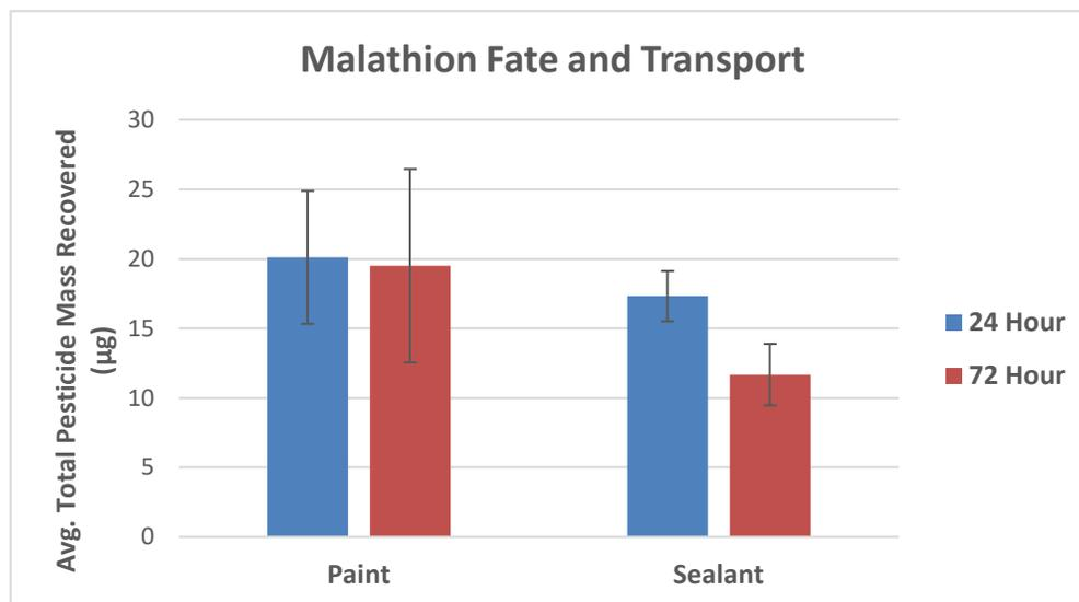
**Figure 17. Total Recovered Malathion for Fate and Transport Testing**
