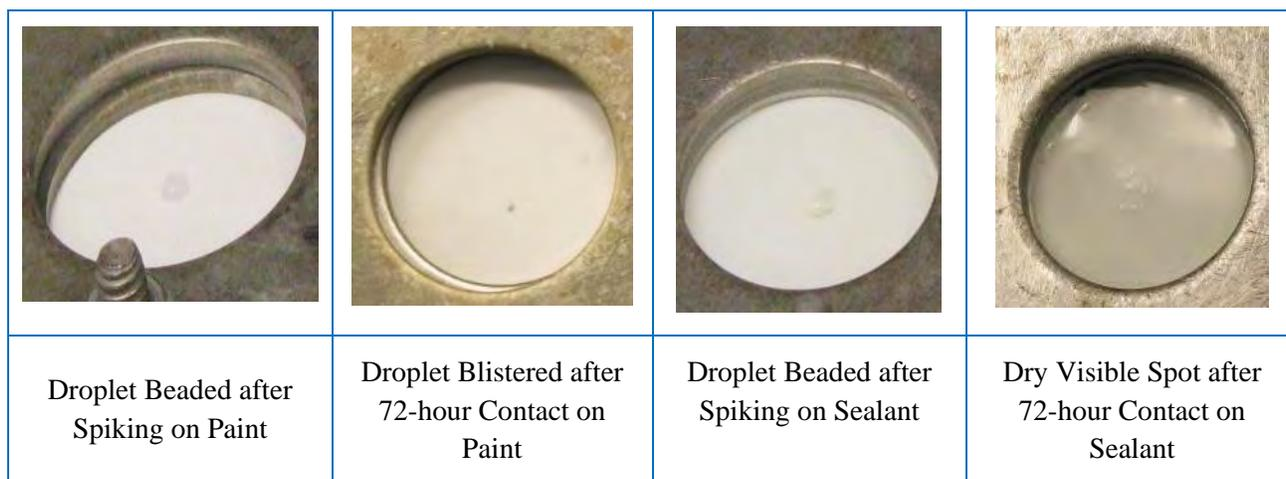
**Figure 15. Malathion Interactions on Paint and Sealant Film Coupons**
