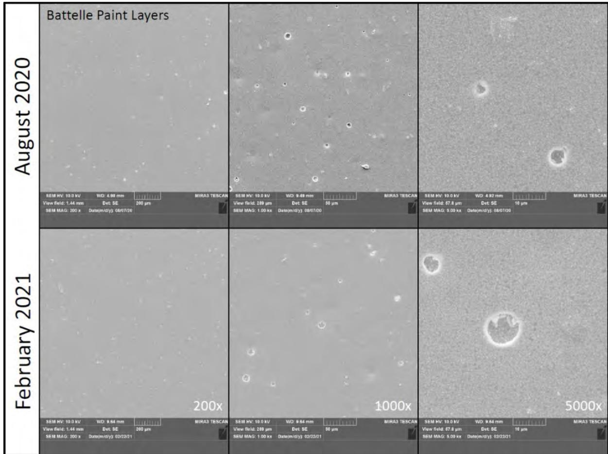
*Figure 3. SEM Image of Paint Films at Increased Magnifications (left to right).*
