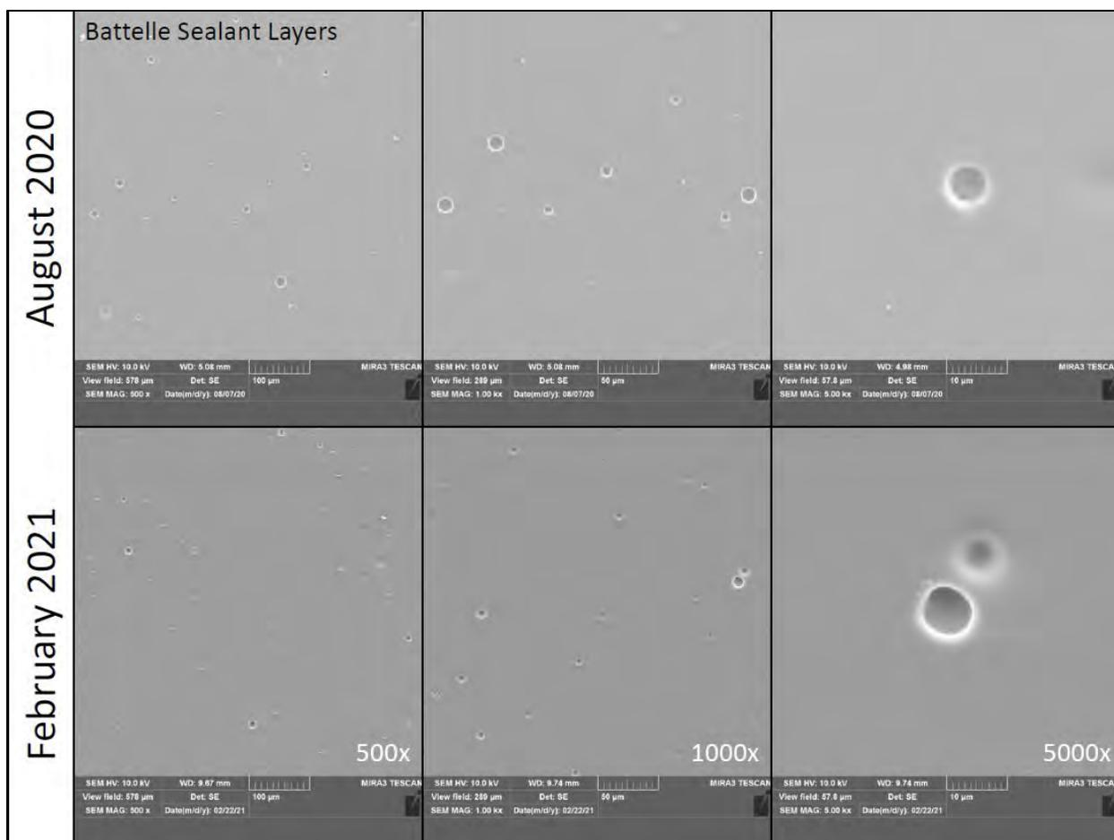
**Figure 4. SEM Image of Sealant Films at Increased Magnifications (left to right).**
