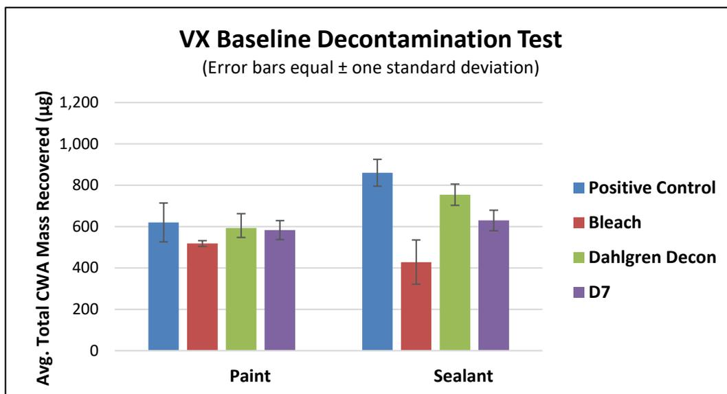
**Figure 24. VX Baseline Decontaminant Test, Average Total Mass Recoveries**
