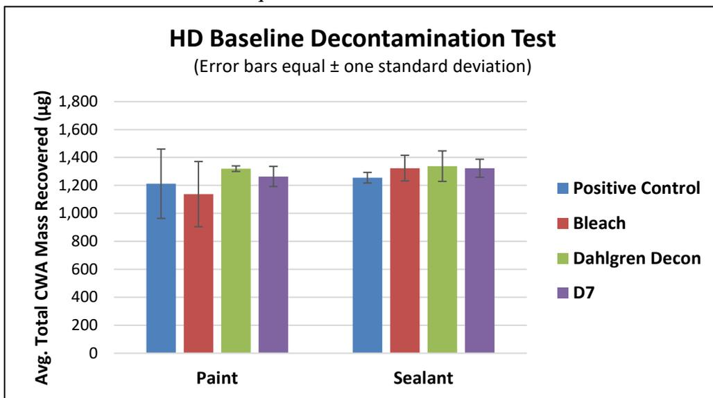
**Figure 23. HD Baseline Decontaminant Test, Average Total Mass Recoveries**
