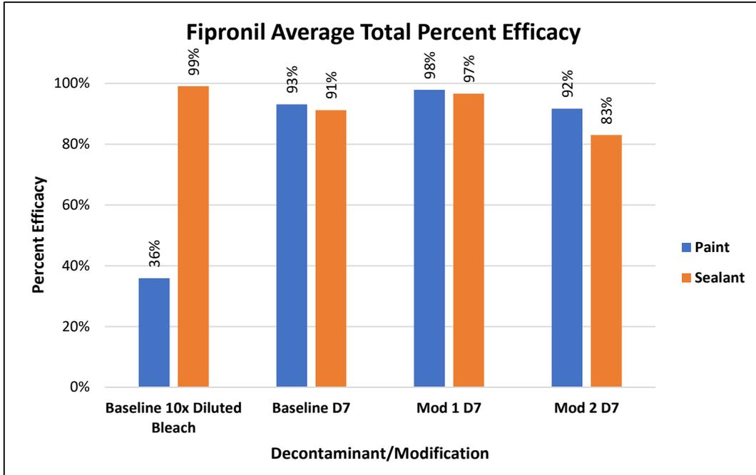
***Figure E 4. Average Total Decontamination Efficacy for Fipronil***
