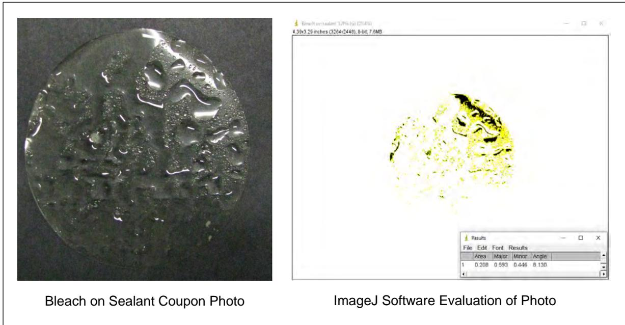
**Figure 6. Example of the Photo Contrast Evaluation of Bleach on Sealant**
