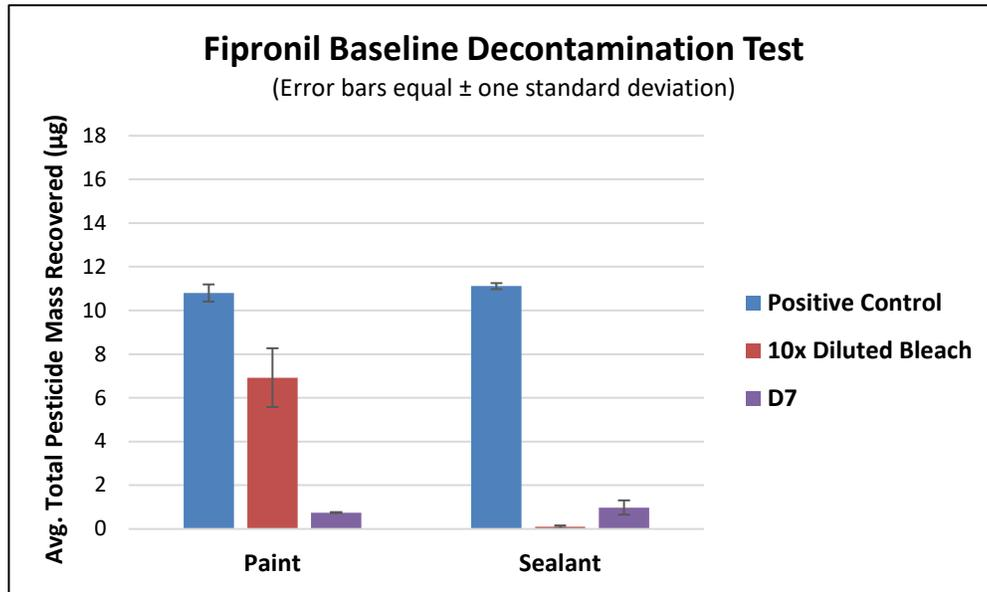
**Figure 26. Fipronil Baseline Decontaminant Test, Average Total Mass Recoveries**
