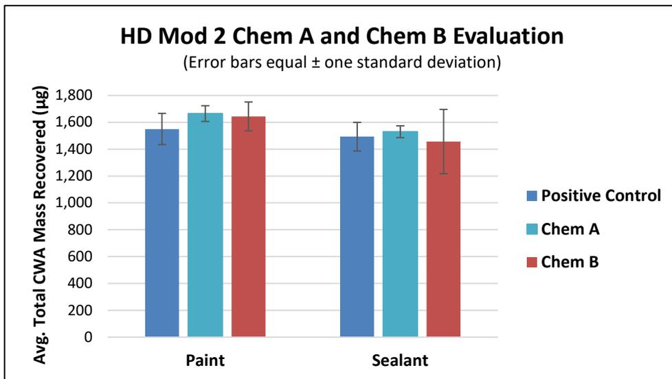
Figure 29. HD Mod 2 Chem A and Chem B Evaluation, Average Total Mass Recoveries
