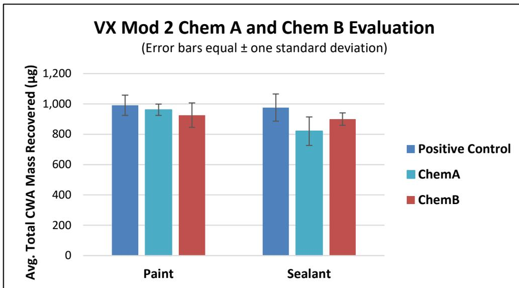
Figure 34. VX Mod 2 Chem A and Chem B Evaluation, Average Total Mass Recoveries
