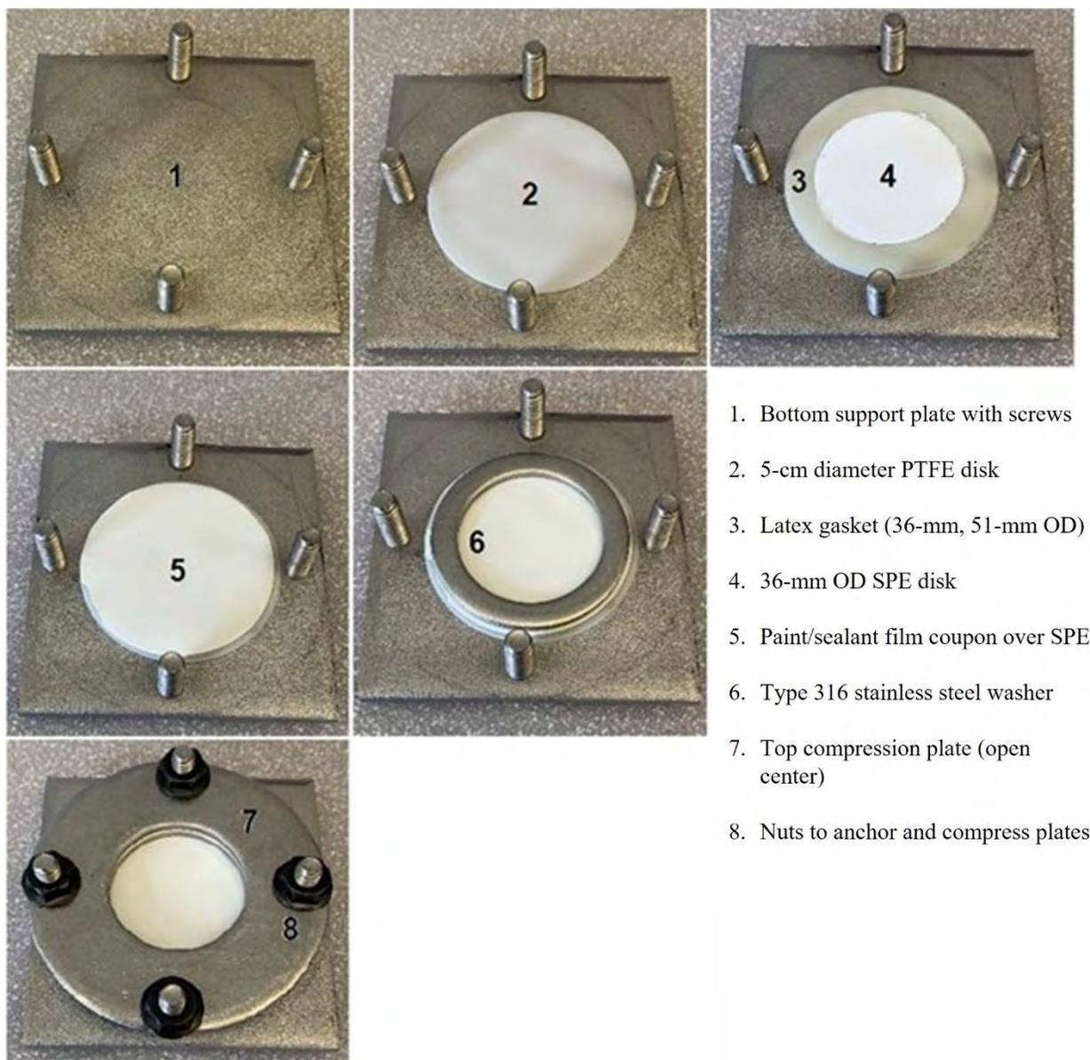
**Figure 5. Paint Film Built into LVAP Assembly**
