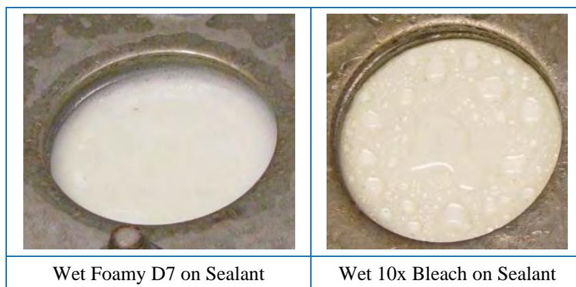
**Figure 21. Sealant Film Coupon Decontaminant Observations after Dwell Time**
