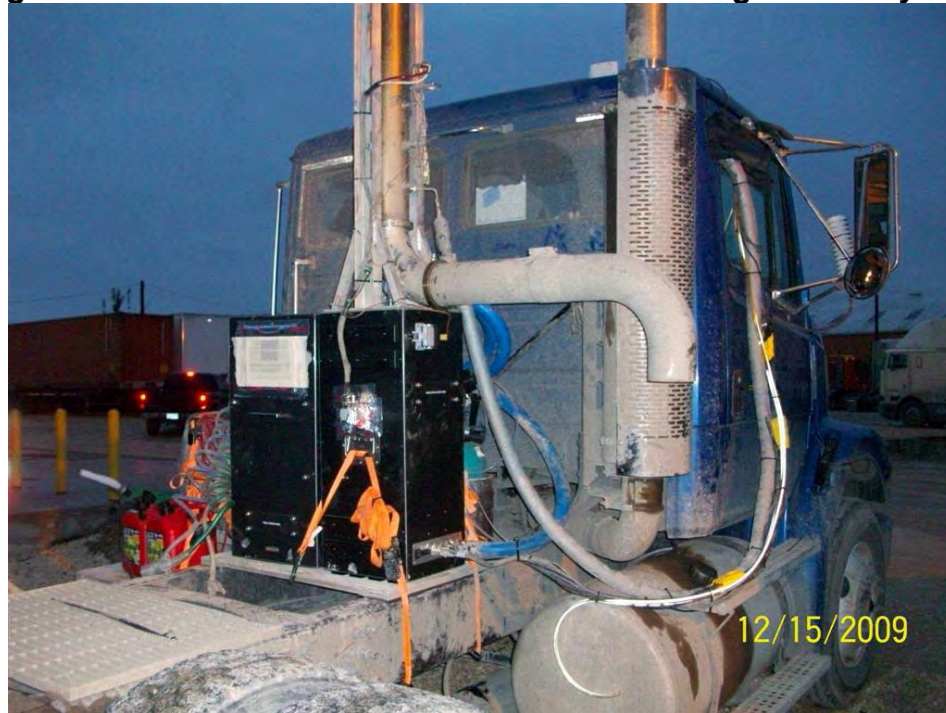
Figure 5.1-5 Grav and MPS Box Outside 1993 Freightliner Day Cab
