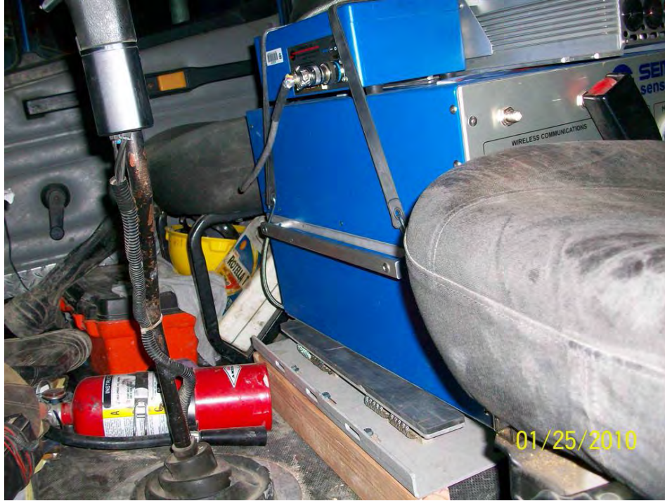
Figure 5.1-19 PEMS Mounting Platform in Day Cab
