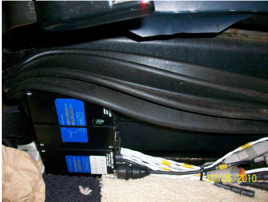
Figure 5.2-2 PAMS Installed on a Seat Base
