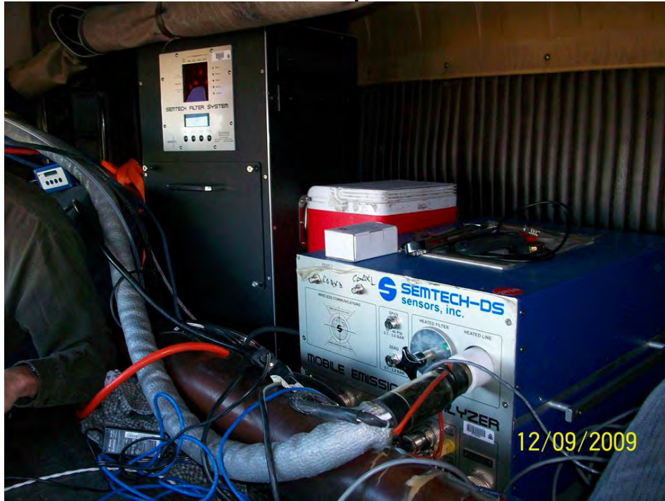
Figure 5.1-9 PEMS and Gravimetric Sampler in 1980 Kenworth Cabover
