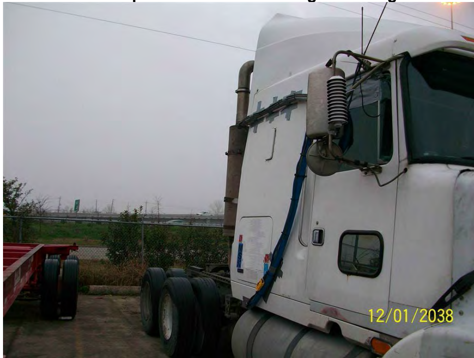
Figure 5.1-17 Sample Lines Routed through Passenger Window
