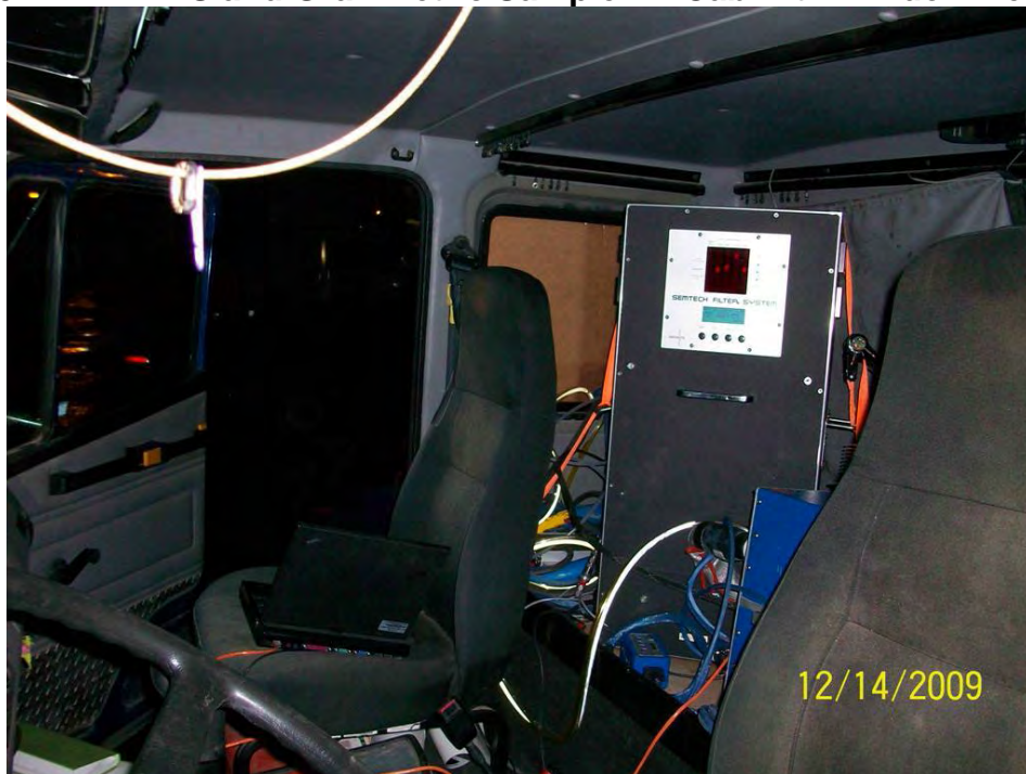
Figure 5.1-10 PEMS and Gravimetric Sampler in Cab with Window Removed
