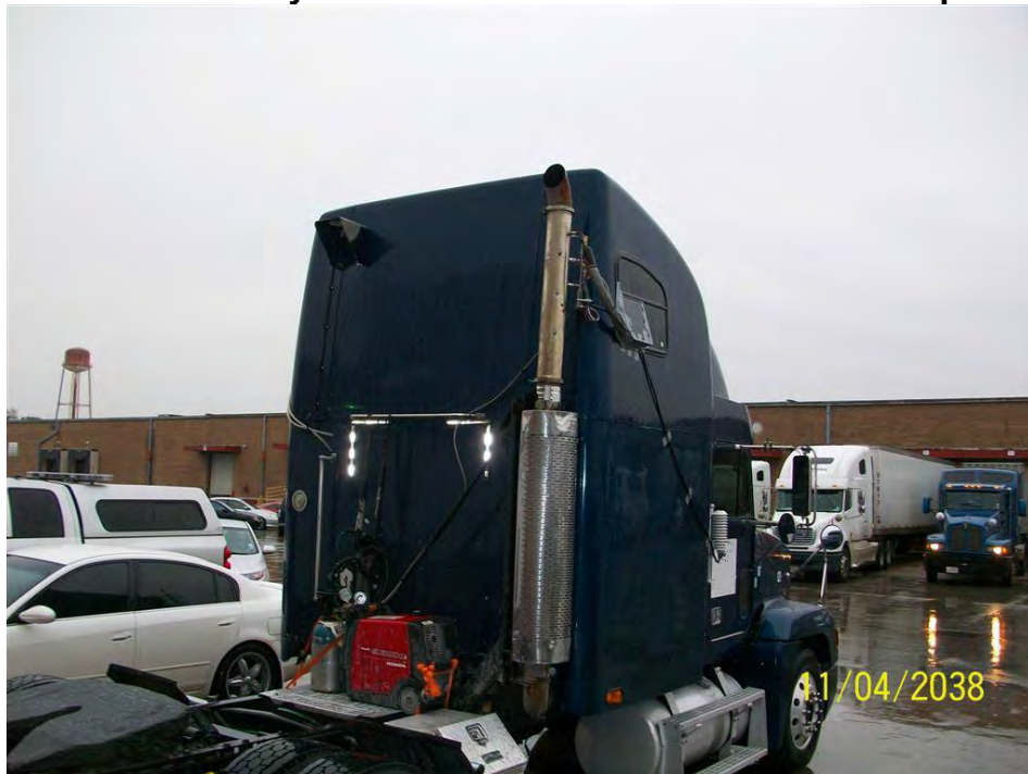
Figure 5.1-7 Gaseous-only Installation on 1998 International Sleeper Cab
