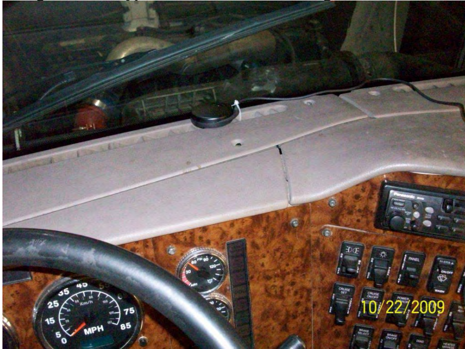
Figure 5.2-3 Typical PAMS GPS Mounting Location
