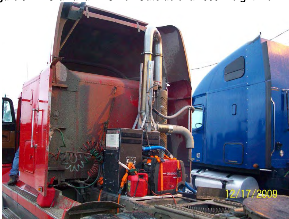
Figure 5.1-4 Grav and MPS Box Outside of a 1993 Freightliner
