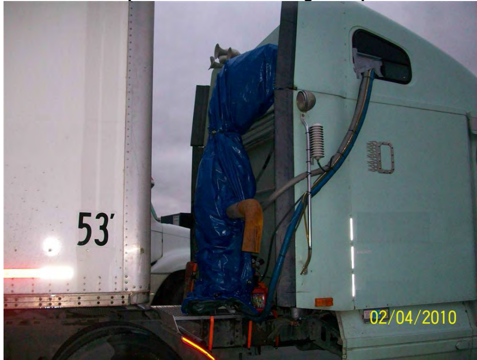
Figure 5.1-14 Sample Lines Routed through Sleeper Cab Window
