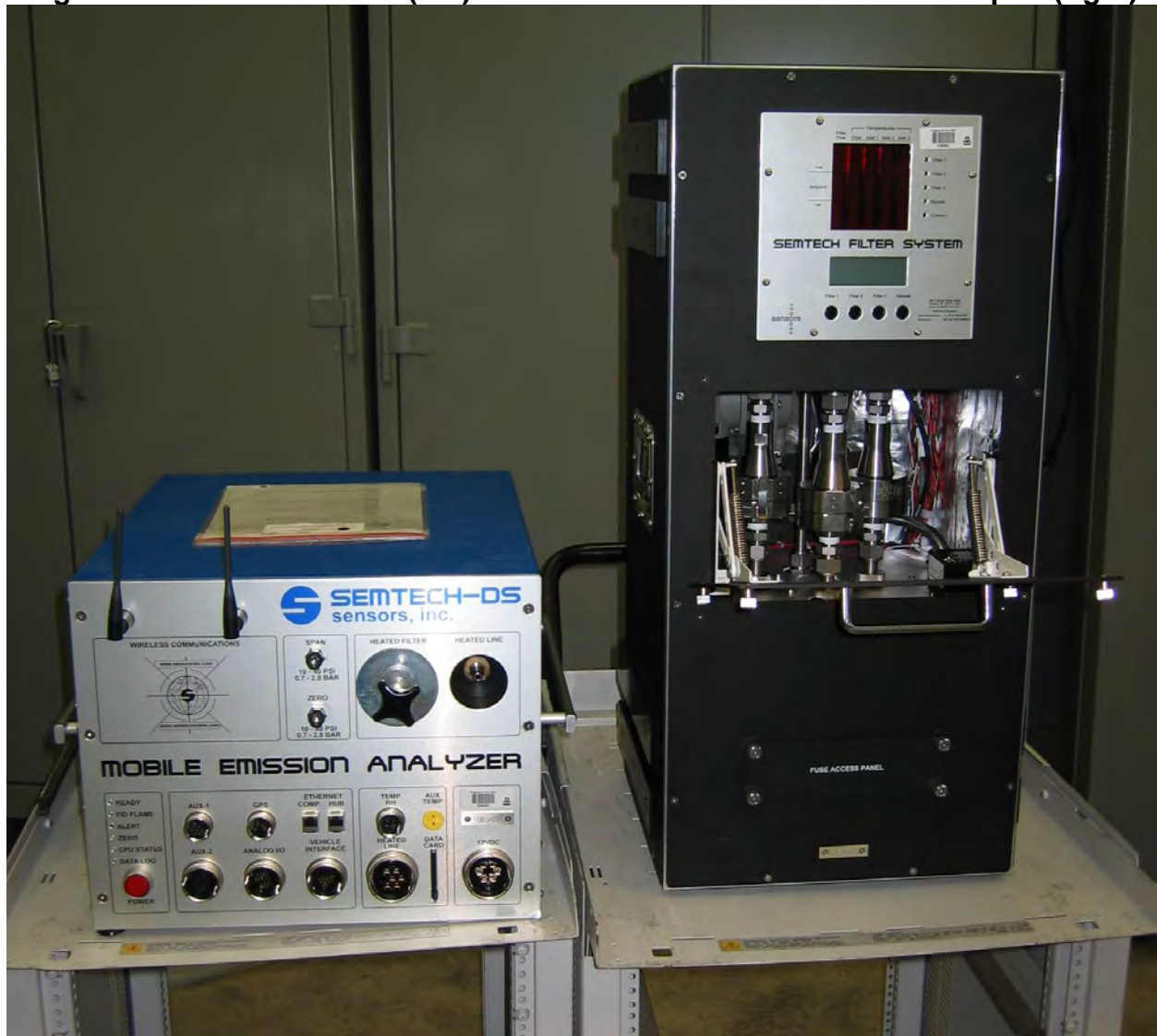
Figure 4.1-1 SEMTECH-DS (left) and 3-Chamber Gravimetric PM Sampler (right)
