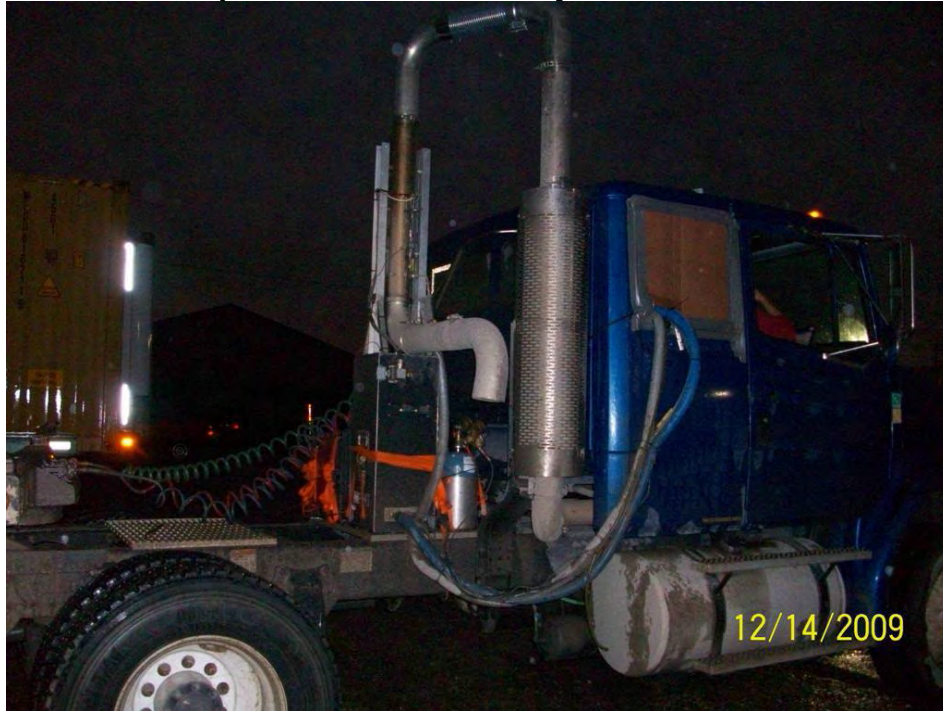
Figure 5.1-11 Sleeper Cab with full PM System and Window Removed
