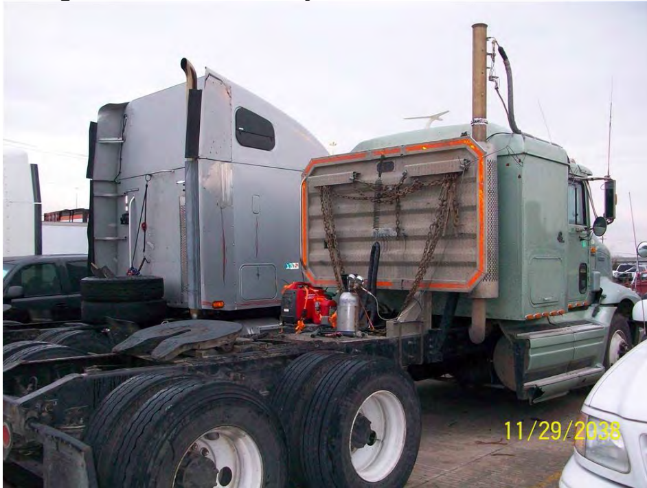
Figure 5.1-1 Gaseous-only Installation on Truck with Bulkhead
