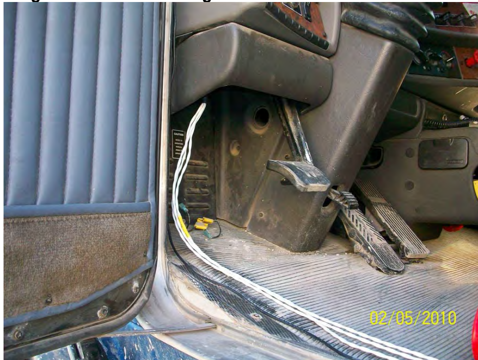
Figure 5.2-4 PAMS wiring from a Deutsch Connector
