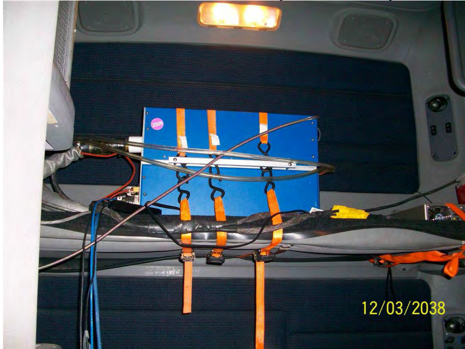
Figure 5.1-12 PEMS installed on Top Bunk of Sleeper Cab
