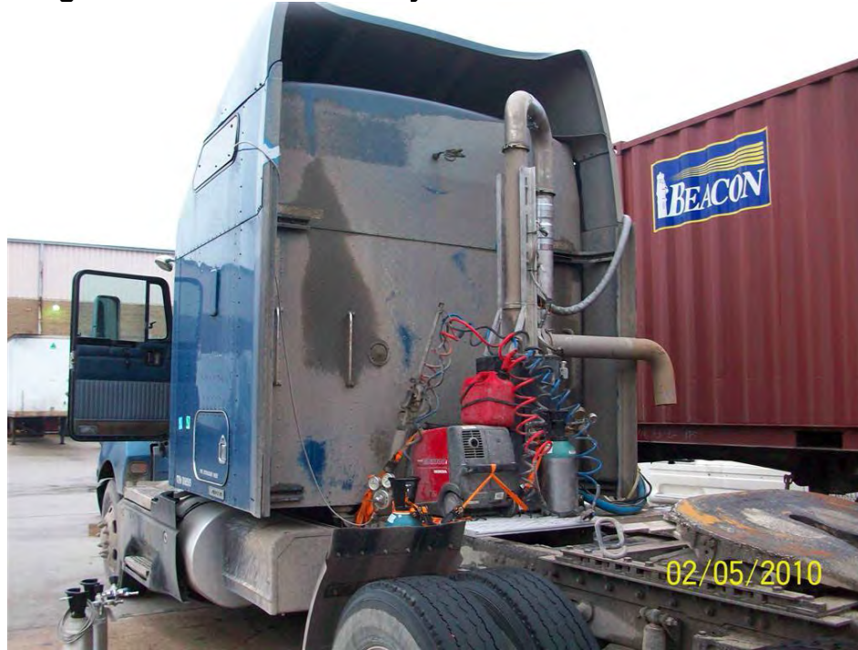
Figure 5.1-3 PM/Gaseous System on 2004 Kenworth
