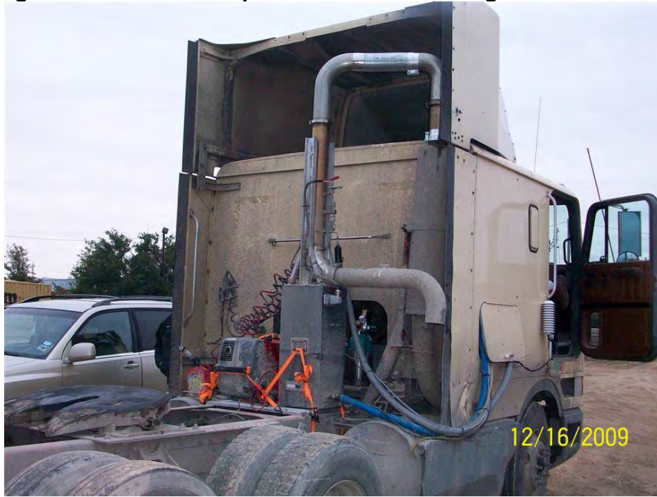
Figure 5.1-16 Sample Lines Routed through Toolbox
