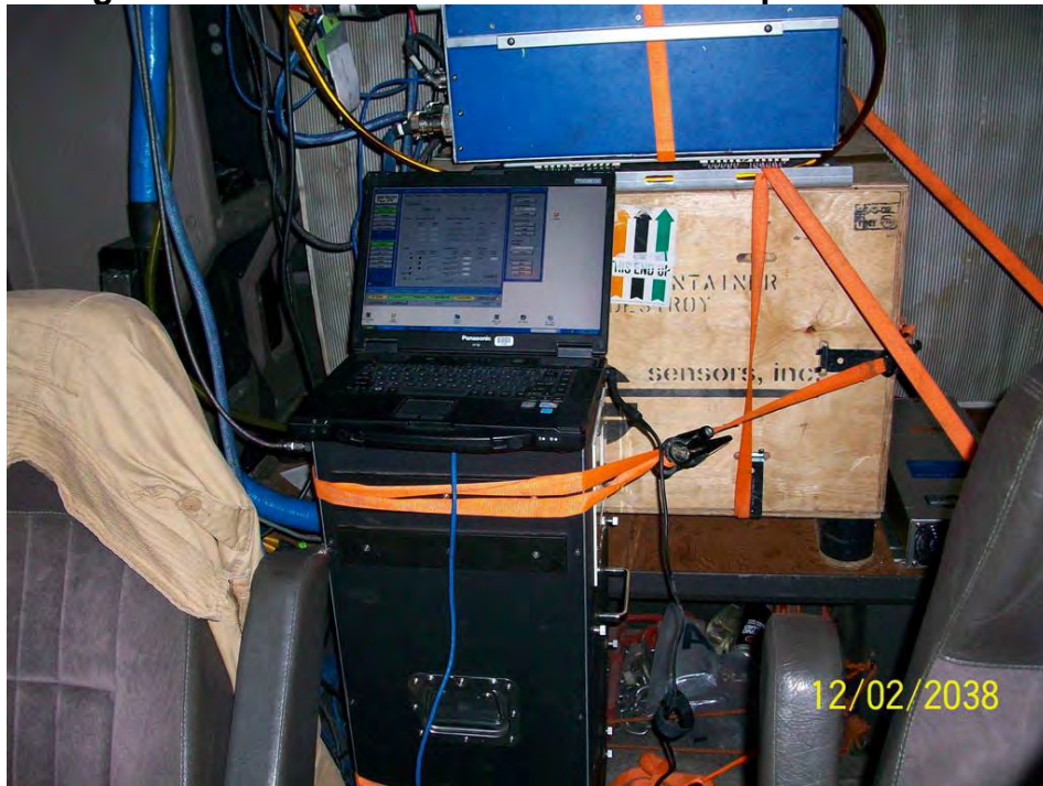
Figure 5.1-13 PEMS On Crate in Sleeper Cab
