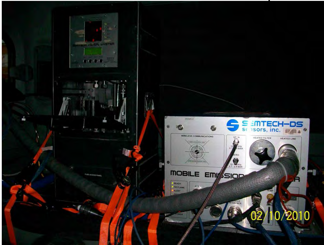
Figure 5.1-23 Access to Filters within the Gravimetric Sampler Assembly
