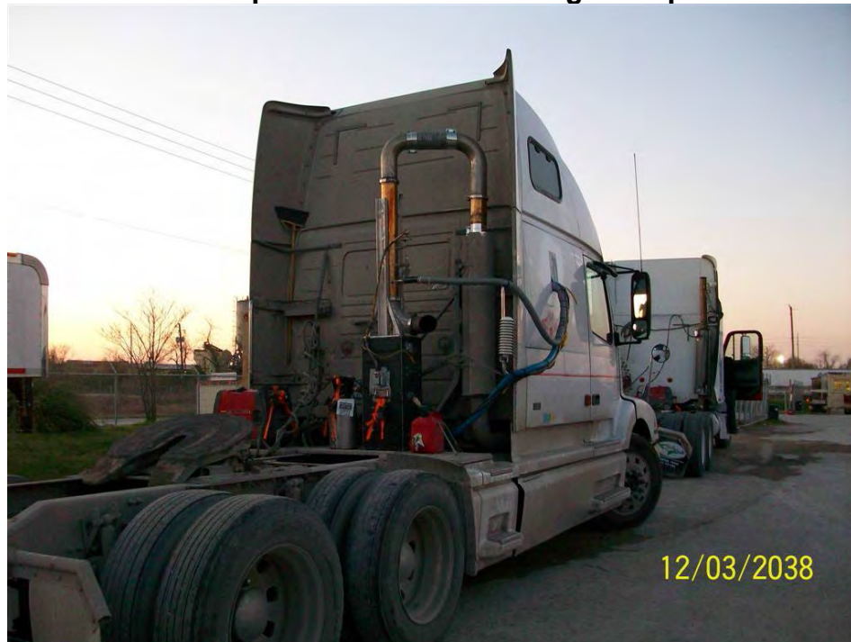
Figure 5.1-15 Sample Lines Routed through Sleeper Cab Vent
