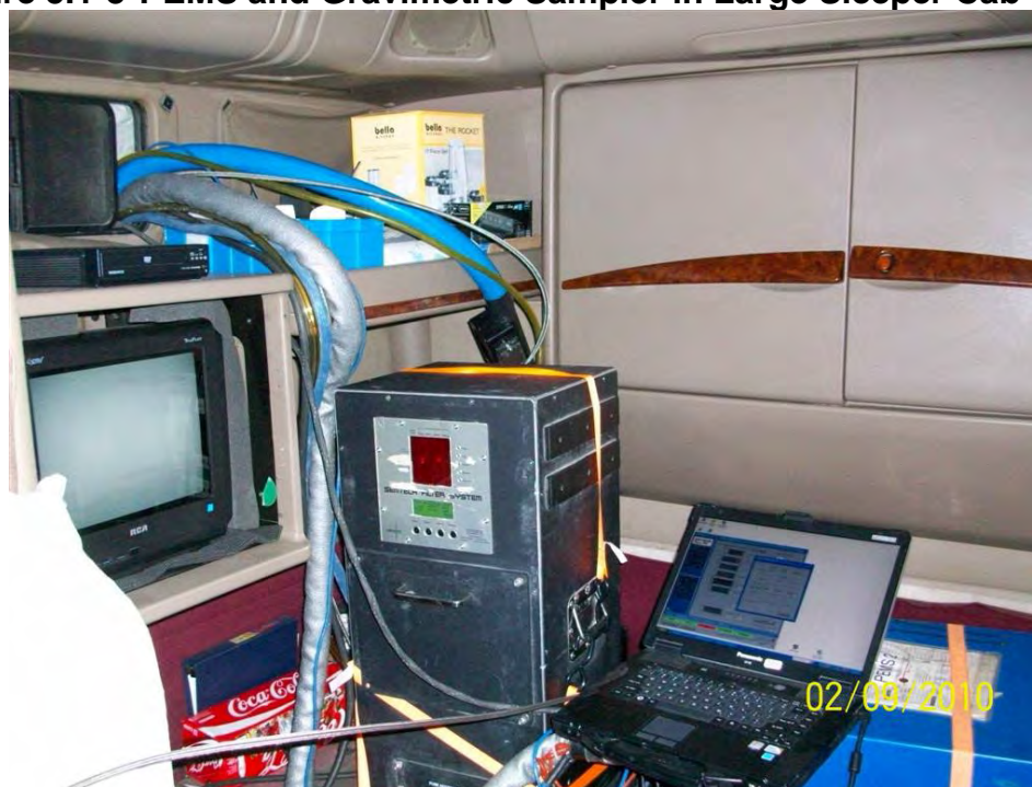
Figure 5.1-8 PEMS and Gravimetric Sampler in Large Sleeper Cab
