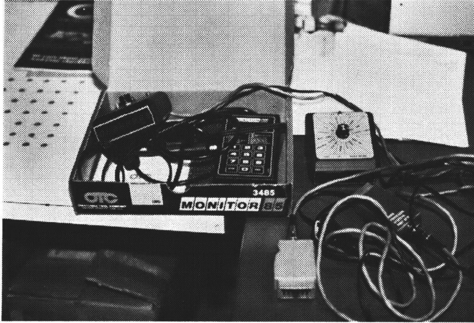
GM computer scanner and volt/ohm tester
