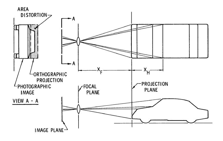
Figure A-2. Schematic of Front View Photographic Projection
