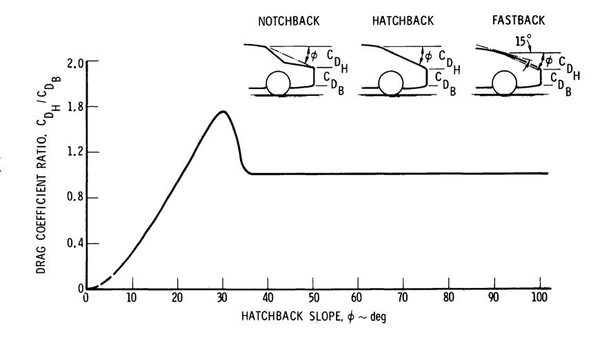
Figure 3-2. Hatchback-Notchback Drag Coefficient Ratio
