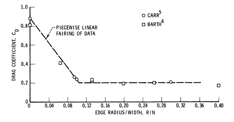
Figure 3-1. Effect of Edge Radius on Drag Coefficient of Rectangular Configurations
