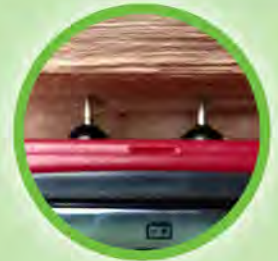
Insert probes into the wood grain
